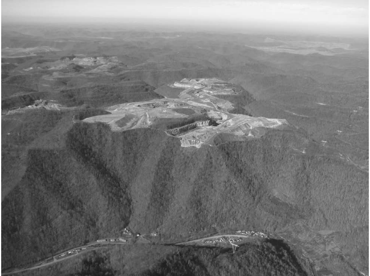
Aerial View of Mountaintop Removal, at Marthatown, West Virginia. The mountaintop removal method of strip mining for coal, practiced in the U.S. since the mid-1980s, is largely controversial for the devastating effects the practice causes to an ecosystem. The states of West Virginia and Kentucky have declared states of emergency several times since 2000, due to the severe environmental pollution caused in their Appalachian regions by this form of mining. FLYOVER COURTESY SOUTHWINGS.ORG/PHOTO COURTESY OF VIVIAN STOCKMAN/WWW.OHVEC.ORG.
