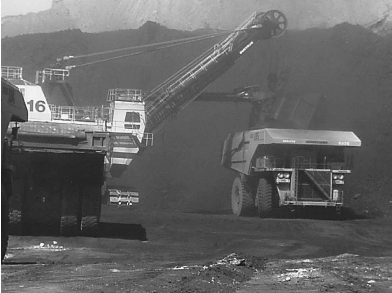
Coal Basin near Wright, Wyoming, 2003. Huge trucks loaded with coal from the Black Thunder Mine can carry from 240 to 360 tons. Unlike other natural resources, coal remains abundant. It has been used to create synthetic gasoline, and can also be converted to electricity. AP IMAGES.
