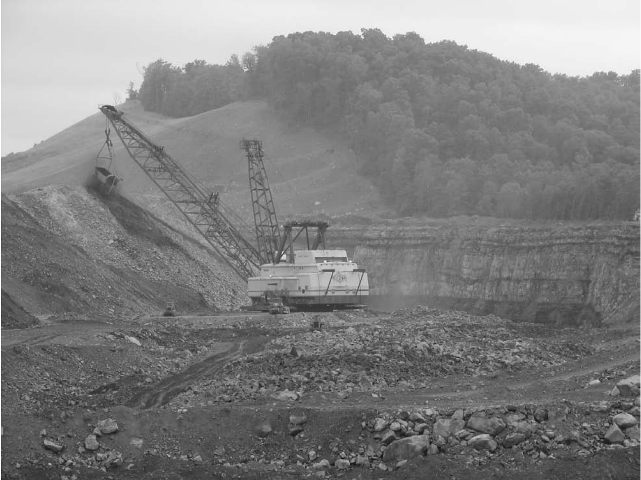
Mining for Coal, West Virginia. Draglines, such as this one at a mine in Boone County, West Virginia, can weigh millions of pounds and are tall enough to loom over a 20-story building. They are used to expose mountaintop coal seams. Mining practices can cause severe environmental damage in terms of physical ground impact and possible contamination of water, air, and soil. PHOTO COURTESY VIVIAN STOCKMAN/ WWW.OHVEC.ORG .
