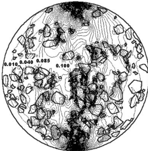
Figure 13. The contour distributions of the maximum principal stress on a non-homogeneous model for the asphalt concrete cross-section from the DIP-FEM analysis (Yue et al. 2003a).
