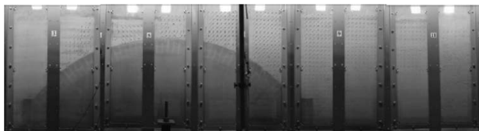
Figure 11. Typical soil displacement around deforming arch barrel.
