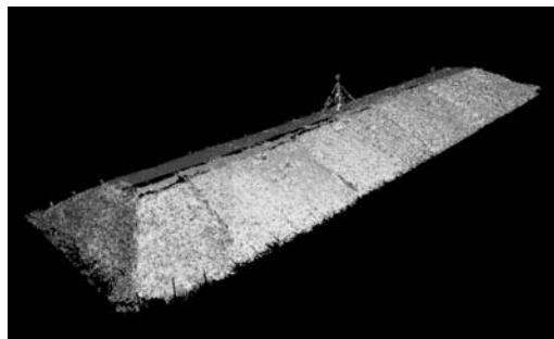
Figure 8. 3-D model from terrestrial laser scan of BIONICS embankment.
