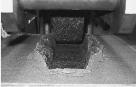
(a) Sand after 8,000 passes at 100kPa (Type 1, 3.4 mm deformation)
