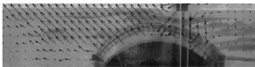
Figure 6. Sample GeoPIV image of crushed limestone test using a coarse mesh.
