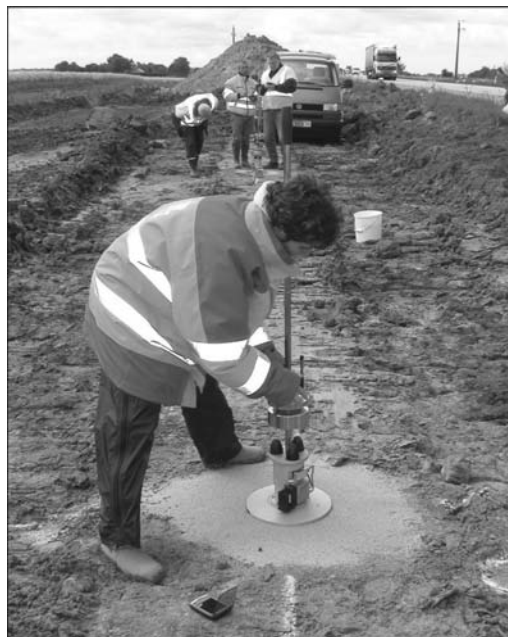
Figure 1. An example of a Light Weight Deflectometer used on a soft subgrade with a E-modulus of less than 10 MPa. (Baltzer et al. 2007).
