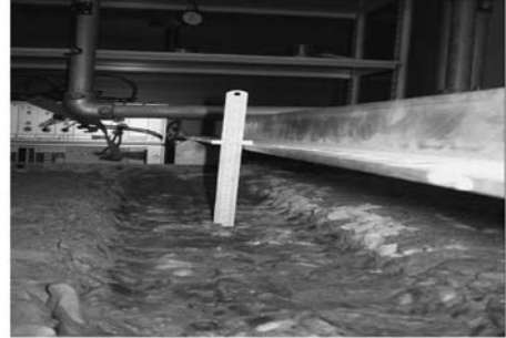
(a) Crushed rock after 10,000 passes at 355kPa (Type 2, 19.5 mm deformation)
