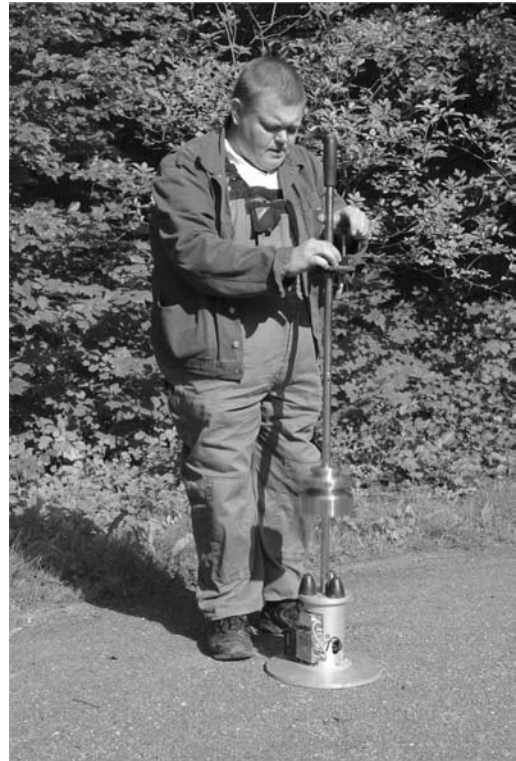
Figure 3. Light Weight Deflectometer testing in Frederiksberg Have, Copenhagen. Photo: P. Kristoffersen, Forest & Landscape Denmark.
