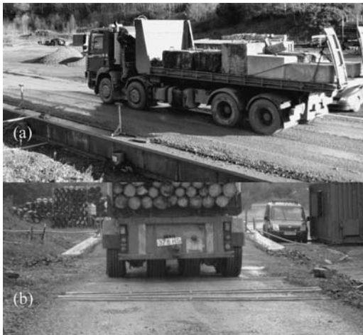
Figure 4. (a) FC “Multi-lift” truck trafficking a Ringour trial (b) “Low ground pressure” vehicle trailer with tyres equally spaced across pavement on stub-axes.
