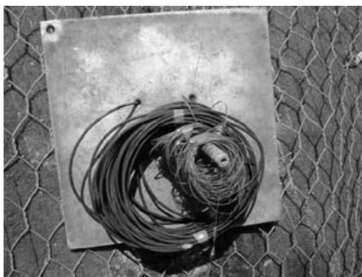
Figure 11. Loose head plate mounted in nail and OFS cables for access to analyser or interconnection.
