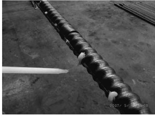
Figure 6. Ribbon fibre attachment in nail.
