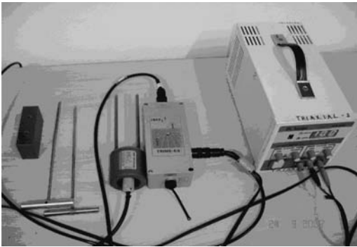
Figure 3. IMKO equipment employed to calibrate TDR probes.
