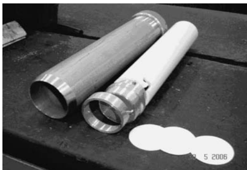
Figure 11. Equipment used for suction measuring in pavement layers.
