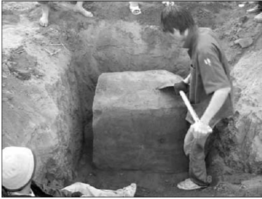
Figure 5. An undisturbed block sample.
