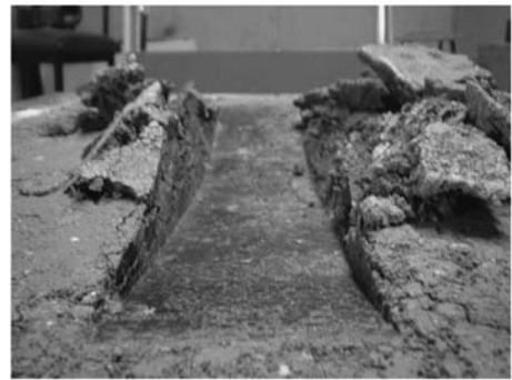
(b) Silty-clay after 650 passes at 301kPa (Type 3, 37.1 mm deformation)
