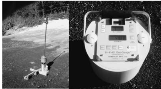
Figure 8. Light portable falling weight deflectometer – LFWD- (left) and stiffness gauge (right) equipments.
