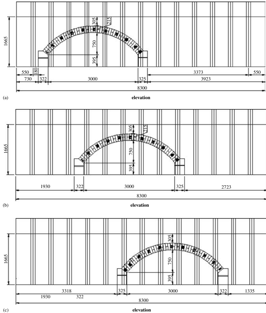
Figure 8. General test arrangement for the full-scale arch tests.
