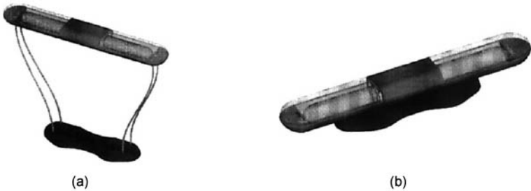
Figure 4 CAD models of the TV backlight: (a) higher position and (b) lower position configurations
