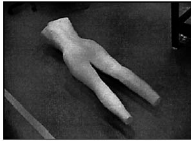
Figure 8. Full-scale custom size mannequin model using Layered-manufacturing
