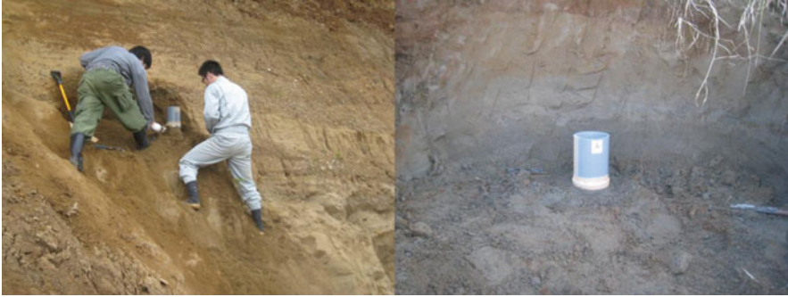
Fig. 3.15 Photographs of block sampling using a PVC tube of 100 mm diameter and 200 height (Left: Pleistocene sand, Right: Holocene sand)
