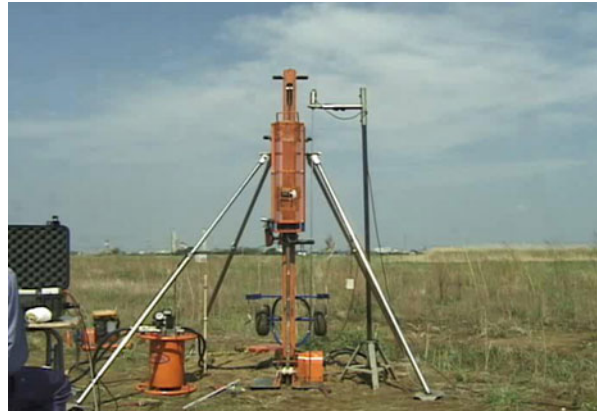
Fig. 6.22 Dynamic CPT with pore pressure recording (Sawada and Towhata 2011)
