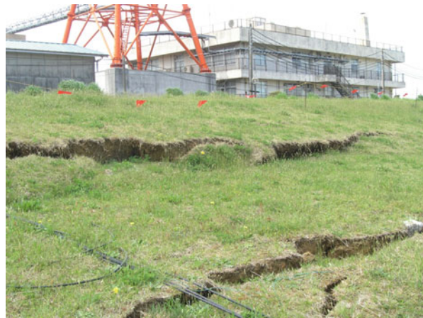
Fig. 6.3 Significant distortion of levee of Tone River in Sawara
