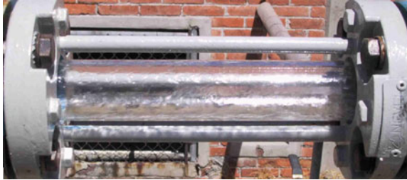
Fig. 2 Flow peephole photograph with annular two-phase flow
