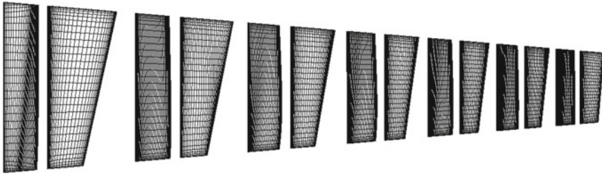
Fig. 2 Meridional view of the compressor mesh
