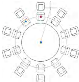
FIGURE 8.8 Stretch Radius in progress.
