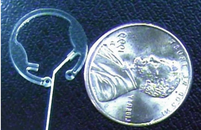
Fig. 13.16 Capsule ring device prototype compared to a penny showing valve assembly with a 27-gauge cannula in the valve access port. Reprinted from Molokhia et al. (2010a, b). Copyright 2010, with permission from Elsevier
