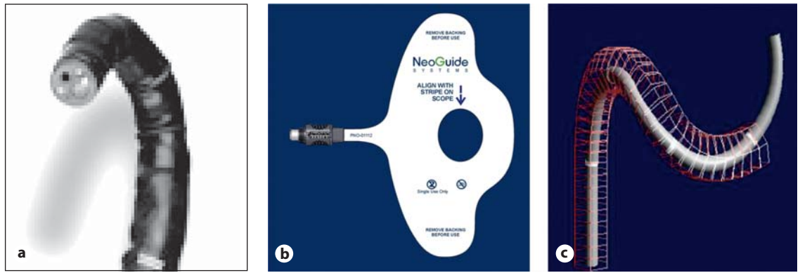
Fig. 1. NeoGuide colonoscope function. A tip position sensor (a) constantly measures tip position, whereas an external position sensor (b) measures tip depth. c A 3D colon map is generated as the scope is advanced.
