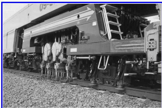
Figure 14.2 A closer view of the tamping machine showing tamping tines and lifting rollers.
