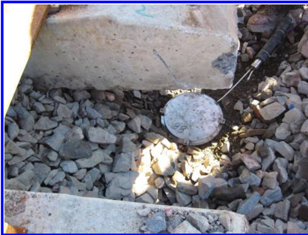
Figure C6 Installation of pressure cell at the ballast-capping interface at Singleton.
