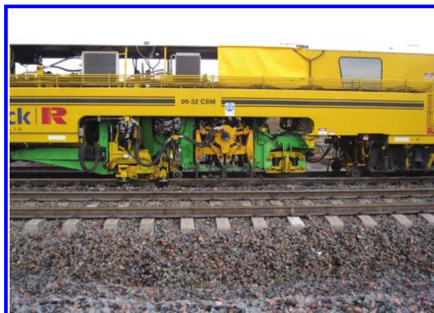
Figure C3 Automated tamping equipment used at fully instrumented track at Singleton town near Newcastle, New South Wales.
