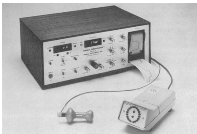
Figure 3. The EMG transducer with associated detector and recording instrumentation for monitoring the contractile activity of the pubococcygens muscle. (Courtesy of Farrall Instruments, Ins., Grand Island, NE.)
