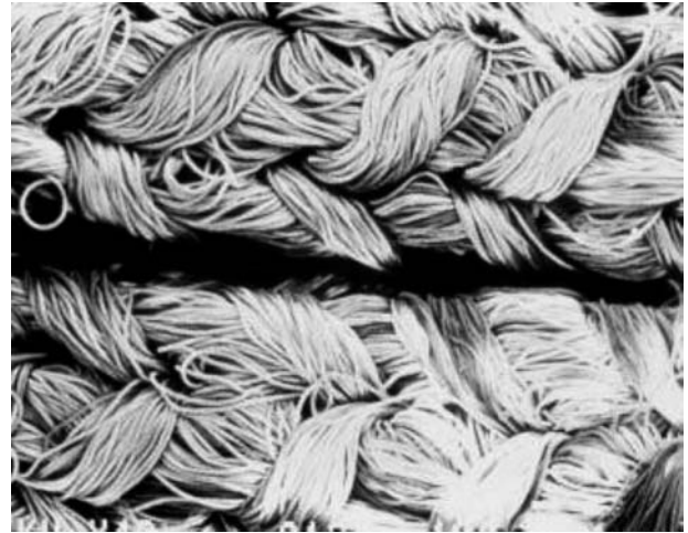
Figure 3. Scanning electron micrograph (SEM) of knitted Dacron vascular graft prostheses. The knitted prostheses are of lower porosity than the woven Dacron prostheses and must be sealed by preclotting prior to implantation. SEM, Original Magnification 1000 \times .
