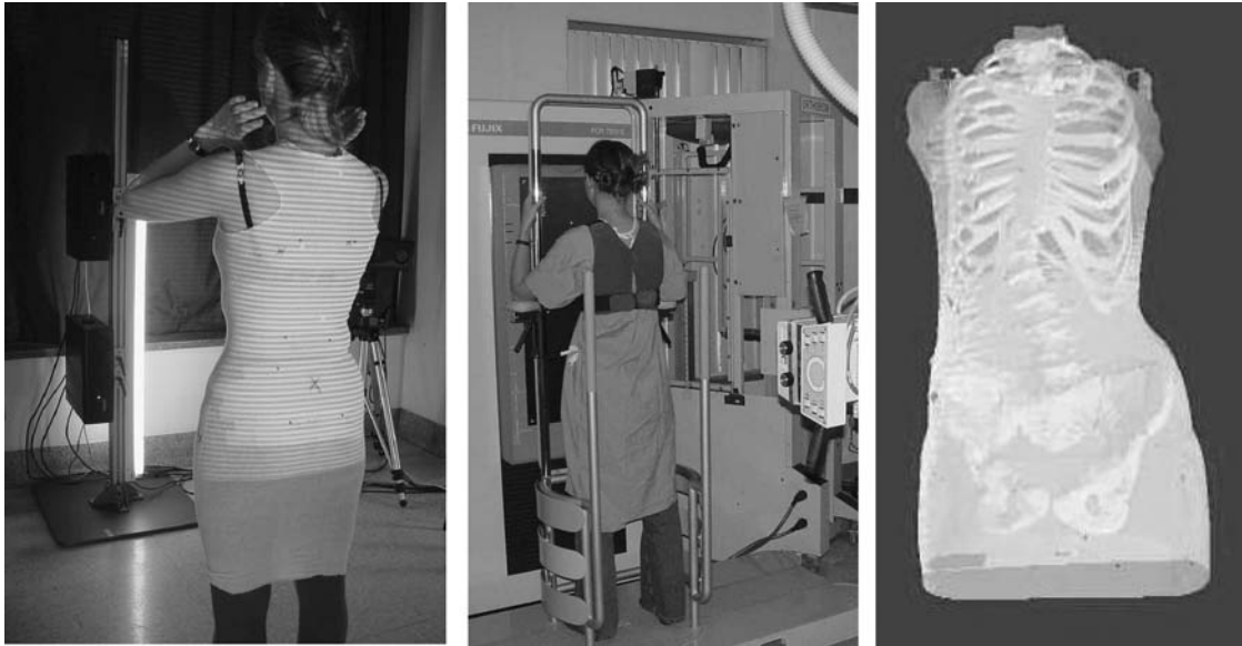
Figure 9. Range sensing topographic scanner (two of the six cameras that surrounds the subject are shown on left panel) and biplanar X-ray system (middle panel) for concurrent surface and spine imaging, showing typical superimposed 3D torso spine model (right panel).
