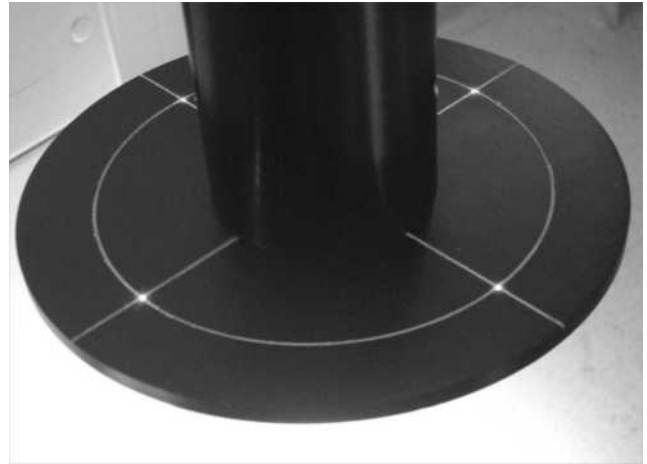
Figure 11. Example of the optical alignment used on the Mevatron ME linear accelerator. This test jig is used before each procedure to check the alignment of the lasers. Alignment is correct when the dots and lines (not easily seen here, but overlapping the radial lines) cross on the circle.
