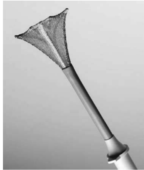
Figure 26. NovaSure catheter used for endometrial ablation. This catheter has an electrode consisting of multiple electrically isolated meshes, with rf energy applied bipolar between different meshes. Image provided courtesy of Cytac Corporation and affiliates.
