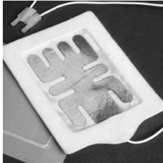
Figure 38. An electrostimulation electrode with cut-out metal plate in an effort to increase peripheral edge. The green sponge impregnated with gel has largely been removed to facilitate inspection of the underlying plate.
