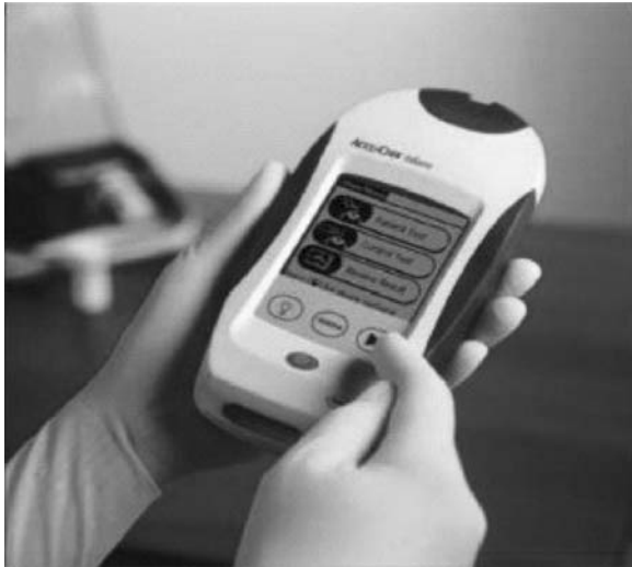
Figure 4. The Roche Accu-Check is a small, easy to use blood glucose meter; it is widely used by our Point of Care Testing program. Test results are downloaded to the Laboratory Information System.
