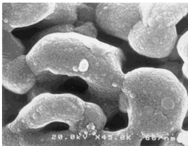
Figure 21. The SEM photograph showing the surface morphology of the SHA900 immersed in SBF for 9 weeks.
