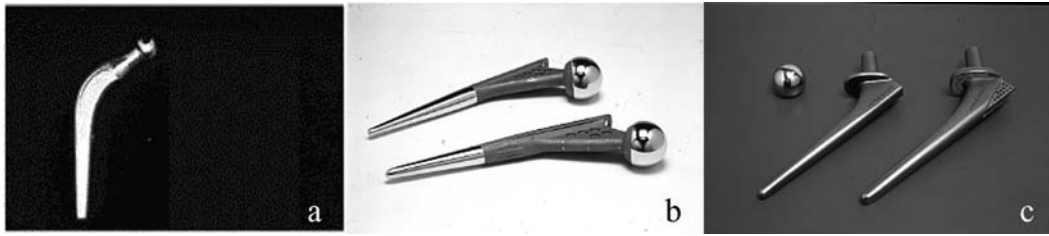
Figure 3. Photographs of stainless steel (a), cobalt–chromium (b), and titanium alloy (Ti6Al4V) (c) hip implants. (All three photographs are used with permission from the Department of Materials at Queen Mary University of London.)
