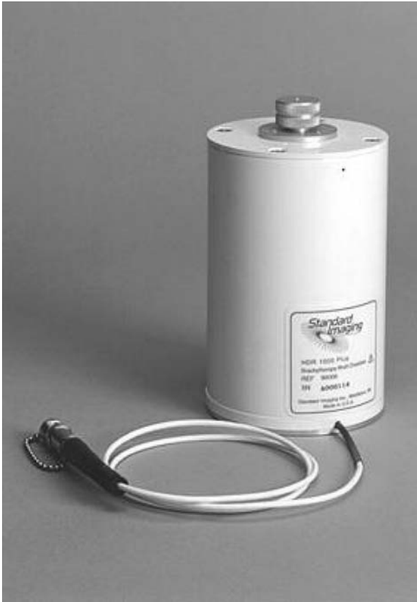
Figure 7. A re-entrant well-type ionization chamber used for calibration of the HDR brachytherapy sources.
