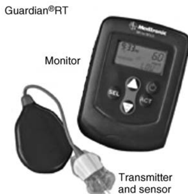
Figure 3. Ambulatory glucose monitoring with guardian real time system (Medtronic MiniMed).
