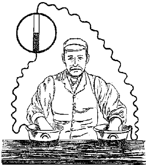
Figure 14. Human subject connected to capillary electrometer via large area bucket electrodes (81).
