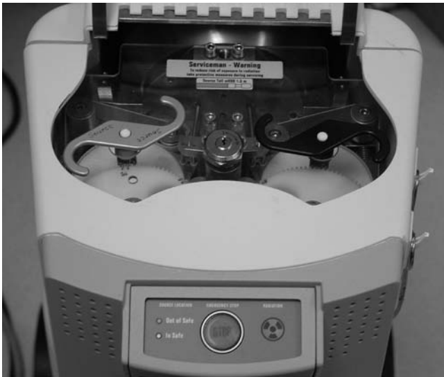
Figure 14. A view of the access panel of the MicroSelectron treatment unit. The center button is an emergency stop button on the treatment unit. Also showing are the manual retraction of the radioactive source cable (left) and the check cable (right).
