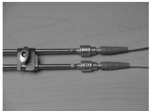
Figure 10. View of the transfer tubes connected to a gynecological applicator. Ball bearings beneath the gray polymer coating allow verification of the proper connection of the transfer tubes to the applicator. The number 1 and 2 represents that these transfer tubes must connect the channel 1 and 2 of the indexer ring and the similarly numbered parts of the applicator.
