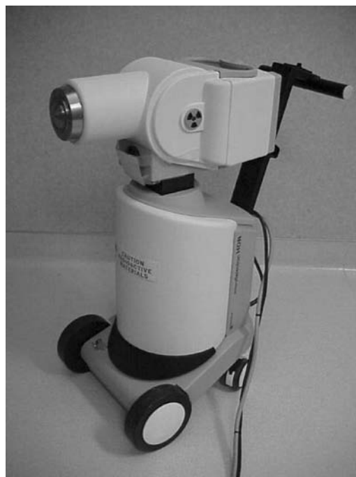
Figure 1. The Nucletron MicroSelectron V2 HDR RAL. The RAL wheels allow it to be conveniently positioned near the patient. The treatment head is mounted on a telescopic base that allows the head to be raised or lowered to the required height for treatment without moving the patient.
