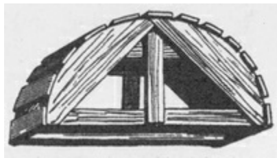
Centering of a round-headed arch.
