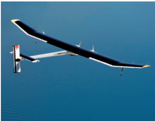
A 1.34 What electrical self-sufficiency means is demonstrated figuratively by the ambitious project of circumnavigating the globe in five consecutive phases with an exclusively solar-powered electric glider [61]. The aircraft’s wings span 63 m and are completely covered with high-performance solar cells. Batteries with a capacity of just under 100 kWh serve for buffering. Weighing 400 kg, the batteries comprise a fourth of the aircraft’s total weight.
