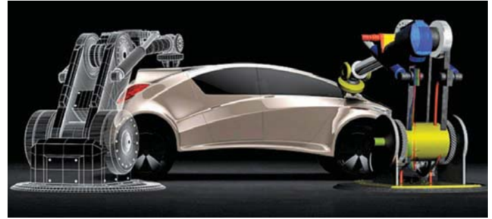
FIGURE 3.27 A representation of CADD data used within a CIM process of automobile assembly and inspection. Courtesy Autodesk, Inc.
