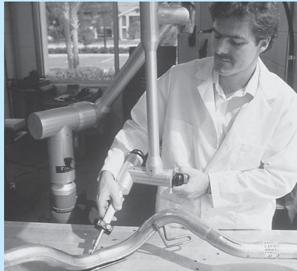
FIGURE 21.64 The dimensions of an existing pipe can be input to the CADD software using a 3-D digitizer.
