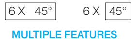
FIGURE 13.15 The basic dimension symbol is a thin line box placed around the dimension value. When dimensioning multiple features, the number of places or times can be applied inside or outside the basic dimension symbol.
