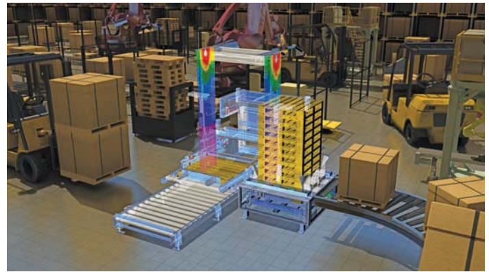
FIGURE 3.16 Using digital prototyping to model, analyze, simulate, and visualize the operation of packaging equipment within a virtual packaging facility. Courtesy Autodesk, Inc.
