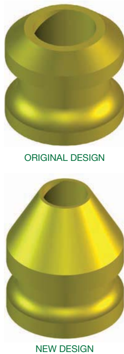
FIGURE 3.54 Significantly modifying a design by quickly editing a few model parameters.
