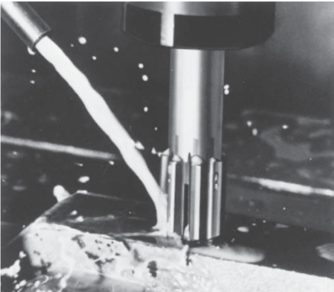
FIGURE 4.22 End milling operation. Courtesy Greenfield Industries
