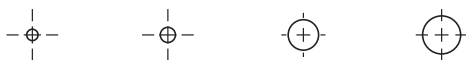
FIGURE 6.8 Centerlines for small circles. These drawings have been reduced to fit in the space available. Keep in mind that the center dashes should be .125 in. (3 mm) long. © Cengage Learning 2012
