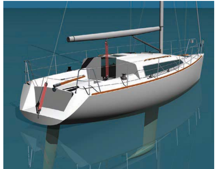
FIGURE 3.41 A sailboat modeled using AeroHydro, Inc., MultiSurf surface modeling software. Courtesy Reinhard Siegel
