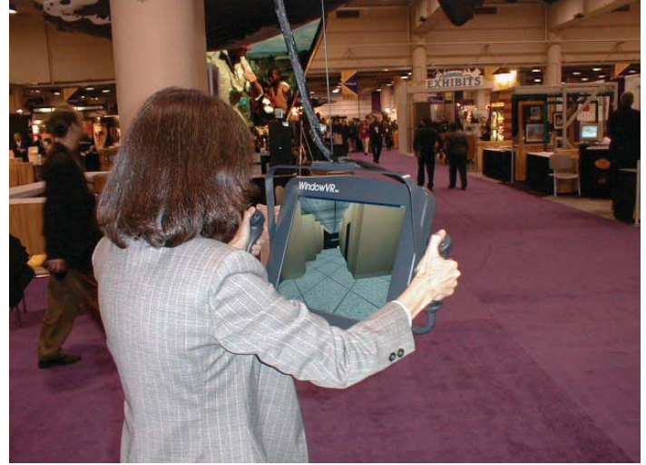
FIGURE 3.29 This unit is designed to allow natural interaction with the virtual environment. Museum and showroom visitors can walk up, grab the handles, and instantly begin interacting. Observers can follow the action by moving beside the primary user. Courtesy Virtual Research Systems, Inc.
