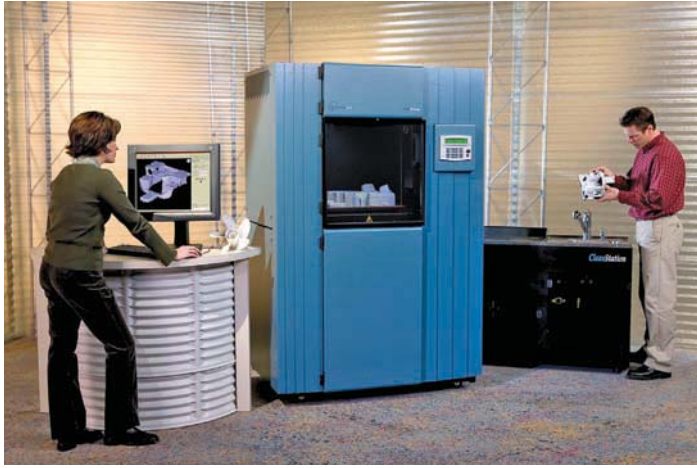
FIGURE 3.17 Following a tool path defined by the CAD file, the fused deposition modeling (FDM) system builds the model layer by layer. The build head extrudes molten thermoplastic in layers of .005–.010 in. with tolerances of up to .003 in.
