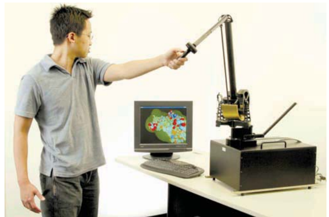
FIGURE 3.34 Phantom haptic device provides haptic feedback to the user.
