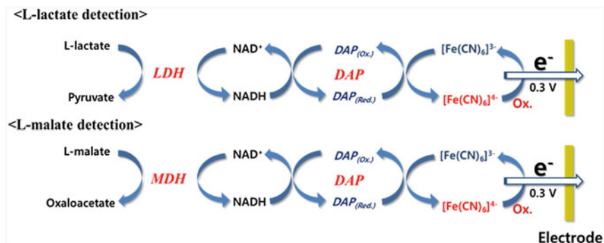
Fig. 9 Schematic illustration of a cascadic bienzyme reaction employed in an electrochemical L-lactate/L-malate biosensor suggested by Katrlík et al. [73]. DAP , Diaphorase; LDH , Lactate dehydrogenase; MDH , Malate dehydrogenase; NAD , Nicotinamide adenine dinucleotide (oxidized); NADH , Nicotinamide adenine dinucleotide (reduced)
