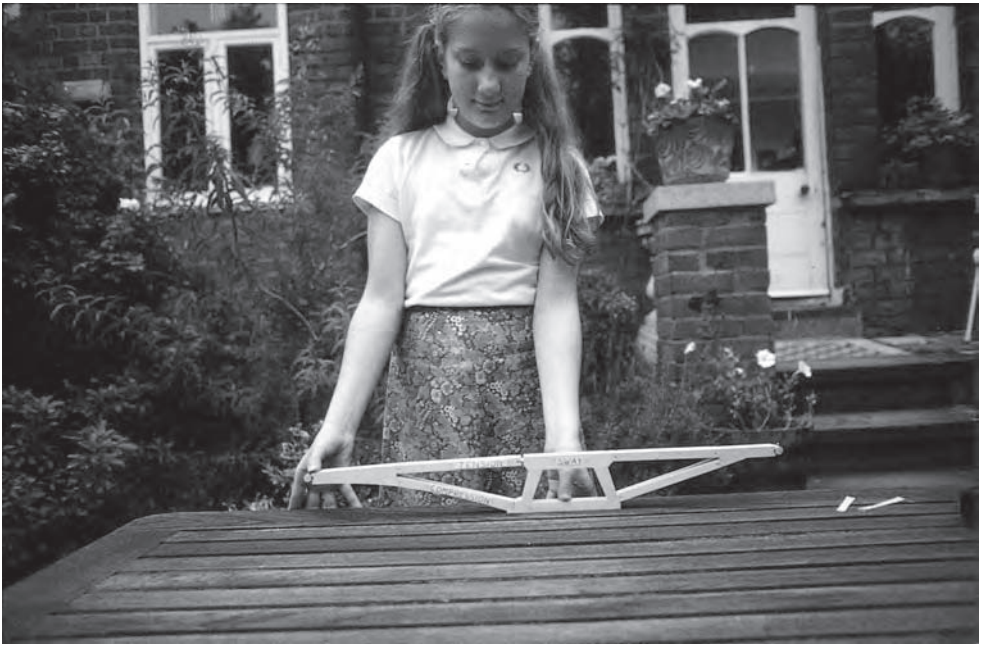
Figure 1.12d New Runnymede Bridge: load testing the bridge model (Photo: Robert Benaim)
