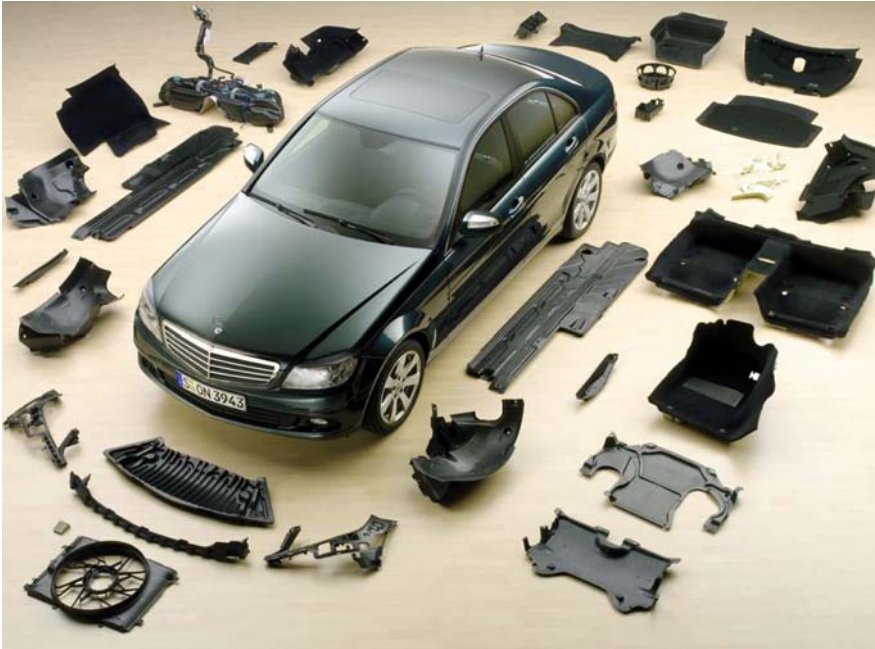
Figure 3.24 A Mercedes Benz can be quickly disassembled for end-of-vehicle life recycling. (Photograph courtesy of Mercedes Benz GmbH, Stuttgart, Germany)
