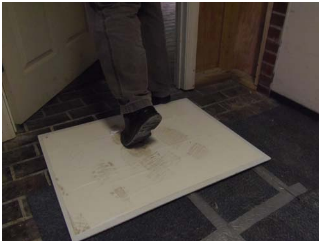
Figure 13.4 Sticky mats and walk-off mats are entrance control measures to help reduce contaminants entering into a clean area. (Photograph courtesy of D. Stephany)
