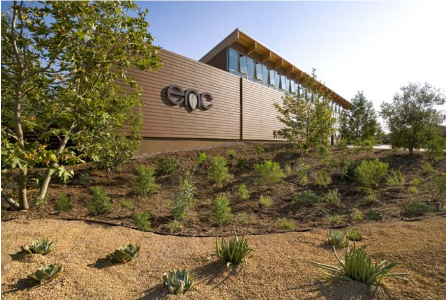
Figure 10.18 The Environmental Nature Center in Newport Beach, California, is landscaped with a water-saving design and a diverse selection of native species. Selection of native plant material in the landscape requires little or no irrigation and helps to maintain not only the ecosystem but also the indigenous character of the site. (LPA, Inc./ Costea Photography, Inc.).
