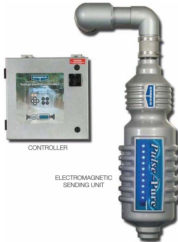
Figure 6.6 Pulsed electromagnetic technology is used to treat the cooling tower water. This technology helps reduce scaling, biological growth, and corrosion, all without the use of chemicals. It also helps reduce water consumption and makes water easier to treat compared to chemically treated systems.
