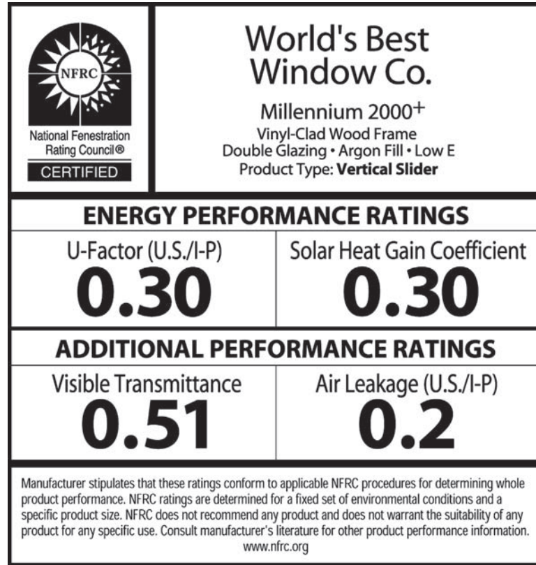
Figure 9.15 The NFRC adopted a new energy performance label in 2005. It lists the manufacturer, describes the product, provides a source for additional information, and includes ratings for one or more energy performance characteristics. (Source: National Fenestration Rating Council)
