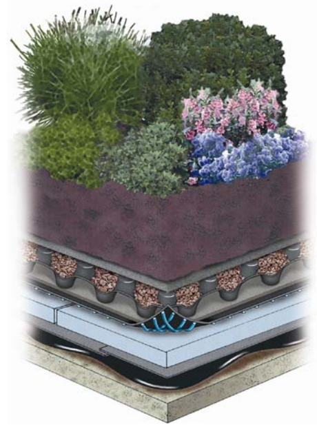
Figure 8.5 Cross section of an extensive eco-roof system that provides structure and drainage. (Image courtesy of American Hydrotech, Inc.)
