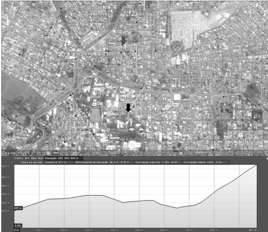
Fig. 3 Longitudinal profile, obtained with Google Earth, of a selected stretch of the proposed network of cycling routes
