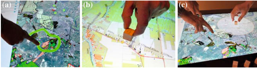
Fig. 2 Details of the user interaction: a sketching with a finger, b using a physical object to display a dynamic scale, c placing and rotating a small wooden block to define the center and size of a buffer/distance
