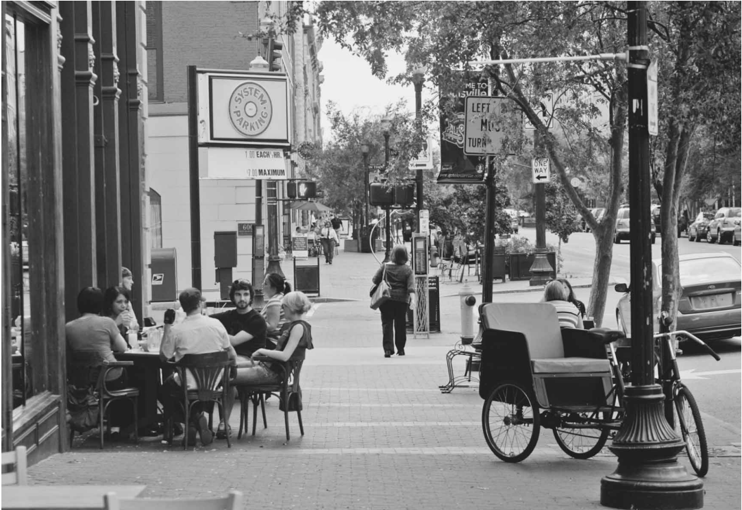
FIGURE 26. WEST MAIN STREET, LOUISVILLE, KENTUCKY (2008). AECOM (FORMERLY EDAW), ALEXANDRIA, VIRGINIA. (Photograph by David Lloyd, © AECOM.) Black brick pavers with a high iron content were used to correspond to the adjacent historic cast-iron facades and ornament.
