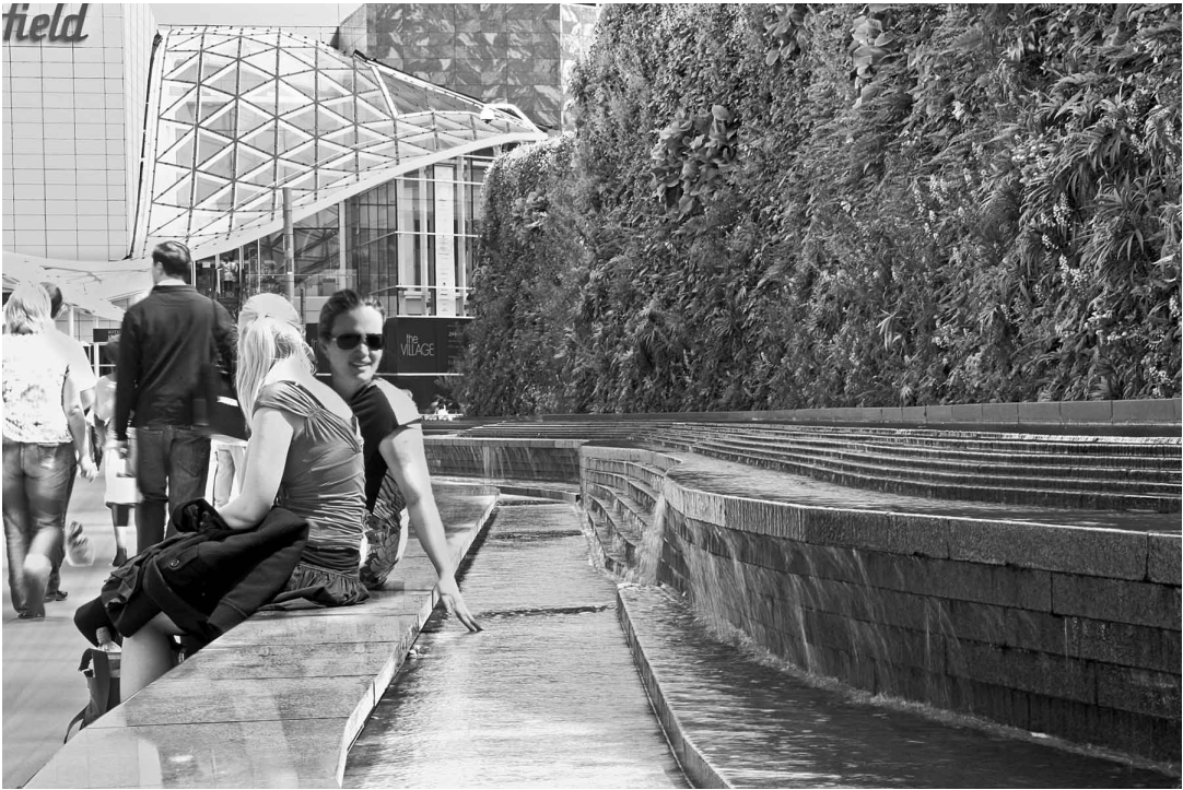
FIGURE 51. WESTFIELD SHOPPING CENTRE, LONDON (2008). AECOM, U.S. WEST. (Photograph by James Haig Streeter, © AECOM.) Rhino 3-D modeling software was used to draw the design for the granite fountain and seat wall with curving forms. Computer Numerical Control (CNC) machining technology was used to fabricate the stone directly from the software models.
