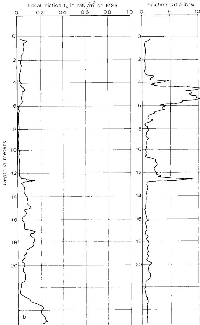
Fig. 11.12b. Local friction cone resistance and friction ratio.
