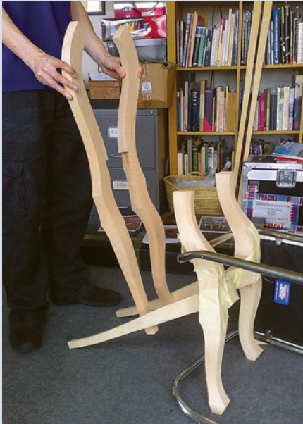
The principal components are loosely assembled for initial appraisal.
