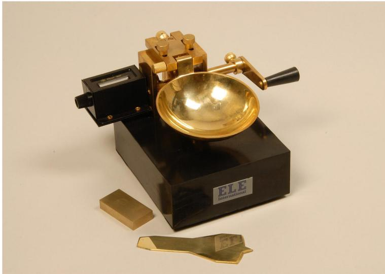
**Figure 2.1** ELE Liquid Limit device with accessories EL24-0410. Reproduced by permission of ELE international.
