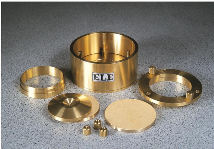
**Figure 7.2** Consolidation Cell Components. Reproduced by permission of ELE International.
