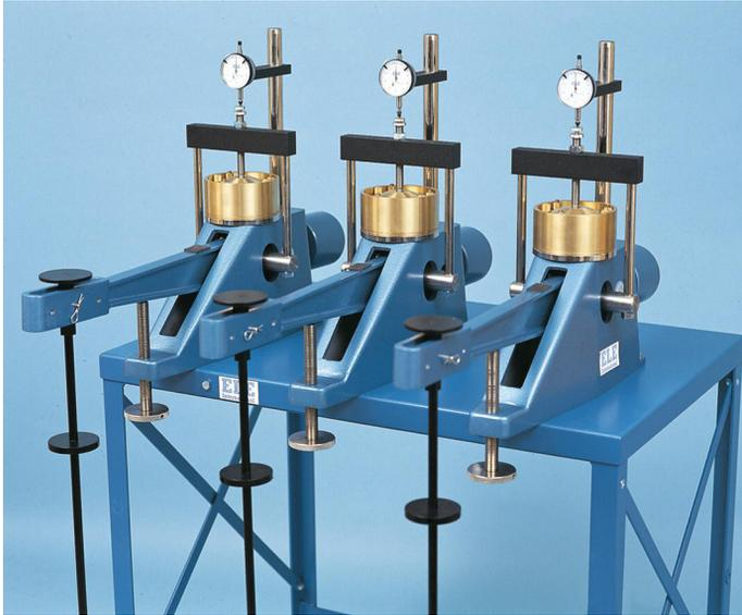
**Figure 7.1** EL25-0402 Consolidation Frames. Reproduced by permission of ELE International.
