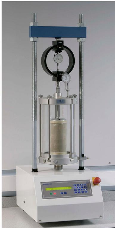
**Figure 6.36** EL25-3700 series MultiPlex50 for quick undrained triaxial test. Reproduced by Permission of ELE International.
