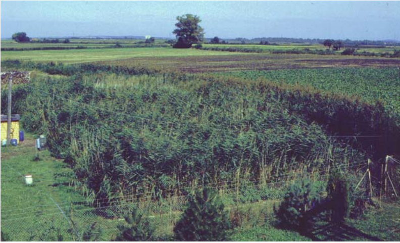
Figure 7-1. Experimental HF constructed wetland Mannersdorf, Austria. Photo by Raimund Haberl, with permission.
