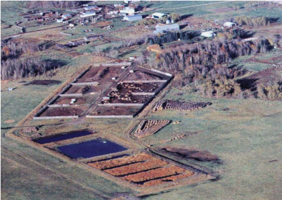
Figure 4-25. A FWS livestock constructed wetland for high strength runoff at the 300-head cow-calf feedlot in Riverton, Manitoba, Canada. The system consists of three units: the settling pond, the holding pond, and 0.5 ha treatment wetland. Photo provided by Prairie Farm Rehabilitation Administration, Winnipeg, BC, Canada.
