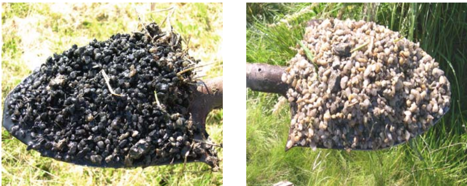
Figure 5-22. HF system at Břehov, Czech Republic. Gravel substrate taken 2 meters (left) and 25 meters (right) from the inflow. Note substantial biomat formation in the inlet sample.
