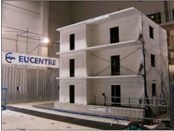
Fig. 44.1 Specimen on the shake table of Eucentre
