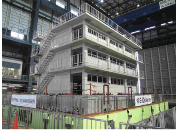
Fig. 11.2 Overview of bare RC specimen in the container with backfill soil on the shake table
