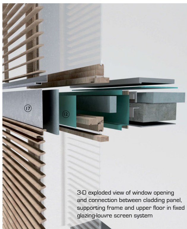
3-D view of timber clad facade incorporating both louvred and board panel types
