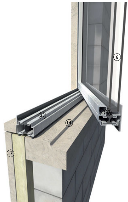
3-D view of double glazed steel framed window set in cavity wall construction
