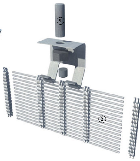
3-D exploded view of hooked metal mesh fixing
