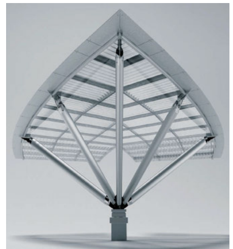
3-D bottom view of louvred canopy
