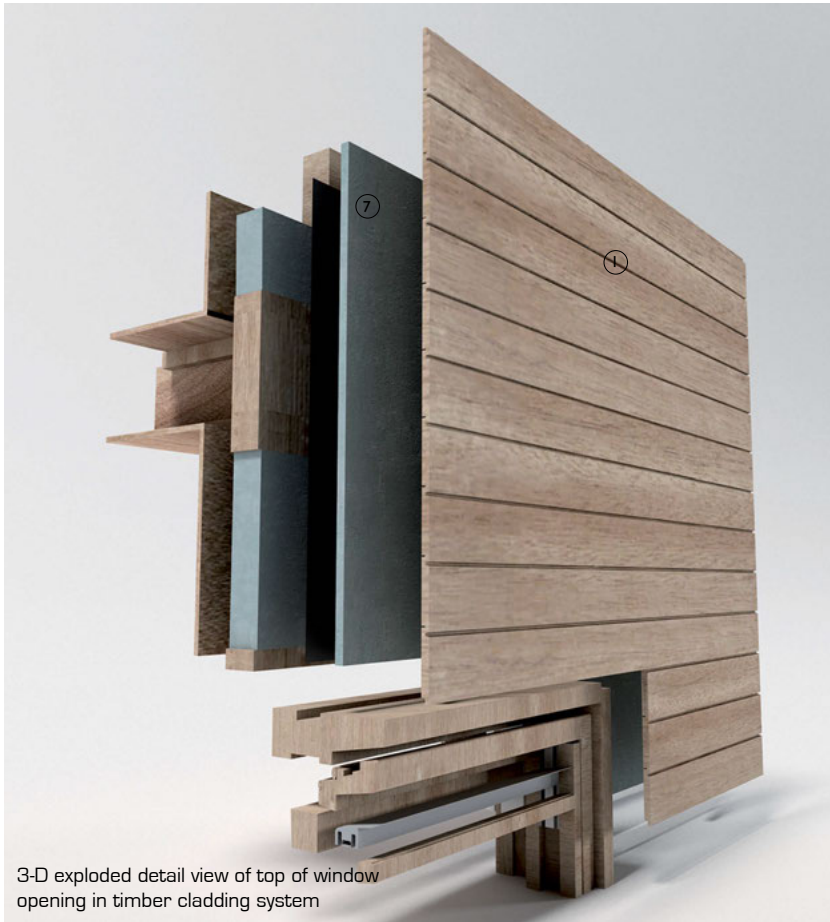
3-D view of window opening in timber cladding system
