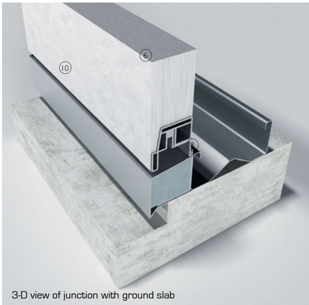
3-D view of concealed gutter detail
