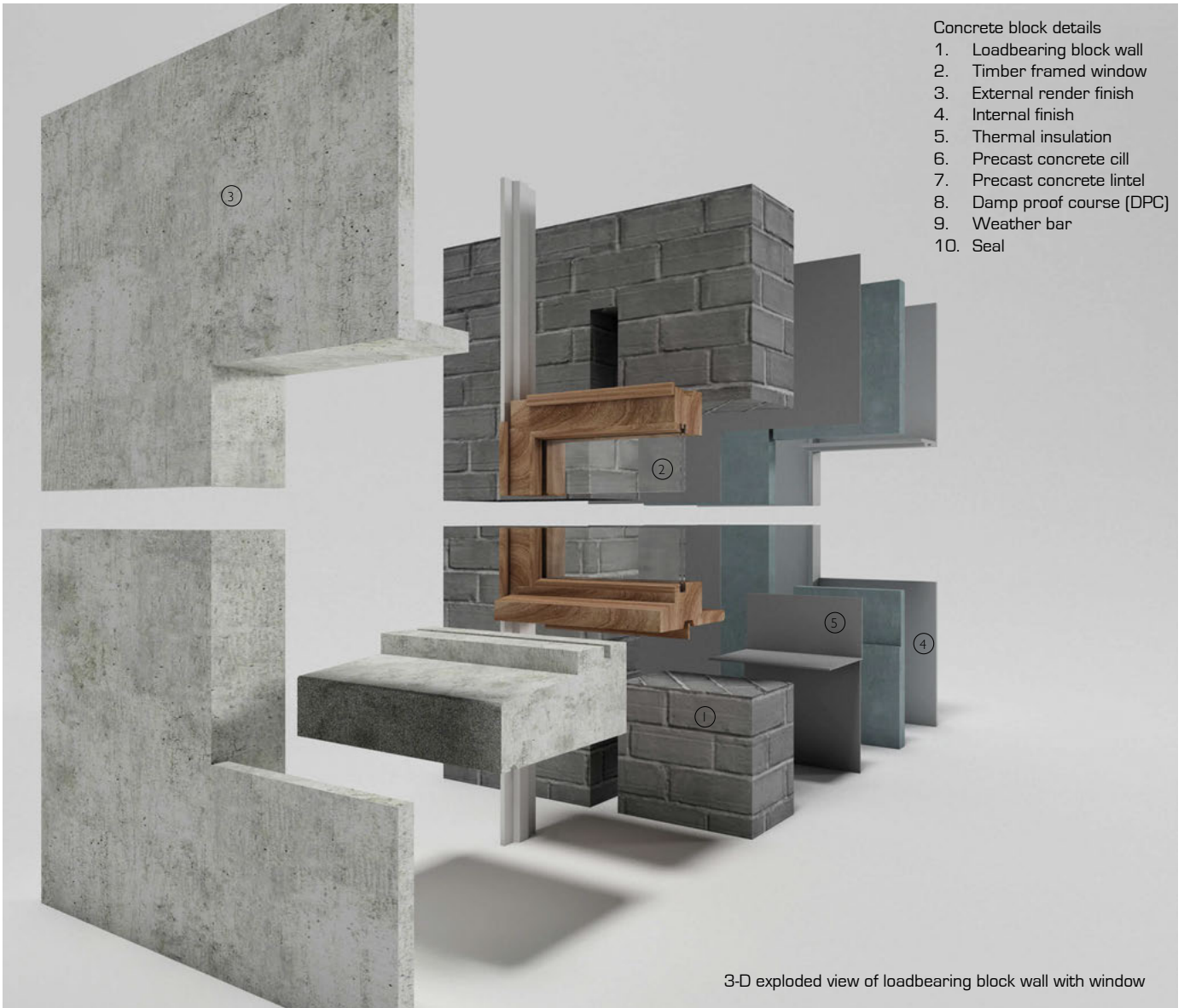
3-D exploded view of loadbearing block wall construction
