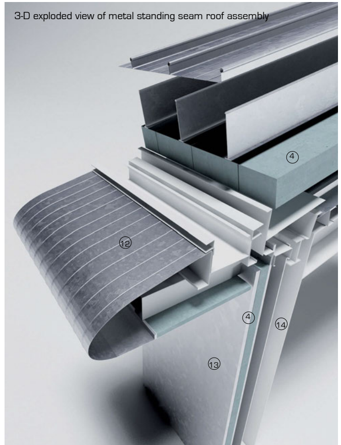
3-D view of metal standing seam roof parapet and gutter detail
