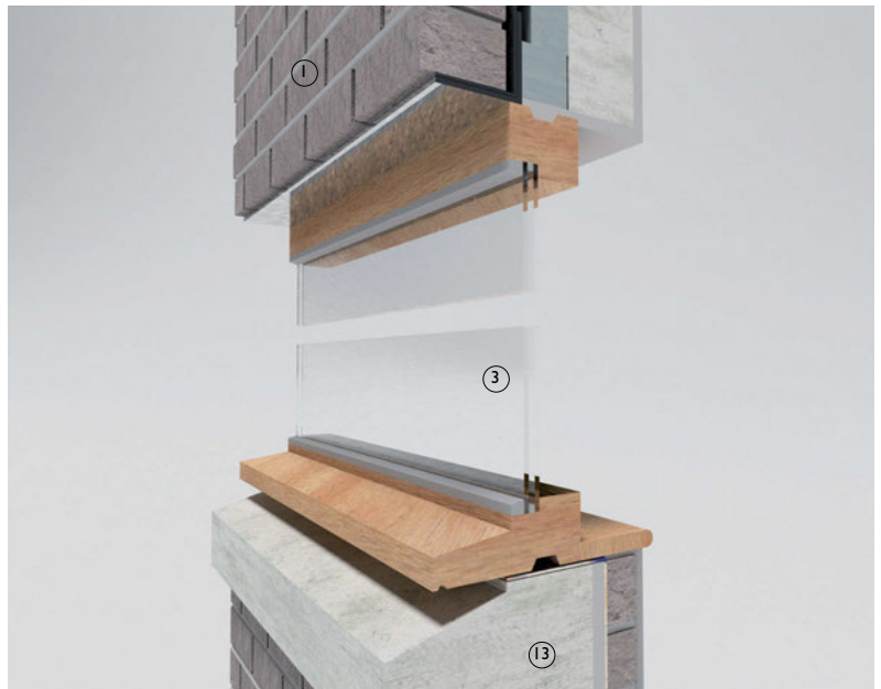
Vertical section 1:10. Junction at ground floor level
