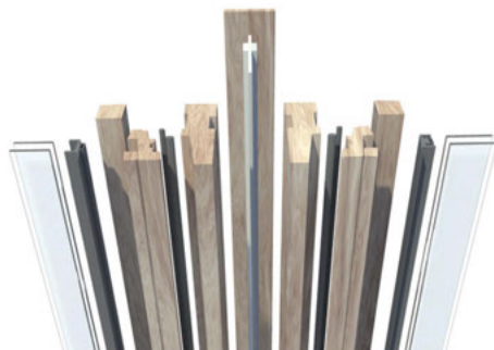
3-D exploded views of various timber window construction configurations
