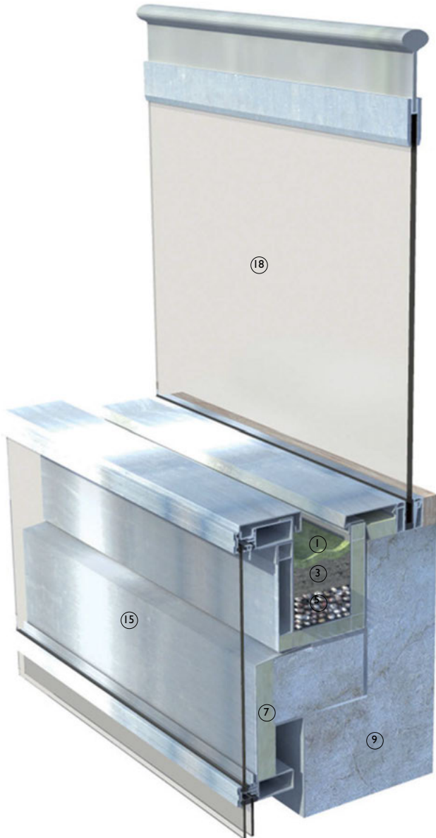
3-D view showing small balcony planter arrangement
