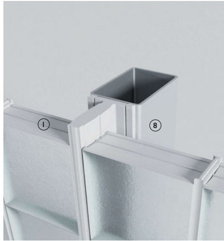
3-D view of connection between glass blocks supported by steel box frame
