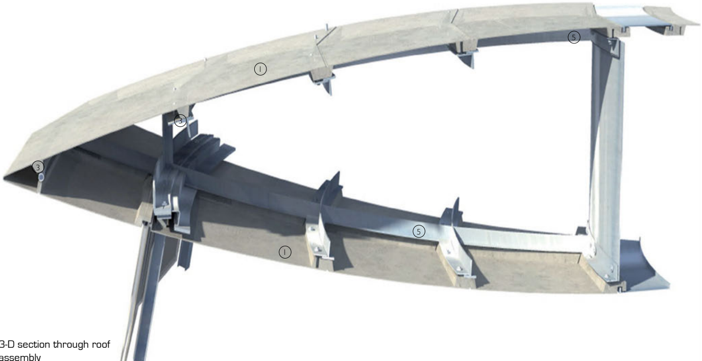
Horizontal and vertical sections 1:50. GRP shell roof
