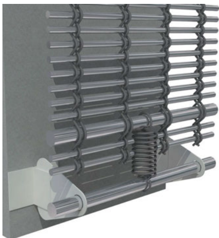
3-D view of metal mesh fixed to steel rod with tensioning spring
