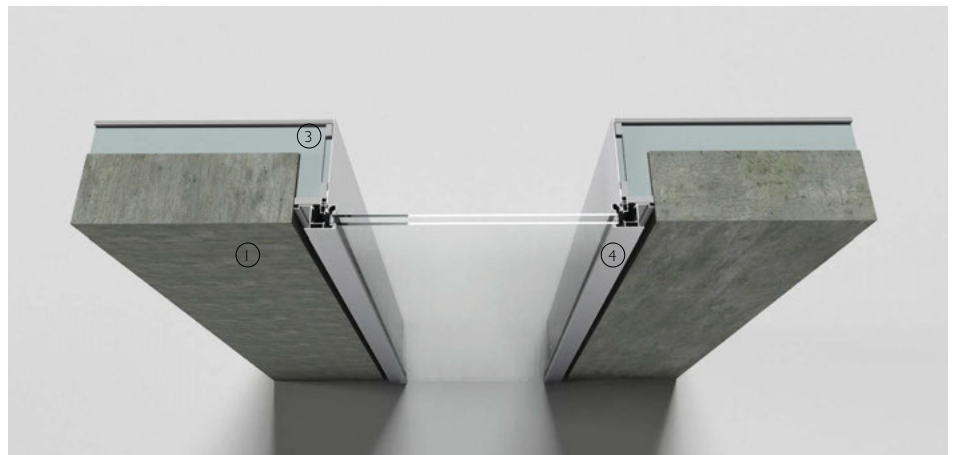
3-D view of in-situ loadbearing concrete wall junction with window flush to exterior face
