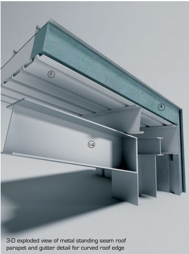
3-D exploded view of metal standing seam roof assembly
