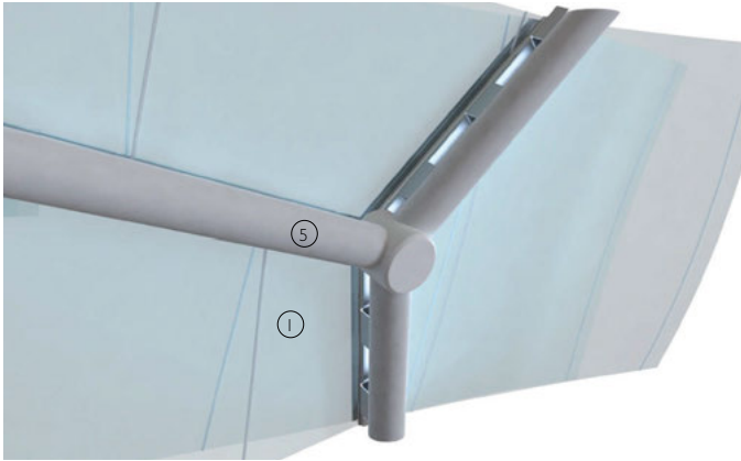
3-D detail of junction between ETFE cushions
