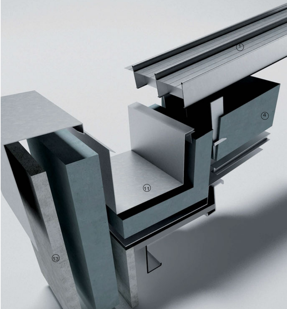
3-D exploded view of metal standing seam roof parapet and gutter detail
