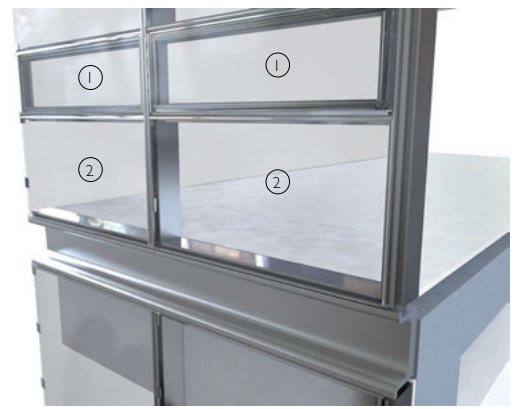
3-D view of aluminium window as part of a unitised glazing system
