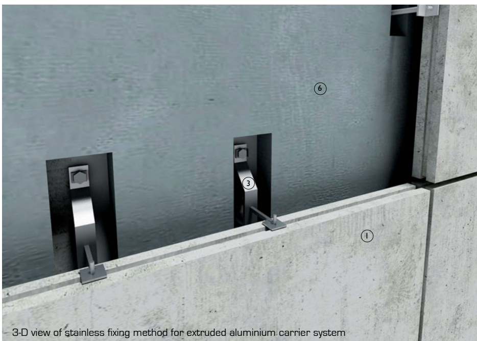
Vertical section and elevation 1:25. Typical stone carrier system made from extruded aluminium. Stone joints with both straight and staggered joints to show flexibility of carrier systems
