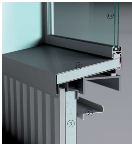
3-D views of head and sill details of recessed aluminium window in profiled metal facade
