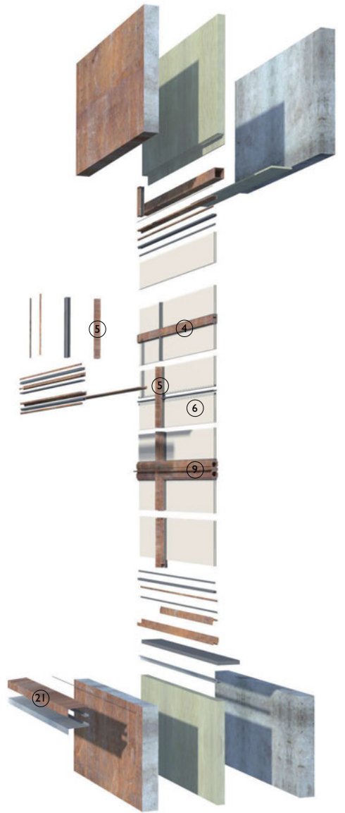
3-D exploded view of rolled steel facade
