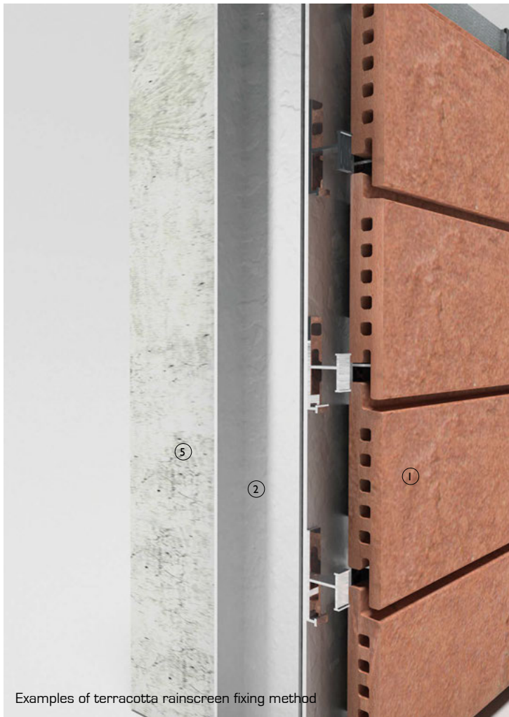
Isometric view of vertically set wall assembly
