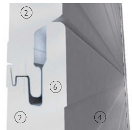
3-D views of profiled composite panel fixed to steel and of horizontal interlocking joint between profiled composite metal panels.
