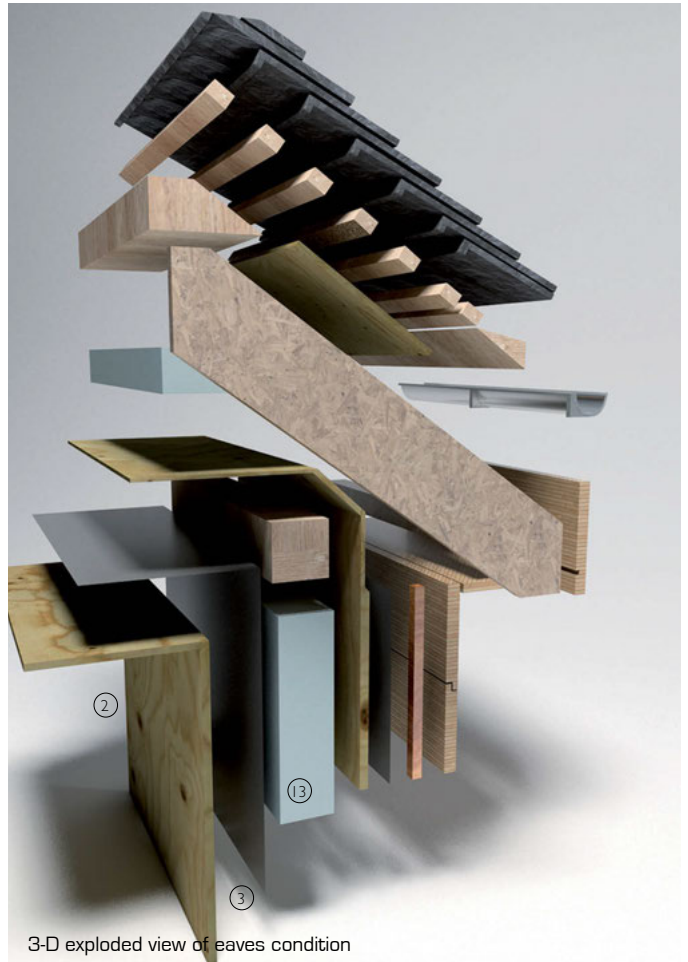
3-D exploded view of eaves condition
