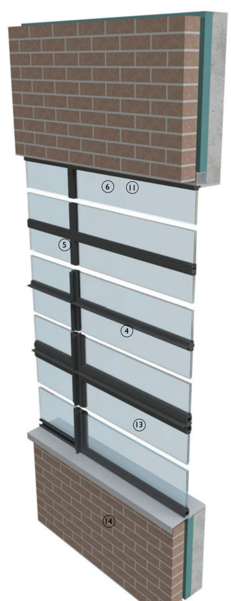
3-D view of rolled steel window details
