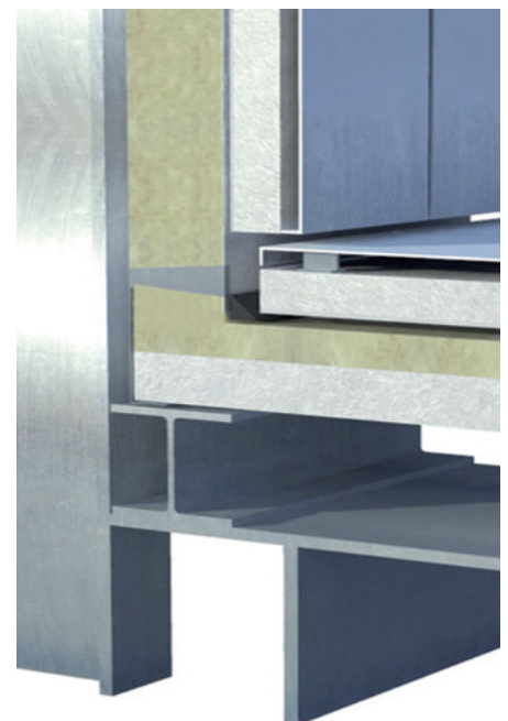
3-D view corner condition of composite panel roof system beneath metal rainscreen
