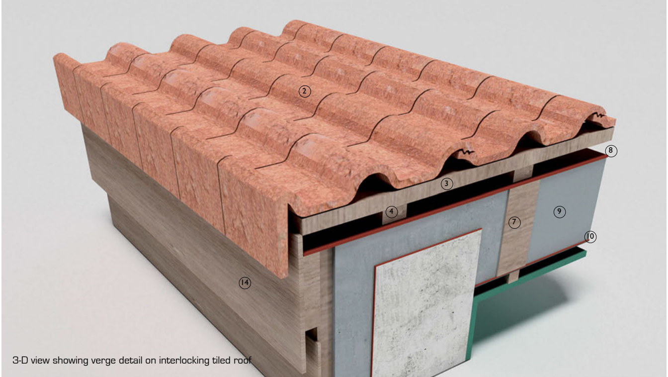
Vertical section 1:10. Interlocking tiles. Verge
