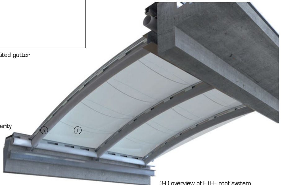
3-D overview of ETFE roof system
