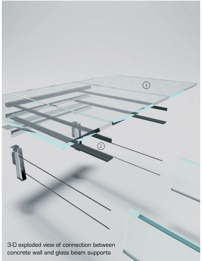
3-D exploded view of glass beam with central steel support beam
