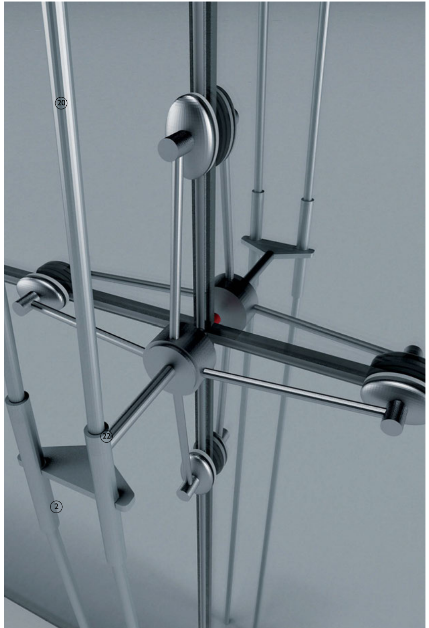
3-D detail view of glazing supported by spider clamp hung from cable truss
