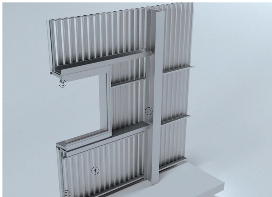
3-D view of rear of recessed aluminium window in profiled metal facade
