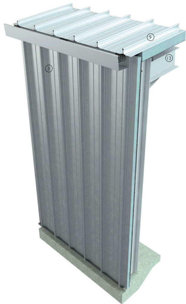
3-D view of vertically set profiled metal sheet
