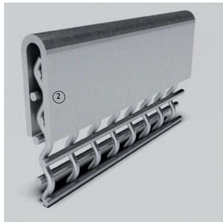
Vertical section 1:2. Edge fixing variations for rigid mesh supported on frame
