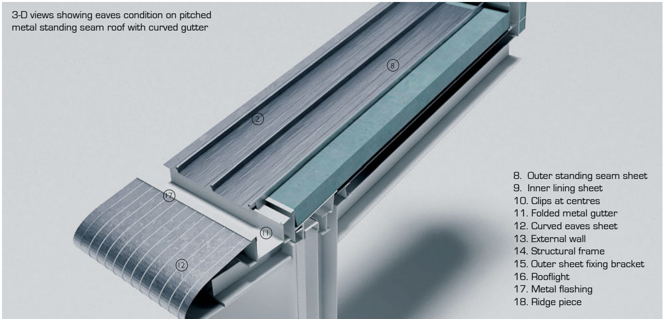
Vertical section 1:10. Eaves with curved gutter
