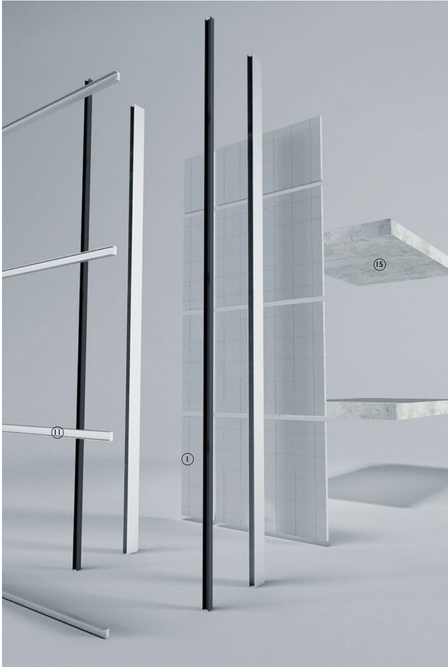
3-D exploded view of top of glass block facade system and floor slab connections
