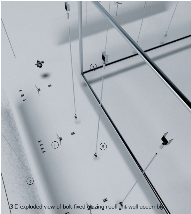
3-D exploded view of bolt fixed glazing rooflight wall assembly
