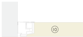
Horizontal section 1:5. Joint between composite panel and concrete wall with fully interlocking connection
