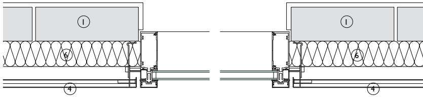
Horizontal section 1:10. Connection between metal rainscreen and curtain wall type glazing with flush finish
