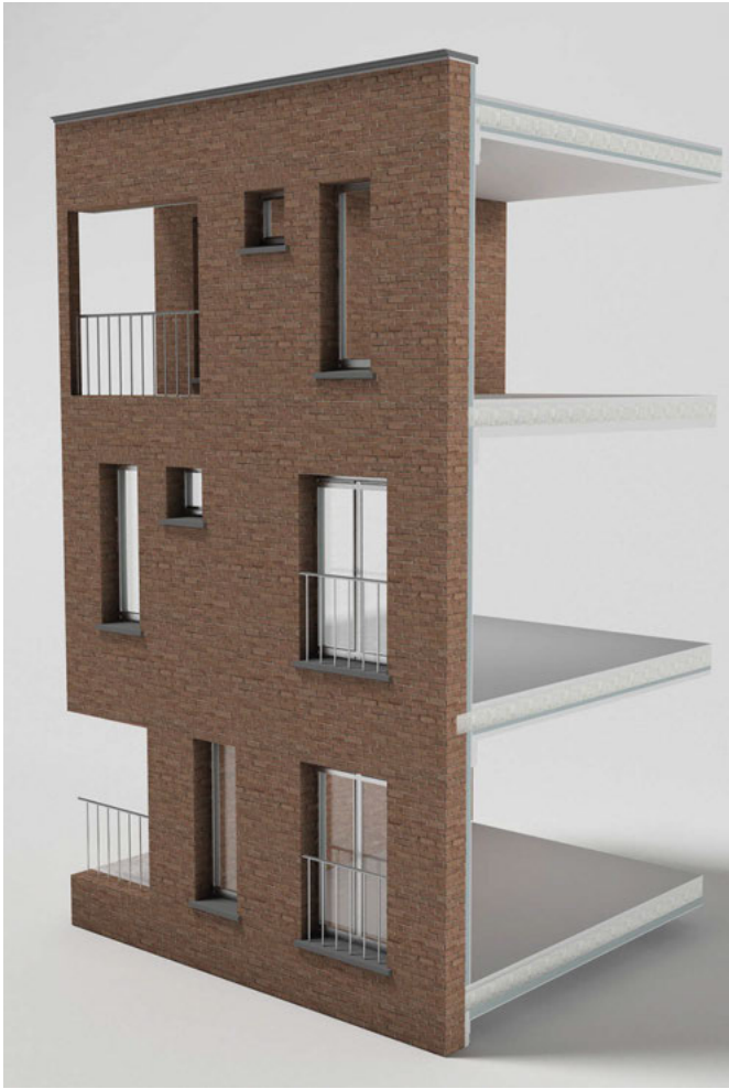
3-D view of loadbearing brick wall
