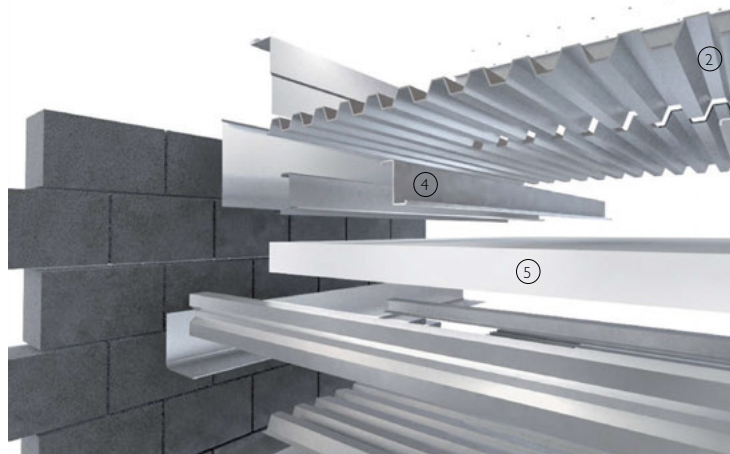
3-D exploded detail view of profiled metal sheet connection to blockwork wall
