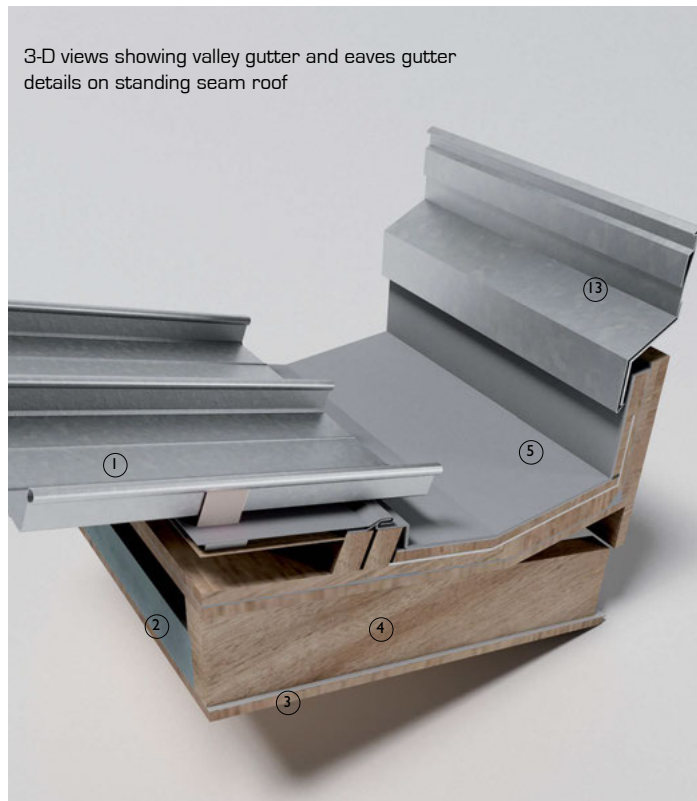
Vertical section 1:10. Standing seam roof. Valley gutter
