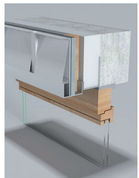
3-D views showing recessed timber window opening in metal rainscreen shingle cladding system
