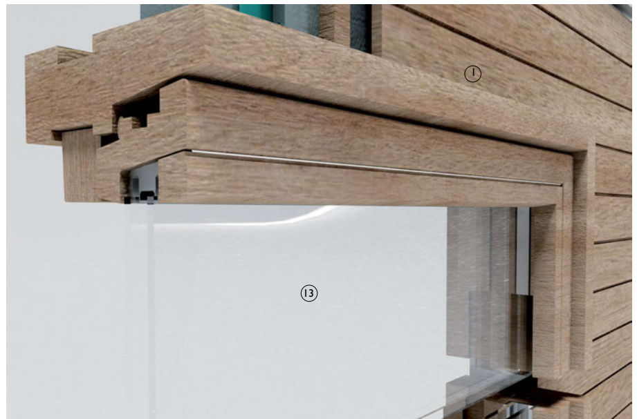
Vertical section 1:25. Cladding panel in twin wall configuration for taller buildings.
