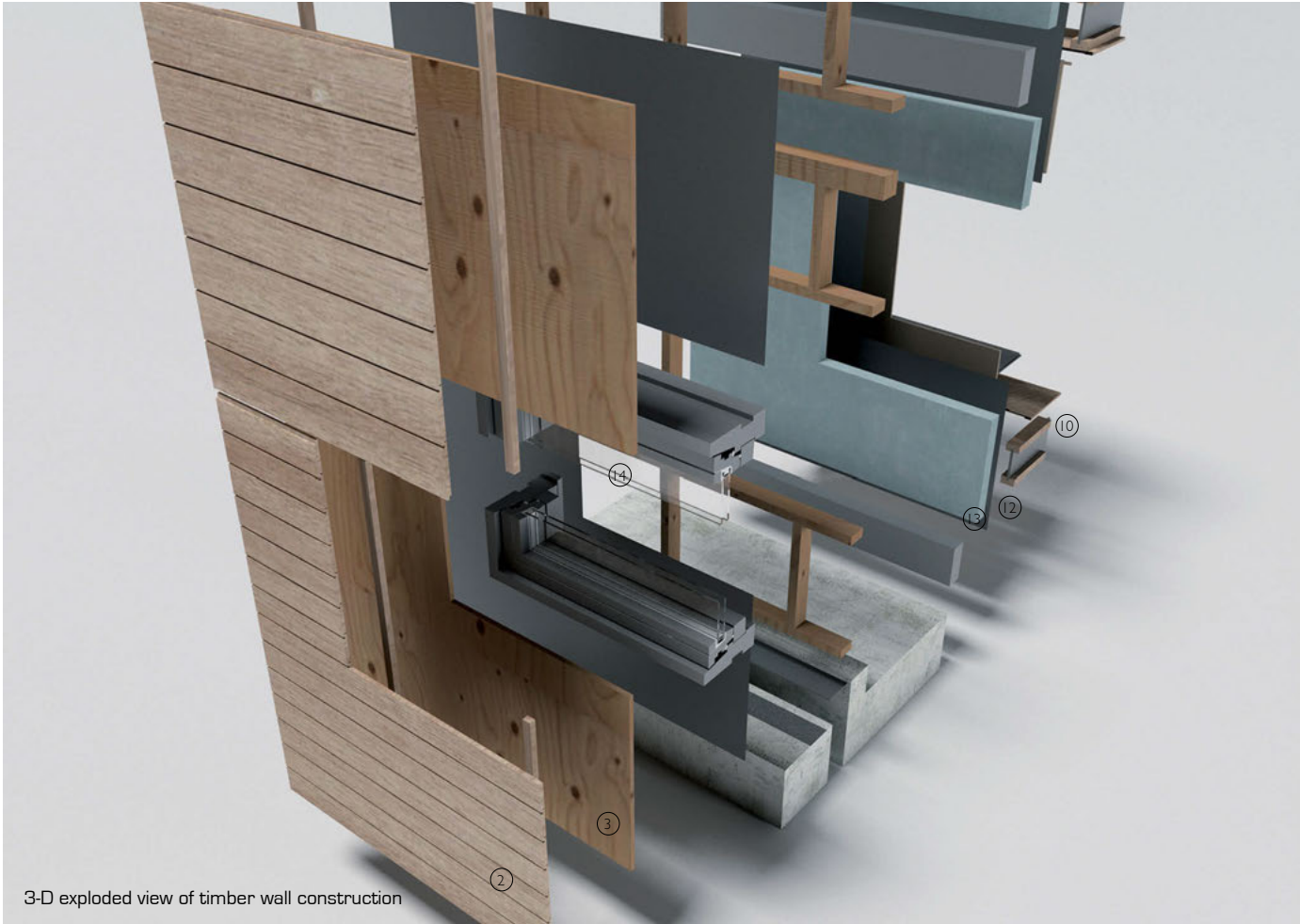
Exploded axonometric drawing of timber wall construction
