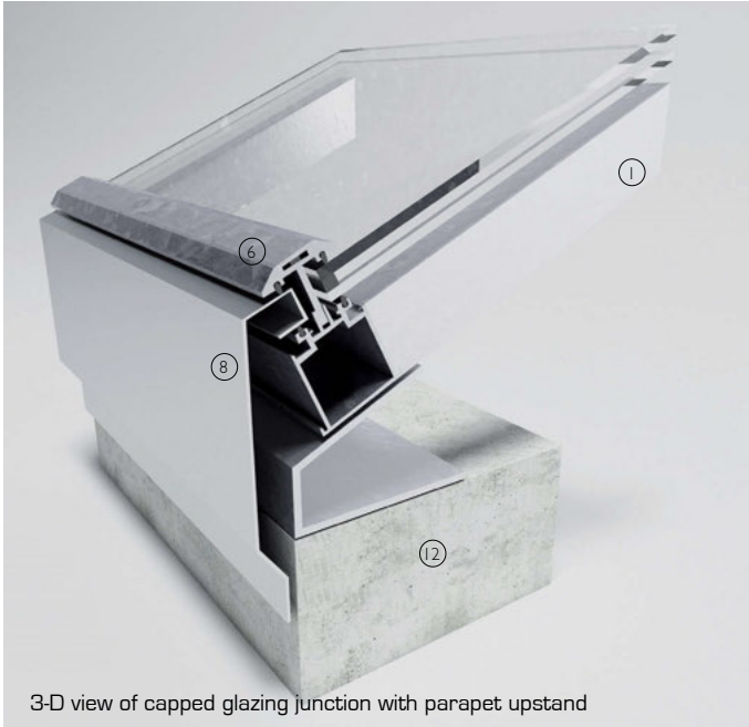
Vertical section 1:5. Capped glazing, parapet upstand detail
