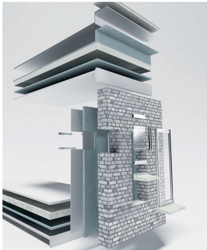
3-D exploded view of loadbearing masonry construction
