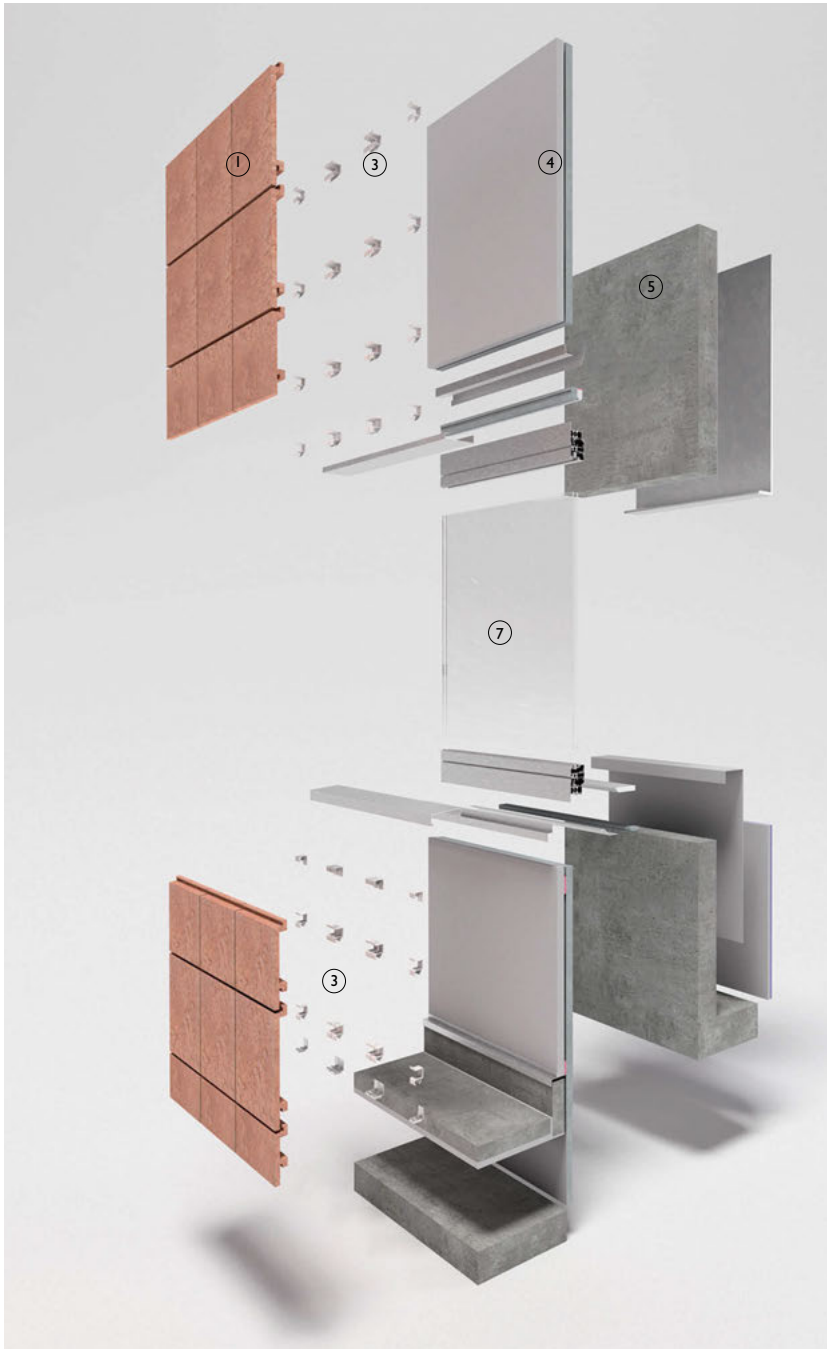
3-D exploded view of terracotta rainscreen facade held in place with individual support clips
