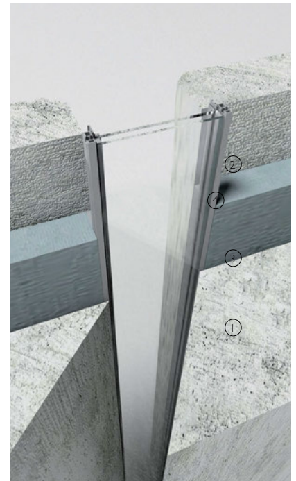
3-D view of in-situ cast concrete wall cast in two skins with rigid closed cell insulation between skins
