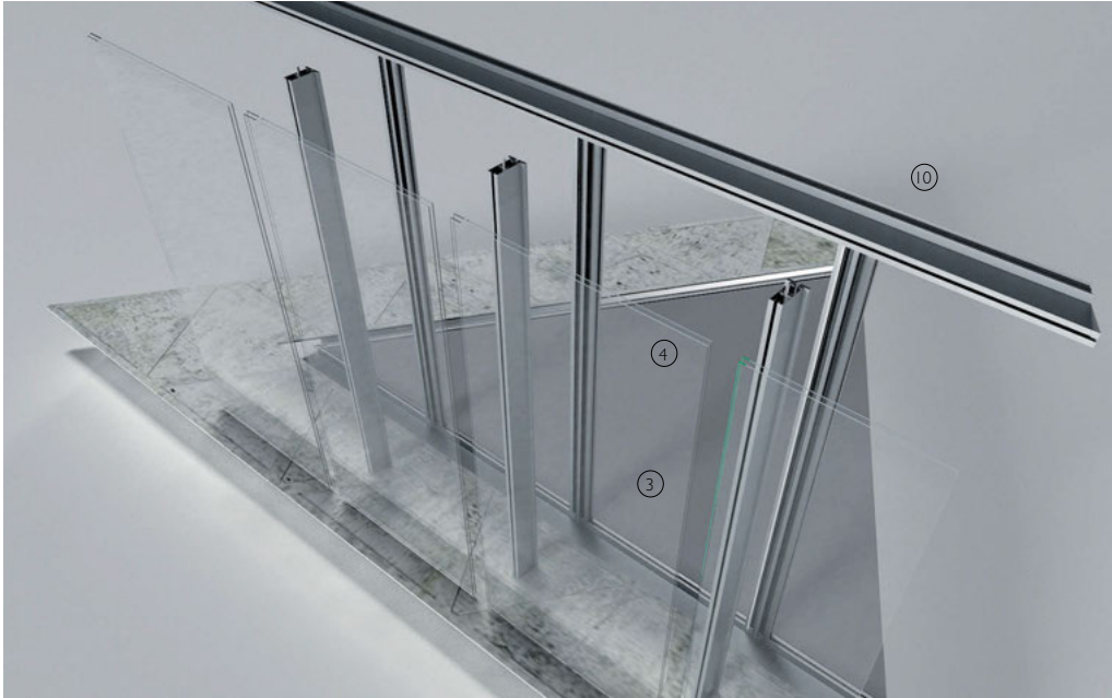
3-D exploded view of unitised window components
