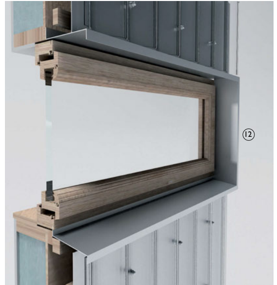
3-D section detail of polycarbonate rainscreen
