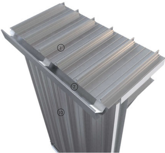
3-D view of flat profiled metal sheet roof construction
