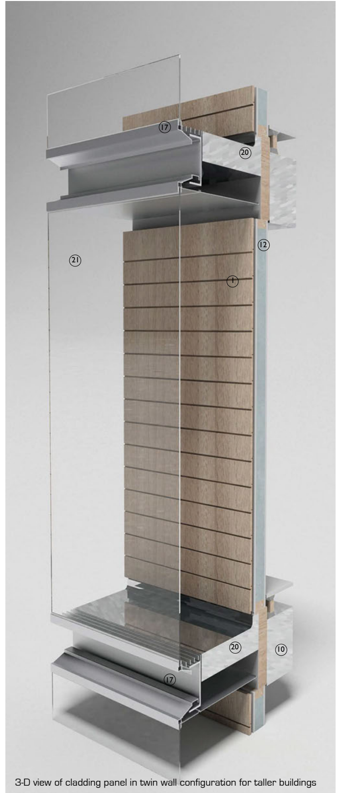
3-D detail view of floor junction in twin wall configuration for taller buildings
