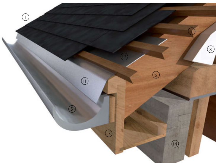
3-D view of timber pitched roof construction with roofing slates with gutter at eaves
