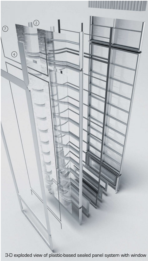
3-D exploded view of plastic-based sealed panel system
