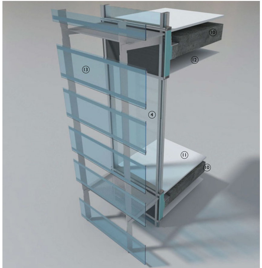
3-D view of glazed curtain wall with maintenance walkway and glazed solar shading panels in front
