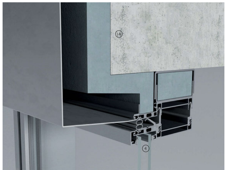
3-D view of unitised panel connection to underside of floor slab
