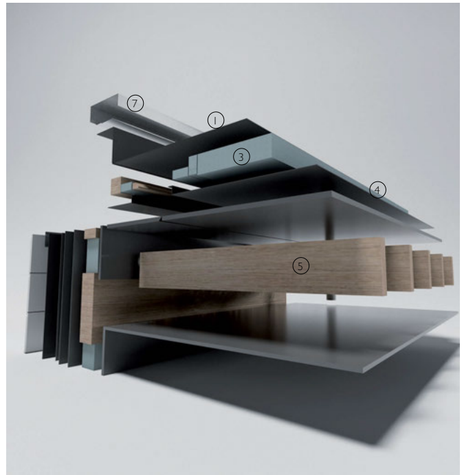
3-D exploded views of typical flat timber roof construction with rigid insulation above roof structure
