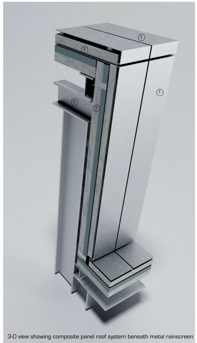
Isometric view showing composite panel roof system with metal flashing
