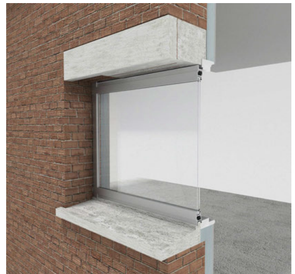
3-D view of window detail
