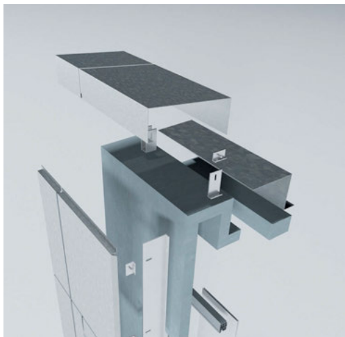
3-D exploded view of parapet condition
