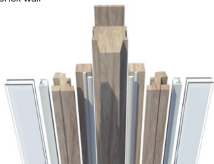
3-D exploded views of various timber window construction configurations
