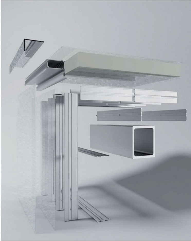
3-D line drawing of small rooflight
