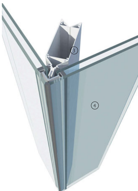
3-D view of framed external corner detail
