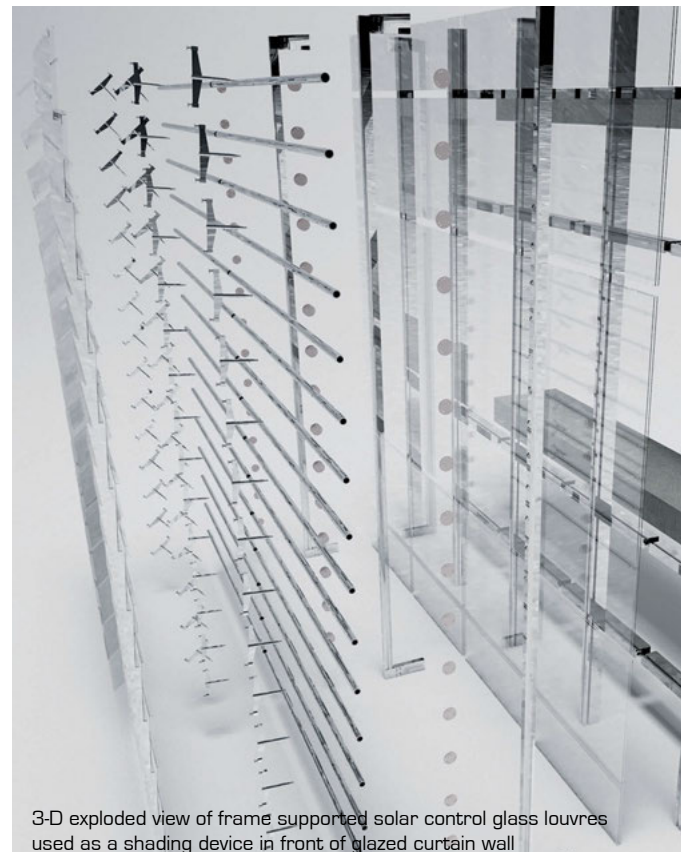
3-D detailed views of frame supported solar control glass louvres used as a shading device in front of glazed curtain wall
