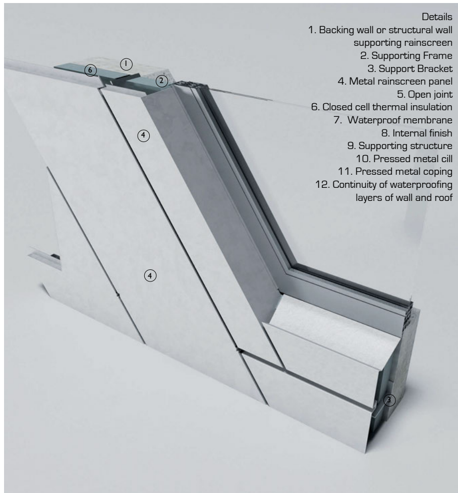
3-D view of semi interlocking metal rainscreen with angled joints and aluminium window recessed into the facade. Type 3
