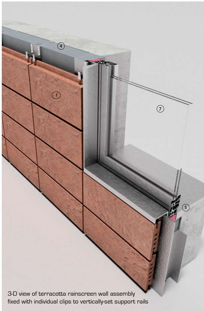
3-D view of terracotta rainscreen wall assembly fixed onto vertically-set support rails
