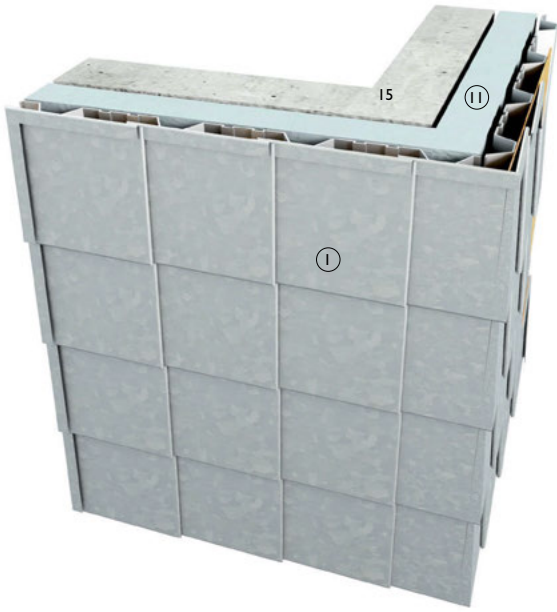
3-D view of folded metal sheet with recessed seams. Type 4
