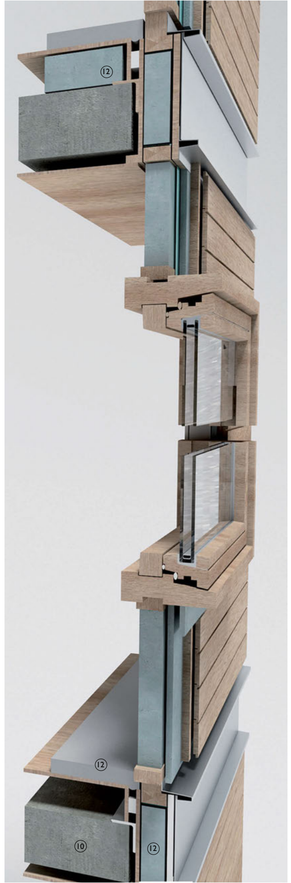
3-D sectional view of timber louvre cladding panel and junction with upper floors
