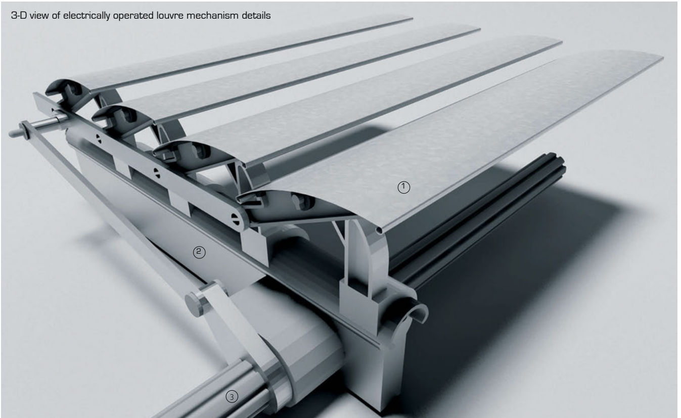
Vertical sections 1:20. Louvre mechanism details
