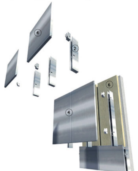
3-D exploded view of rainscreen panel system
