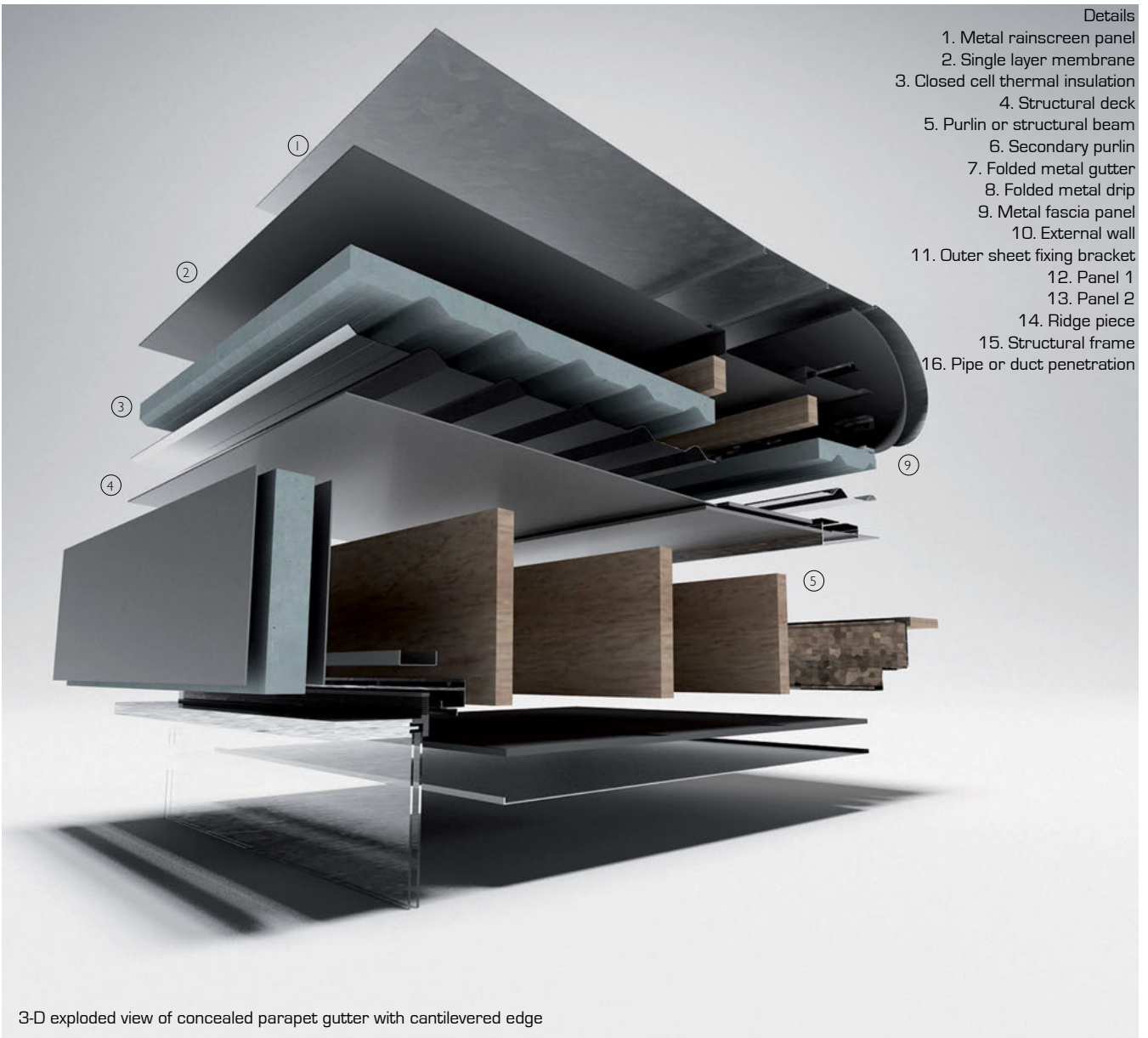
Exploded axonometric view of concealed parapet gutter with cantilevered edge
