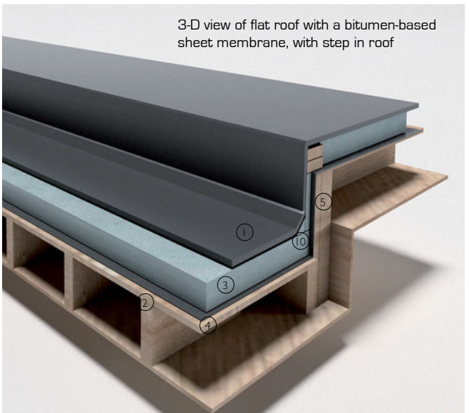
Vertical section 1:10. Step in roof
