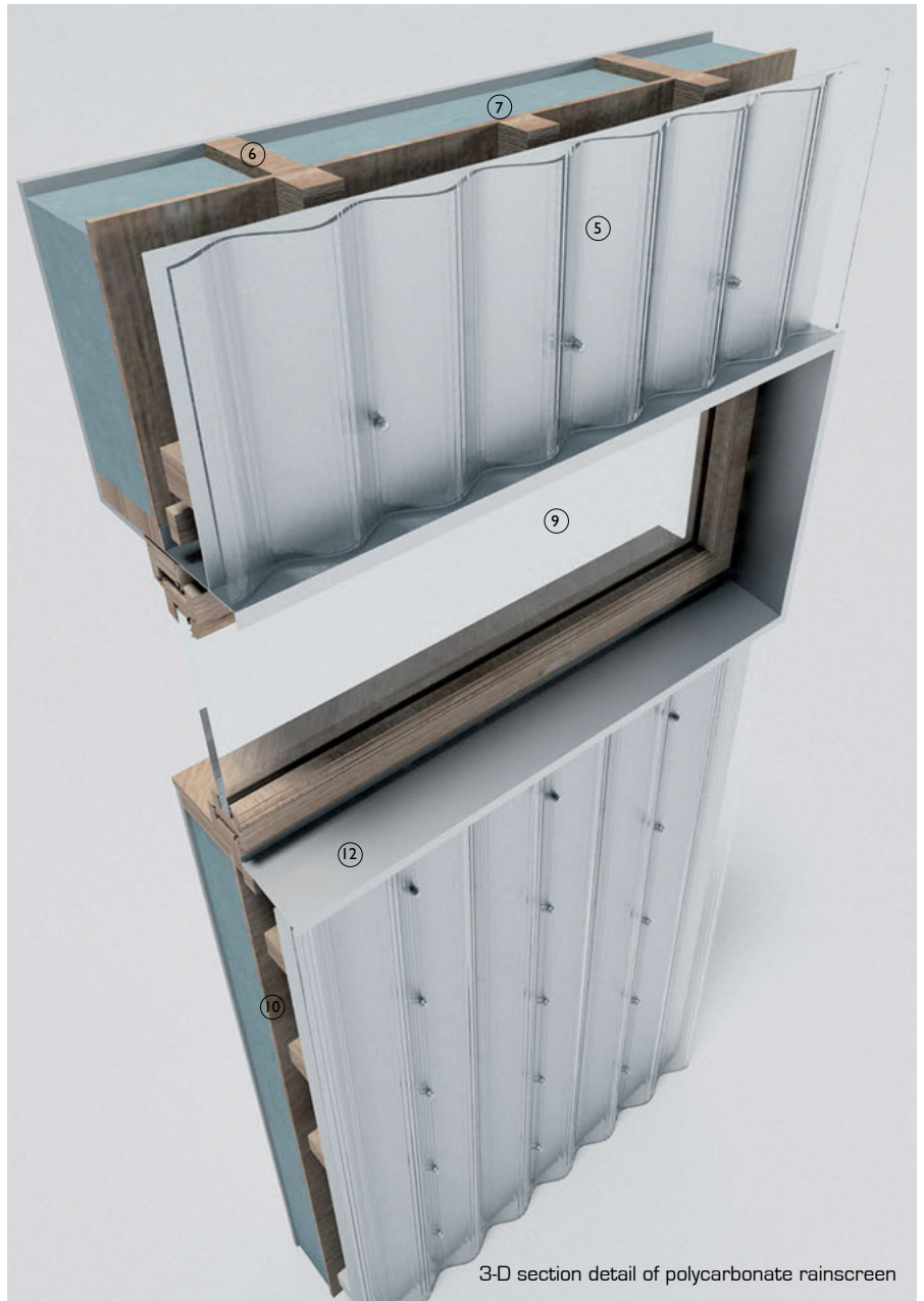
3-D section detail of polycarbonate rainscreen
