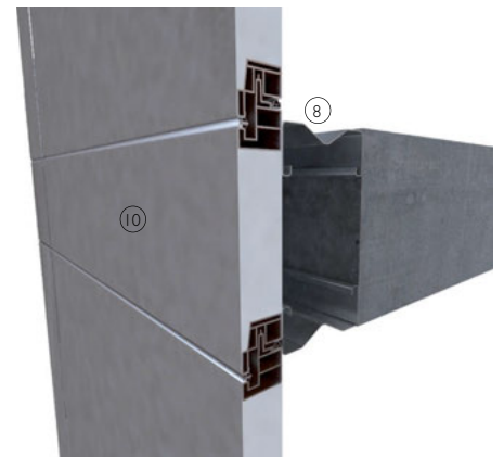
3-D view of spandrel panel connection
