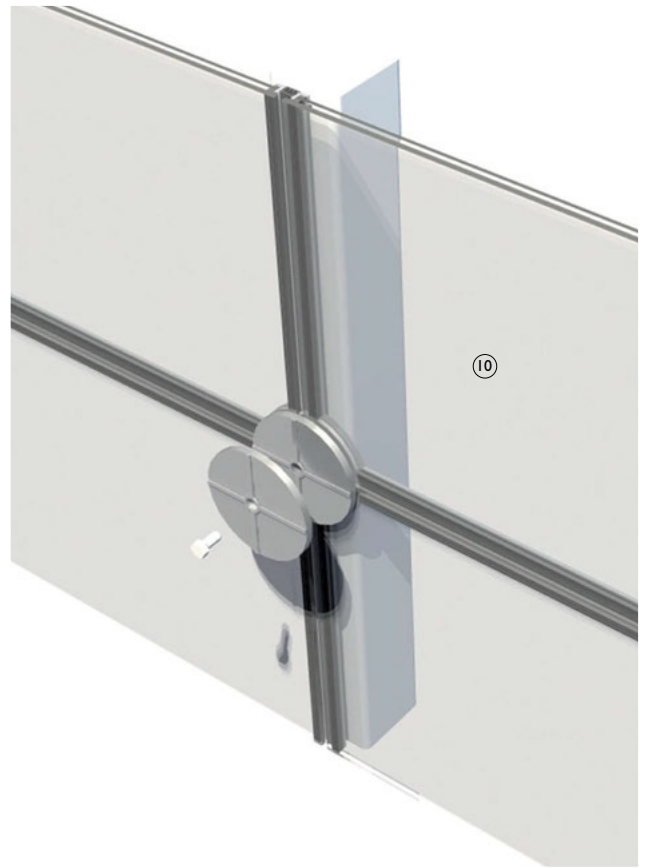
3-D view of corner clamped glazing system
