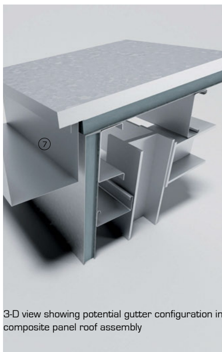
Vertical sections 1:25. Various gutter configurations in composite roof panels
