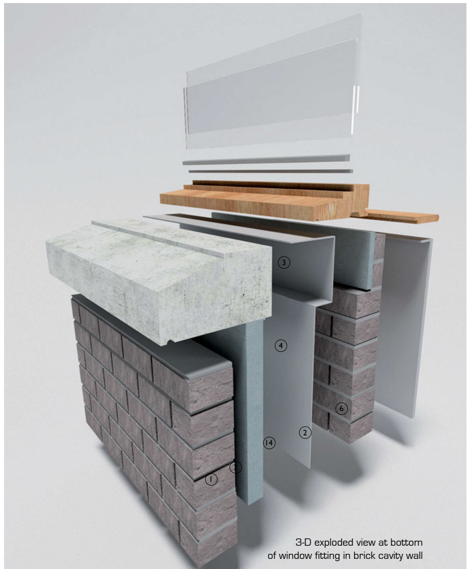
3-D view at bottom of window opening in brick cavity wall
