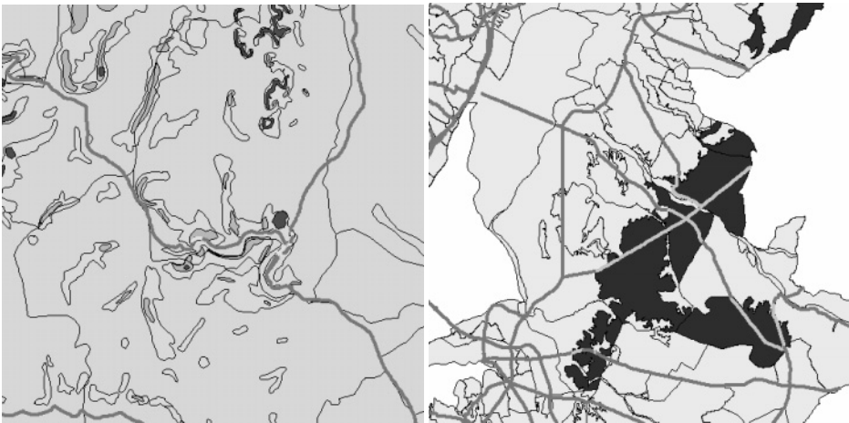
Fig. 2.22. Damages in the roadway lifeline caused by slope sliding (on the left side) and due to liquefaction (on the right side) (light gray: no problem; darker: higher potential for sliding/liquefaction)
