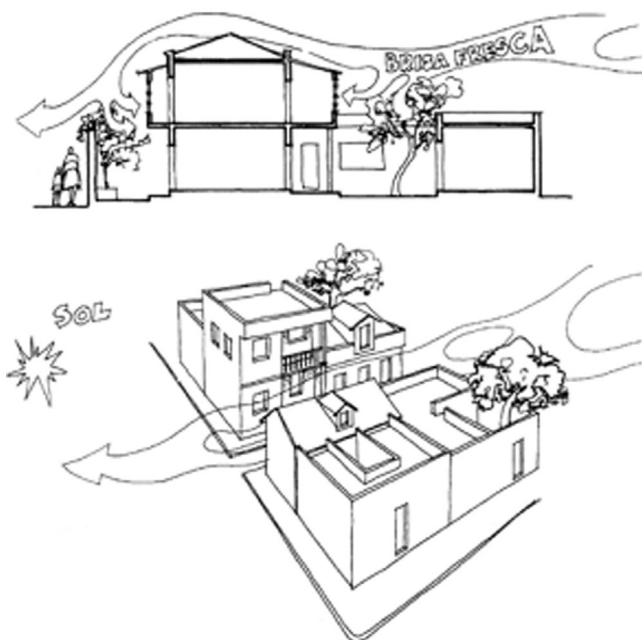
FIGURE 16.19 Ventilation has a fundamental role: one should focus on solutions to optimize air circulation. The use of the courtyard-house typology is an effective measure in dryer climates such as in regions of Angola, Cape Verde and Mozambique.
