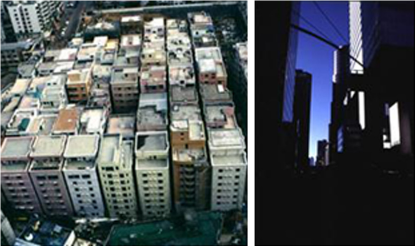
FIGURE 9.8 Narrow street canyons reduce daylighting (left: Shenzhen, China, right: New York, USA).
