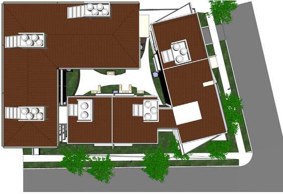
FIGURE 8.35 Top view of the new housing building with solar hot water systems on each humid nucleus.
