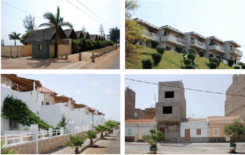
FIGURE 16.21 Top figure (1): residential areas in Maputo, Mozambique: the twinning of houses reduces the area of sun exposure, reducing the risk of overheating. Below (2): left: geminated houses in Sal, Cape Verde; right: a dominant façade an area of contributes to situations of discomfort from overheating.
