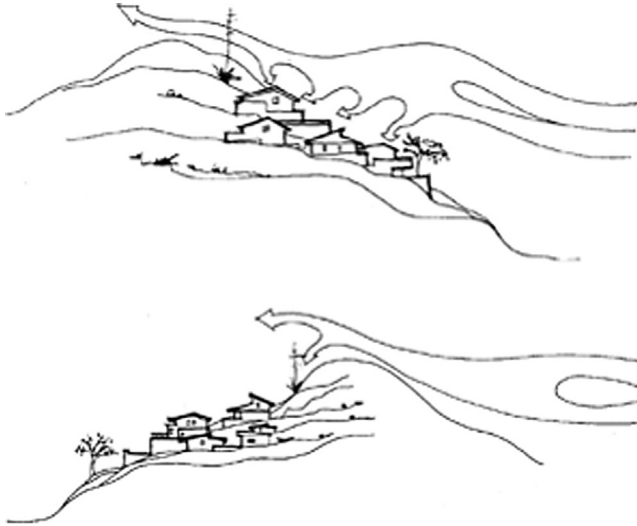
FIGURE 16.15 On a hillside location, we must study the prevailing winds, in order to maximize the potential for indoor ventilation.
