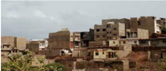
FIGURE 16.52 Suburban area in the island of Santiago, Cape Verde: the use of light-colored paint would be an inexpensive strategy to reduce discomfort due to overheating.
