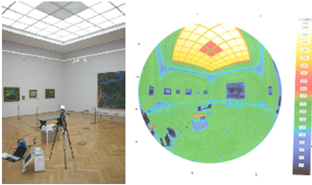
FIGURE 9.3 Comparison of a conventional photograph and a High Dynamic Range Photograph, showing the luminance distribution in false colors (museum room).
