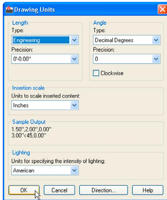
Fig. 4.25 Settings for Imperial dimensions in the Primary Units dialog
