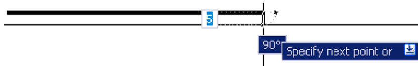
Fig. 3.28 Dynamic Input – first example – Polyline – the horizontal length
