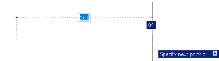
Fig. 3.20 Drag the cursor to the required point and left-click
