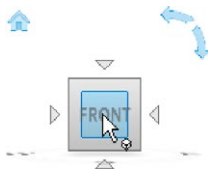
Fig. 16.10 Set screen to the ViewCube/Front view
