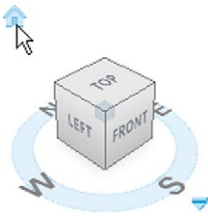
Fig. 16.18 Set screen to a ViewCube/Isometric view
