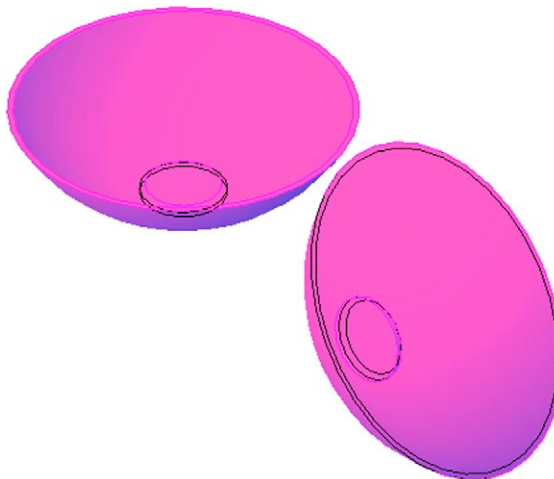
Fig. 14.19 Second example – 3D Mirror – the result in a front view
