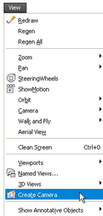
Fig. 15.44 Selecting Create Camera from the View drop-down menu
