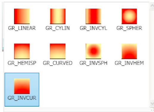
Fig. 8.14 The Gradient patterns in the Hatch Creation/Pattern panel
