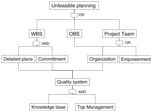
Fig. 14.1 Example of fault tree analysis
