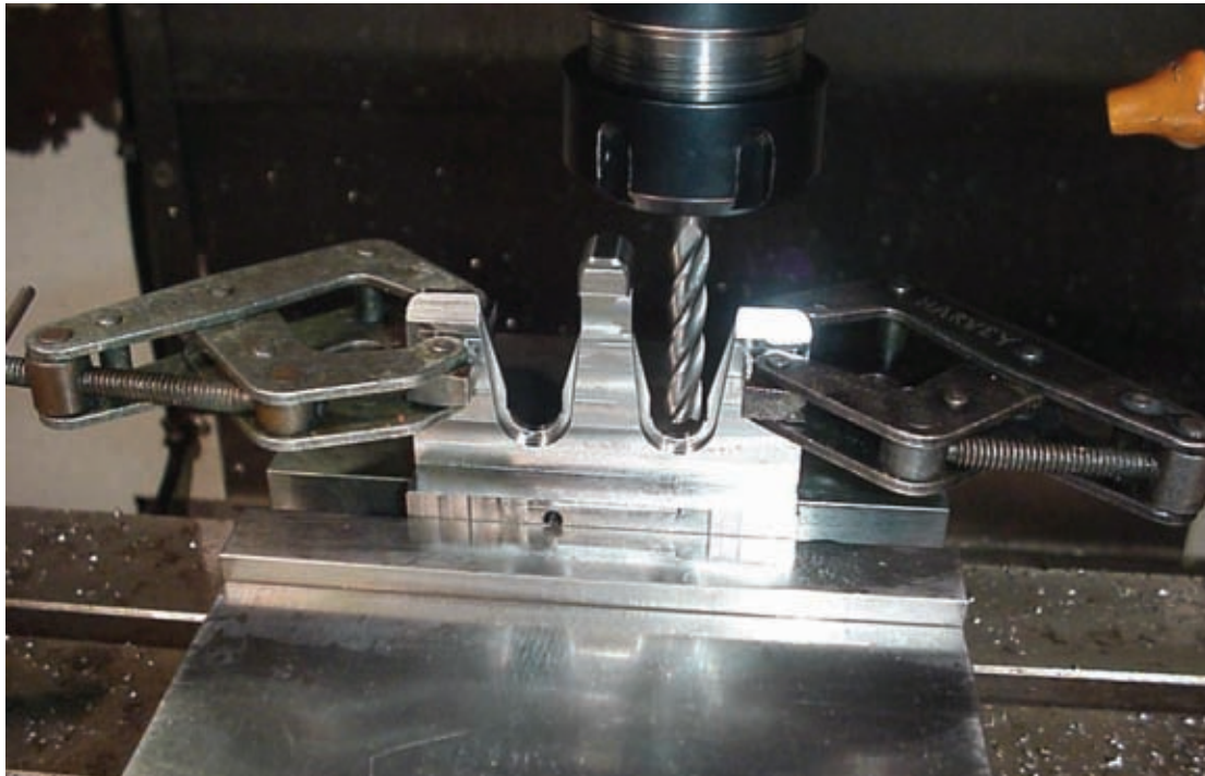
Figure 10-23 Vibration can be reduced or eliminated by adding weight to a part or some feature of a part. In this case, clamps were used to add weight to the outside “ears” of the part, which eliminated the initial vibration.
