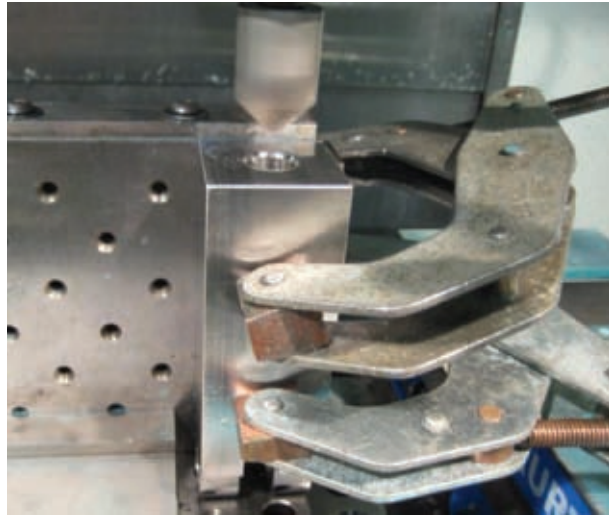
Figure 10-17 Without precise dimensions for a countersink tool, programming a proper depth for the tool would be a guessing game. I've found it easier to let the machinist, at the machine, find the right depth. Once found, the machinist can enter the value in the program.
