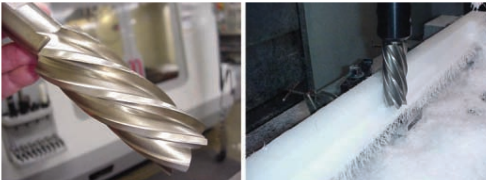
Figure 10-7 A negative rake end mill is being used to machine a long flimsy bar. The downward cutting force helps hold the bar in place.
