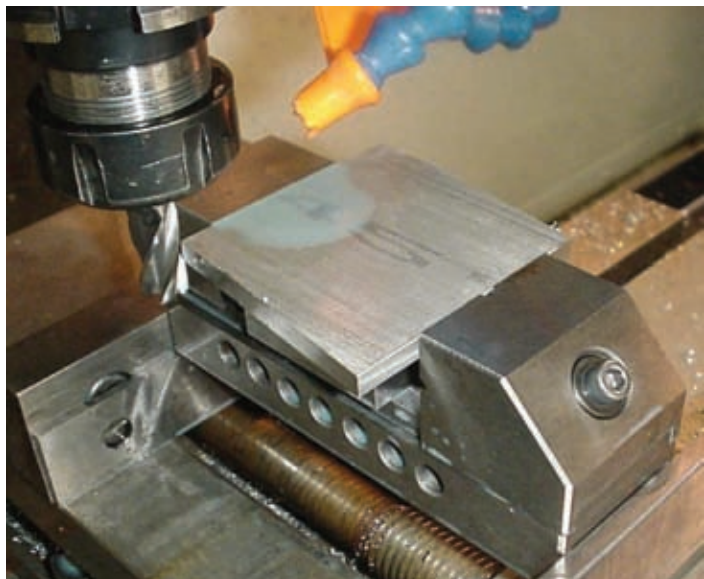
Figure 10-20 Grinding vises seem to come in handy for a lot of setups. One is being used here to hold a part so both ends of the part can be machined in one setup.
