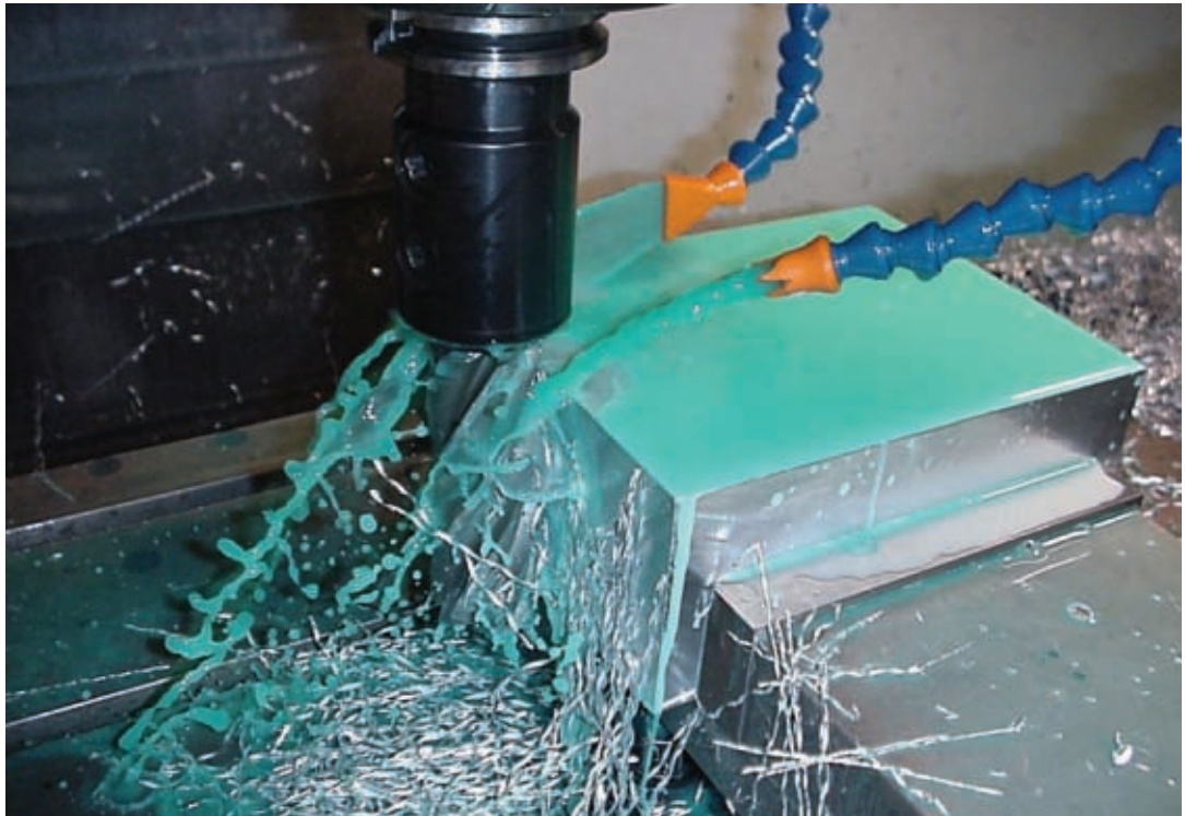
Figure 1-9 Side milled surfaces are more prone to inaccuracies than face milled surfaces, especially when using long end mills.
