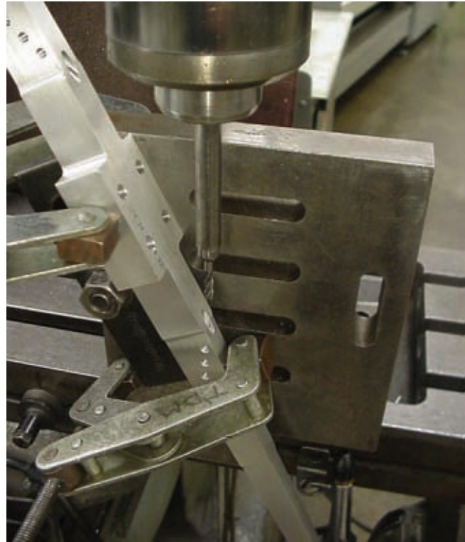
Figure 7-2 Cutting holes into a tilted part using a conventional milling machine.
