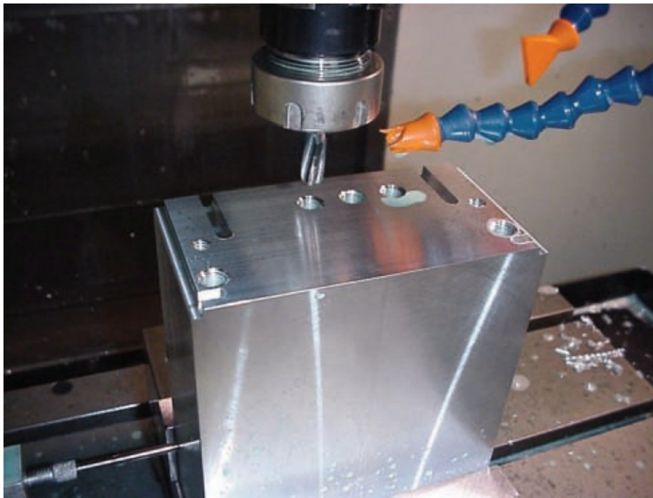
Figure 1-11 Sometimes it is wise to focus on getting precision blanks before adding features. The mold cavity above was precisely squared to size before doing any other machining operations.
