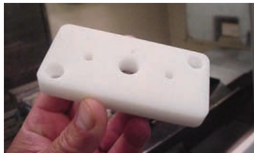
Figure 6-2 This is the finished adapter plate we’ll be modeling, programming, and machining. It’s a simple part, but once you can make one of these using CAD/CAM equipment, you’ll have a good foundation for producing more complex parts.
