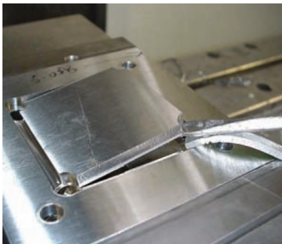
Figure 3-11 I'm cheating here by manually removing the remnant. In hind sight, I could have used a smaller diameter end mill to run around the window to cut the remnant free.
