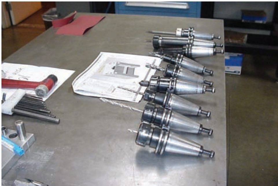
Figure 3-2 It's a good idea for machinists to physically lay out all the tools used in a program in sequential order before installing them in a machine. Most tool numbering errors can be caught early in this way.
