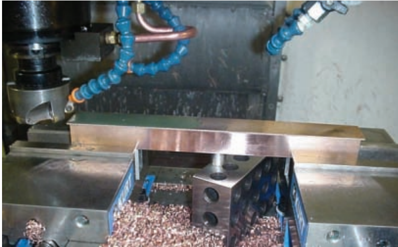
Figure 2-3 A 2-4-6 block in combination with a gauge block stack is used to support the center section of a bar so it doesn't "push away" during the cut..
