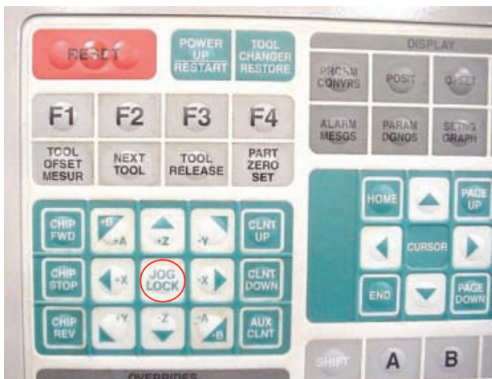
Figure 9-13 The JOG LOCK button engages the machine to run along the axis of your choice so you don’t have to crank the handle dial.
