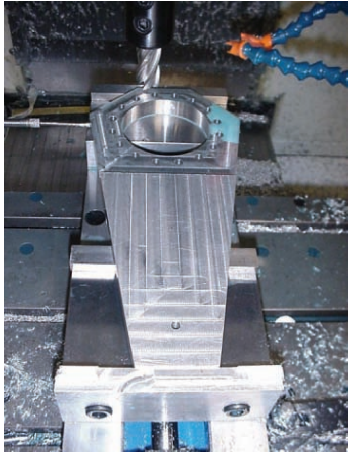
Figure 1-6 Plan to use a vise when possible. Holding parts in a vise eliminates the need for time- and material-consuming fixtures.
