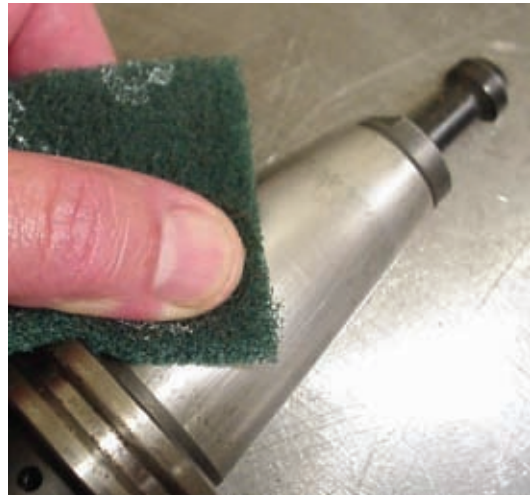
Figure 10-2 Scotch Brite™ is used to remove rust from this tool holder.
