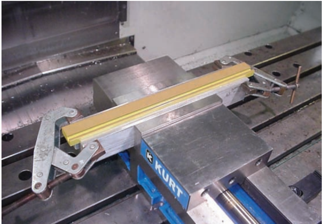
Figure 2-10 Long jaws such as these come in handy for holding parts that extend beyond the vise jaws.
