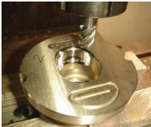
Figure 10-5 Light cuts were used to rework this hardened part using a carbide cutter.
