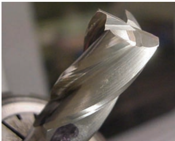
Figure 8-22 Hog nose end mills cut with less pressure than ball nose end mills.
