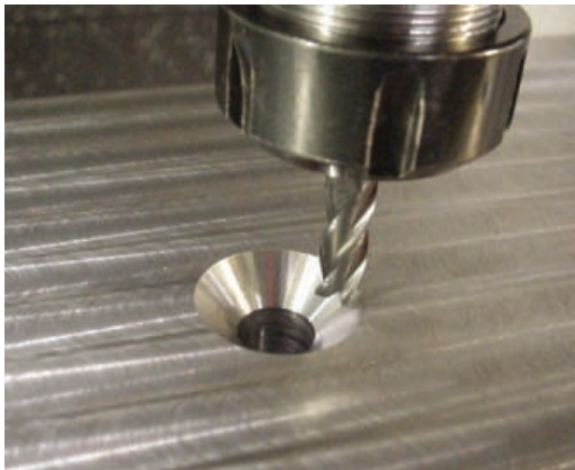
Figure 10-14 Though not a common practice, countersinks can be 3D milled. A 1/2" diameter hog nose end mill was used to machine this feature .
