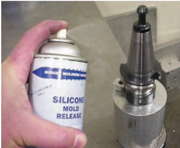
Figure 10-1 Silicone mold release is sprayed on a tool holder for easier tool changes.
