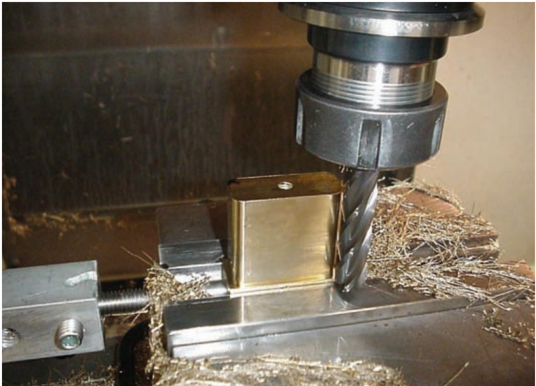
Figure 1-10 Small, stocky parts are less prone to warping than thin hogged-out parts.
