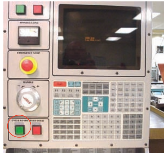
Figure 9-7 When you're ready to run your program, press the CYCLE START button.
