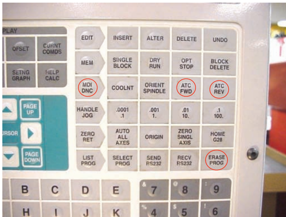
Figure 9-3 The MDI , ATC FWD, and ATC REV buttons all help with changing tools.
