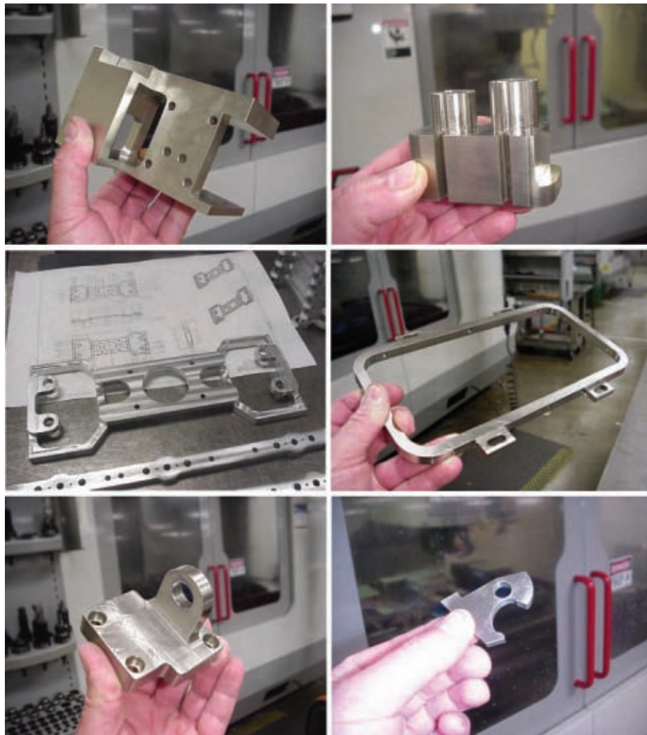
Figure 8-12 These parts were all made using nothing more than the commands described thus far. The programs to make these parts, however, were generated using CAM software.
