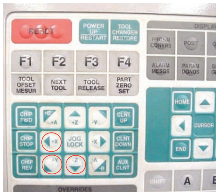
Figure 9-11 Once in Handle Jog mode, you can move or cut along an axis of your choice.
