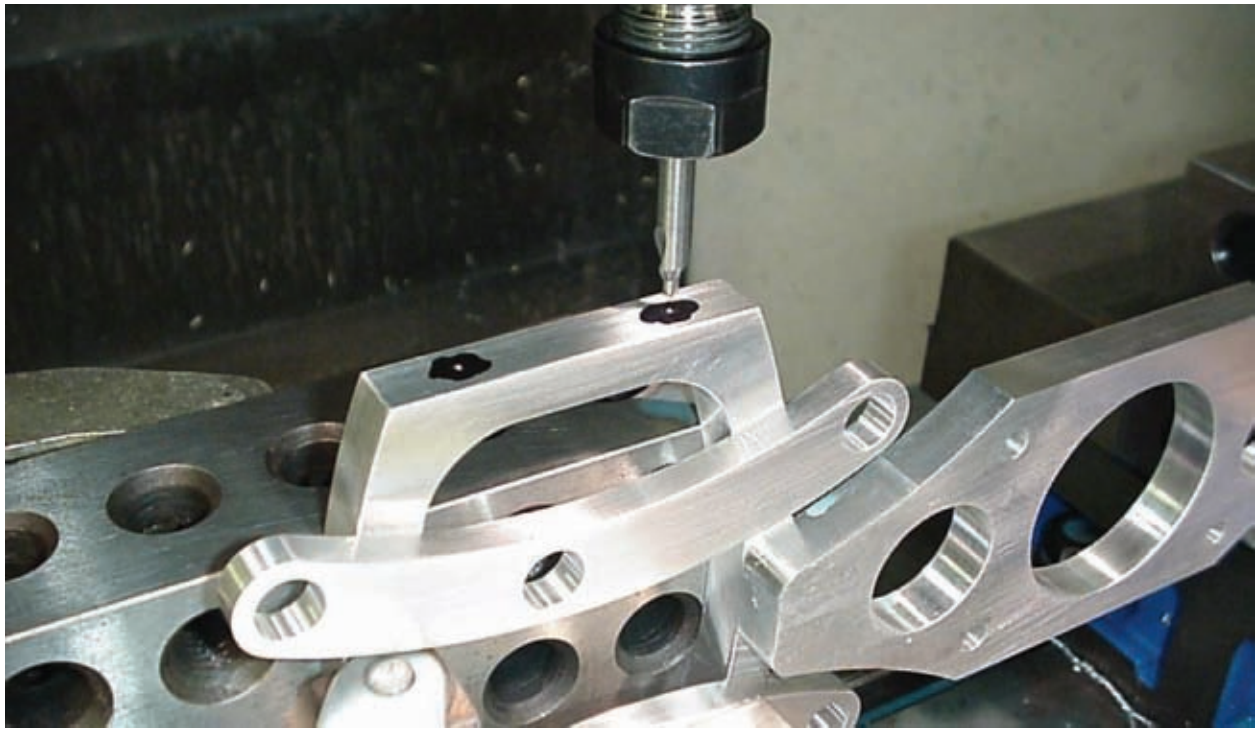
Figure 10-16 One way to make sure holes are in the correct locations is to set center drills to lightly spot the surface.
