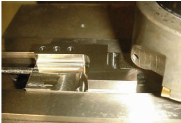
Figure 10-4 A final pass with the initial facing tool helps remove burrs.
