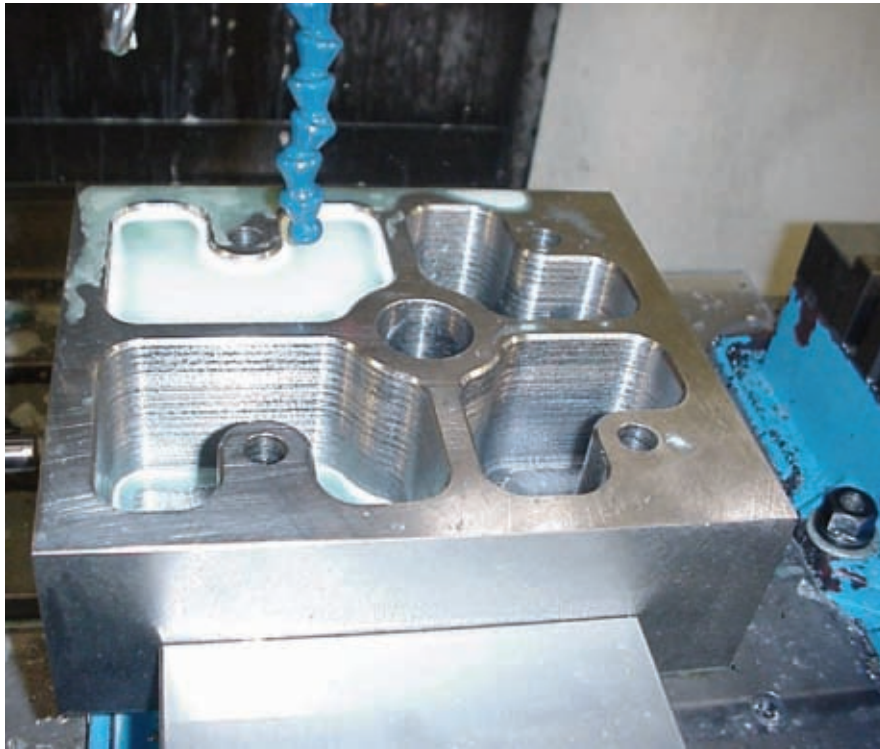
Figure 10-19 The machine's air nozzle is set up to blow trapped chips and coolant from the pockets in this part.
