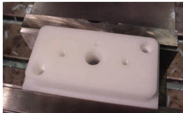
Figure 8-11 This is the adapter plate after all the tools have been run. The only thing left to do is face off the back side and bring the part to the correct thickness.
