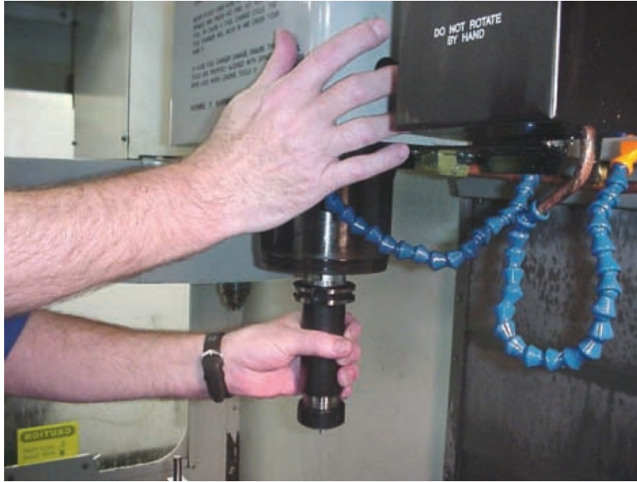
Figure 9-4 When installing a tool manually, line up the lugs.
