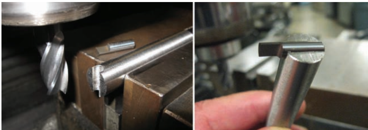
Figure 10-12 Sometimes custom cutters are needed to machine unusual features. These photos show a custom cutter under construction.
