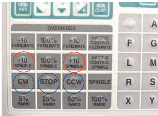
Figure 9-8 The buttons for increasing and decreasing SPINDLE speed are circled in red. The buttons for stop, CW, and CCW are circled in blue.
