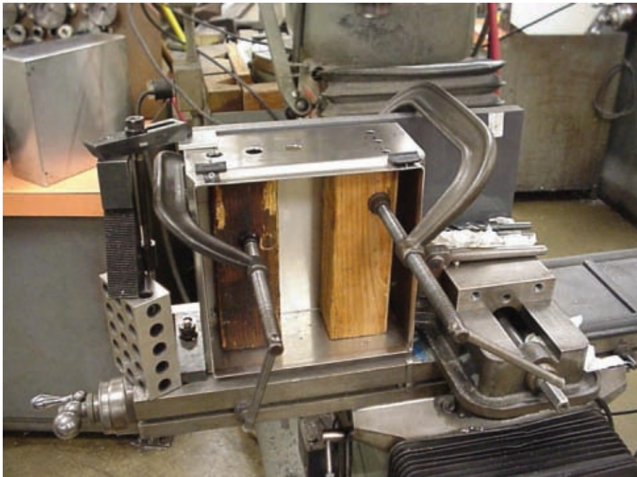
Figure 2-6 Sheet metal parts are often difficult to hold for further machining.
