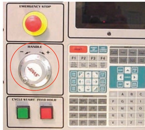
Figure 9-10 The main dial for moving the table manually.
