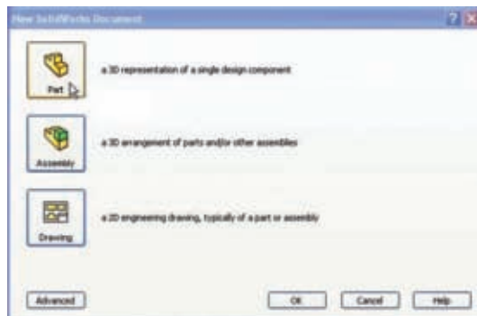
Figure 6-5a Select what you want to create. In this case, we want to model a “part” — the adapter plate.
