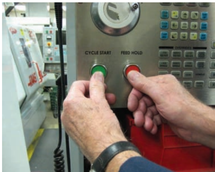
Figure 3-3 The machinist is being careful here by toggling between the cycle start button and the feed hold button as the cutter approaches the part. If there is a programming error, the machinist is in a good position either to catch the error before any material is cut or to reduce the damage the programming error may cause.
