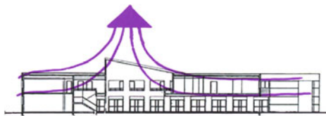
Figure 11. Natural ventilation of the building
