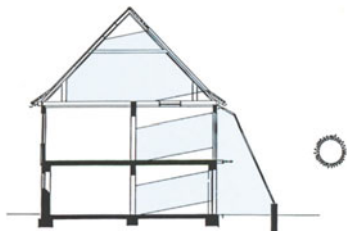
Figure 8. Direct gain on a winter's day with the shading devices open
