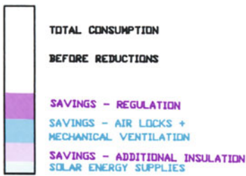
Figure 21. Reduction in annual energy requirements achieved in improved (Technosite) building compared with standard building
