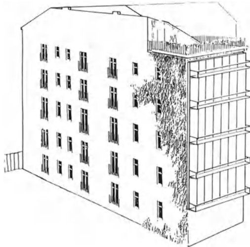
Figure 12. The TIS facade on side wing of 80 Naunynstrasse
