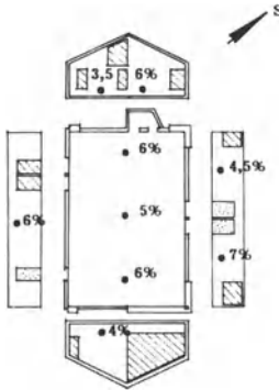
Figure 18. Daylight factors in multi-use room determined by on-site measurements on 18 January 1989
