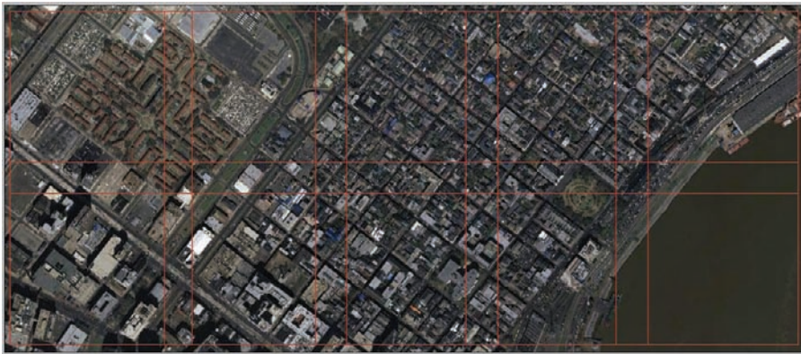
Figure 6.8. All downloaded images to be tiled must have areas of overlap with the adjacent images. This example has 10 images to be tiled.
