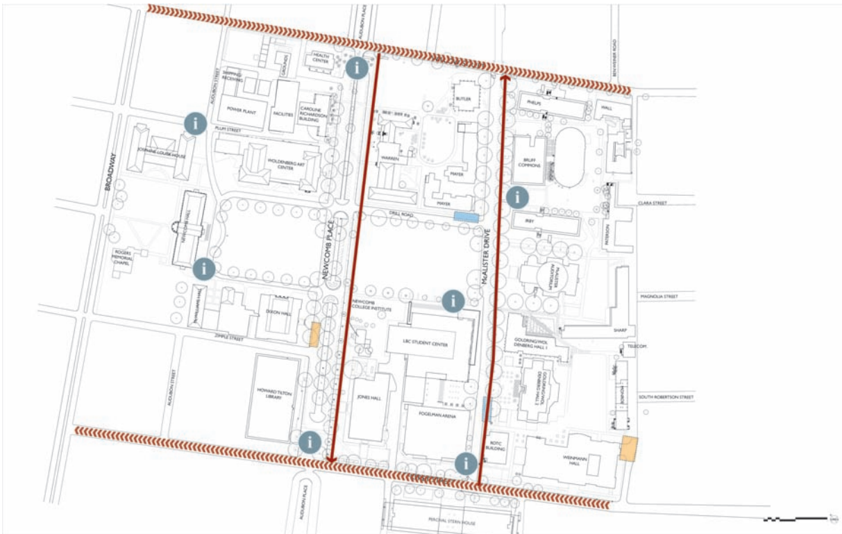
Figure 13.2. Once a symbol is created, drag it from the Symbols palette onto the drawing. The symbol can then be copied around the drawing to place the symbol instances.
