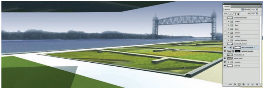
Figure 30.16. A layer mask crops the image, and an adjustment layer is clipped to the image in order to change the hue/saturation.
