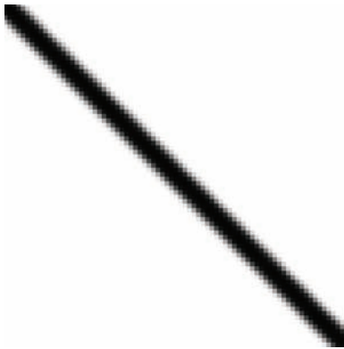
Figure 18.10. When the linework is imported from AutoCAD, it is rasterized. This means that the linework is converted to a set of pixels. To replicate the smooth edges of the linework, Photoshop adds some gray pixels along the edges of the lines. From a distance, this makes the lines appear smooth. Without these gray edges, the linework would appear jagged or harsh.
