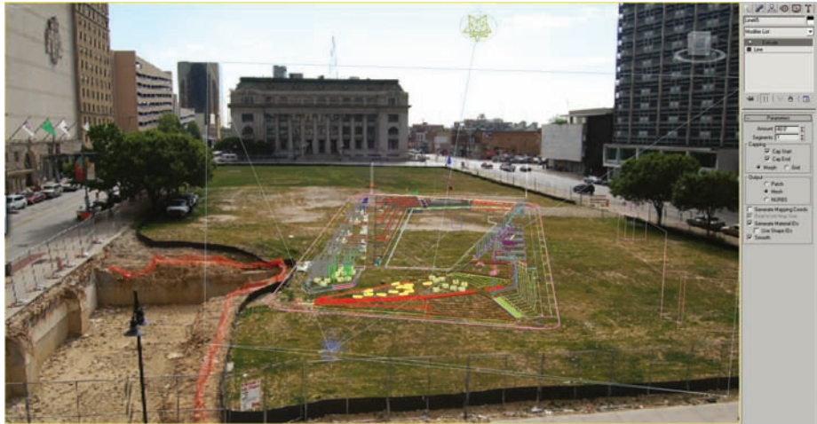
Figure 28.7. Model in relation to the image. Alignment points will be based on surrounding context.
