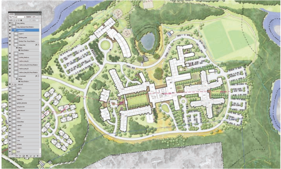
Figure 2.1. The ability to maintain and edit layers adds to the flexibility and editability of digital drawings.
