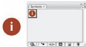
Figure 13.5. To redefine the symbol, hold the Alt key and drag the new geometry over the existing symbol in the Symbols palette.
