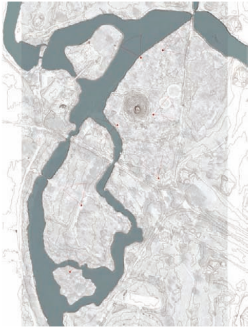
Figure 6.1. An aerial photograph altered in Photoshop to desaturate the image, combined with contour lines created in AutoCAD and water bodies on the site drawn in Illustrator.
