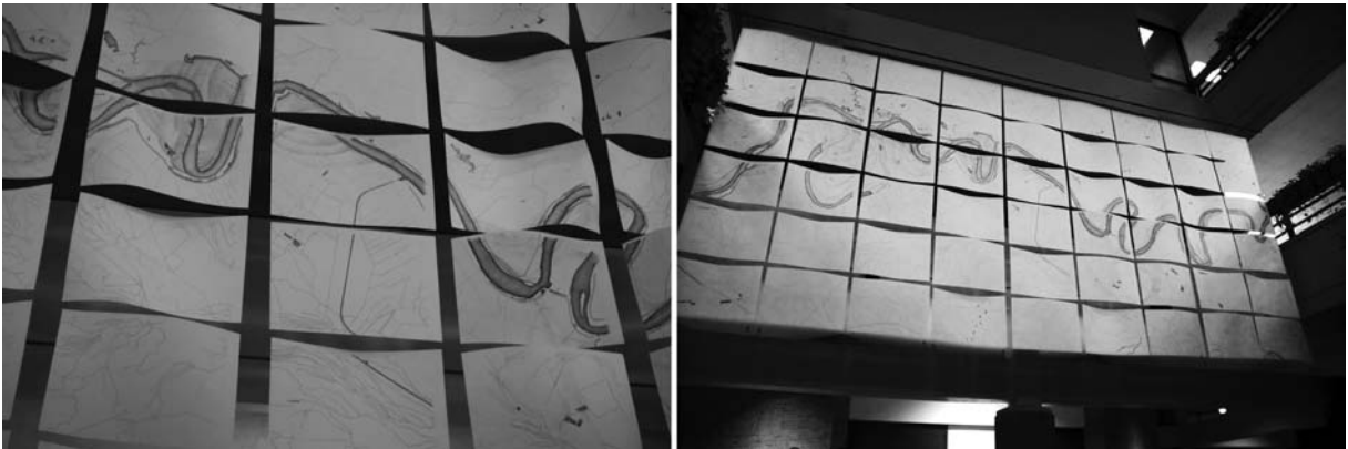
Figure 2.6. Geographical Information System (GIS) data is used to build a regional base plan that is printed across 54 sheets of drawing paper. Site features are then rendered with graphite to accentuate the expansive site.
