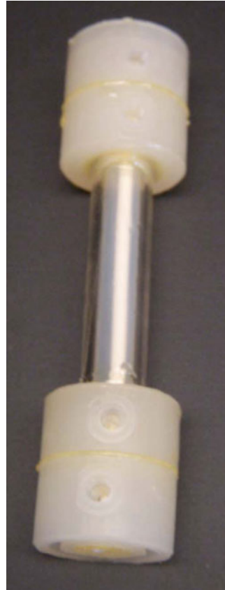
Fig. 5 Completed glued assembly
