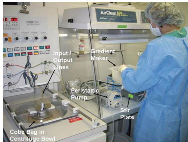
Fig. 6 Setup of the Cobe 2991 cell processor for the gradient separation of islets using Ficoll. The islets and the Ficoll gradient are added to a gradient maker and then pumped into the Cobe bag for eventual separation of the islets from the acinar tissue
