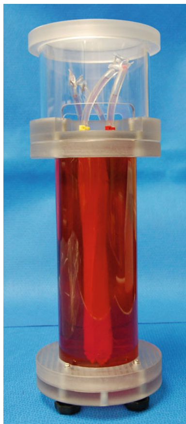
Fig. 2 Bioreactor with scaffold prepared for shipping. Tubing on barb fittings protected from physical damage by shroud. The vessel is completely filled with fluid medium
