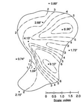
Figure 7.2.11 (a) Computation of areal average rainfall by the arithmetic-mean method for a 24-hr storm. This is the simplest method of determining areal average rainfall. It involves averaging the rainfall depths recorded at a number of gauges. This method is satisfactory if the gauges are uniformly distributed over the area and the individual gauge measurements do not vary greatly about the mean (after Roberson et al. (1998)); (b) Computation of areal average rainfall by the Thiessen method for 24-hr storm. This method assumes that at any point in the watershed the rainfall is the same as that at the nearest gauge, so the depth recorded at a given gauge is applied out to a distance halfway to the next station in any direction. The relative weights for each gauge are determined from the corresponding areas of application in a Thiessen polygon network, the boundaries of the polygons being formed by the perpendicular bisectors of the lines joining adjacent gauges for J gauges; the area within the watershed assigned to each is A_j and P_j is the rainfall recorded at the j th gauge. The areal average precipitation for the watershed is computed by dividing the total rainfall volume by the total watershed area, as shown in the table (after Roberson et al. (1998)). (c) Computation of areal average rainfall by the isohyetal method for 24-hr storm. This method connects isohyets, using observed depths at rain gauges and interpolation between adjacent gauges. Where there is a dense network of rain gauges, isohyetal maps can be constructed using computer programs for automated contouring. Once the isohyetal map is constructed, the area A_j between each pair of isohyets within the watershed, is measured and multiplied by the average P_j of the rainfall depths of the two boundary isohyets to compute the areal average precipitation (after Roberson et al. (1998)).
