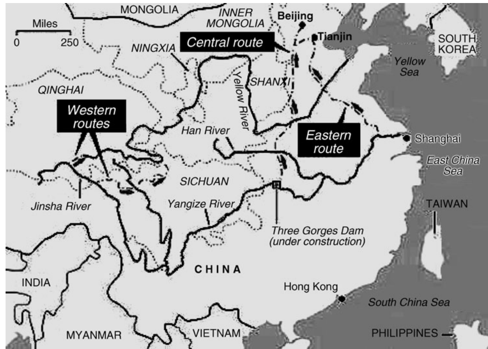
Figure 19.3.10 Three routes of China’s South to North water diversion mega project. The project will divert 44.8 billion cubic meters of water annually from the wetter southern China to the drier north. Planned construction of the project will be completed in 2050 at an estimated cost of $62 billion dollar ( http://www.water-technology.net/projects/south_north/ )
