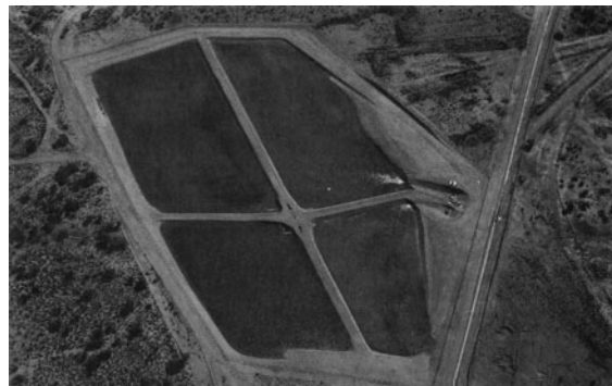
Figure 11.4.7 Avra Valley Recharge Facility near Tucson, Arizona. Recharge facilities consist of five major components: (1) the pipeline that carries the water (or treated effluent) from the source (or wastewater treatment plant); (2) percolation (infiltration) basins where the treated effluent infiltrates into the ground; (3) the soil immediately below the infiltration basins (vadose zone); (4) the aquifer where water is stored for a long duration; and (5) the recovery well where water is pumped from the aquifer for potable or non-potable reuse. (Courtesy of Central Arizona Project, photograph by M. Early.)
