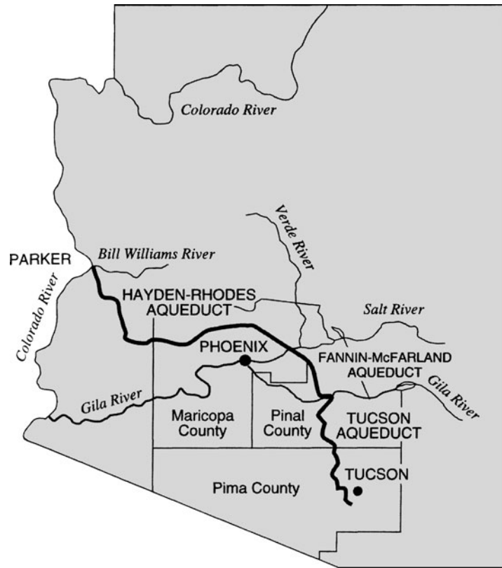
Figure 11.4.3 Central Arizona Project map. Colorado River water is delivered to users by pumping it from Lake Havasu into the conveyance system, then relifting it through a series of pumping plants across the state. From Lake Havasu to the end of the aqueduct, the water is lifted nearly 2,900 feet in elevation by 14 pumping plants. (Courtesy of Central Arizona Project.)
