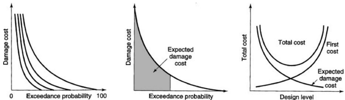
Figure 14.4.3 Computation of expected damage cost and total cost for risk-based design.
