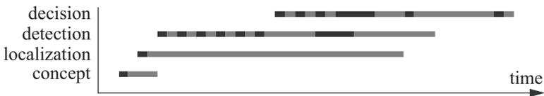
**Figure 10.13.** Distribution of the computation times among the different agents: black indicates the activation of an agent and gray indicates that it is running
