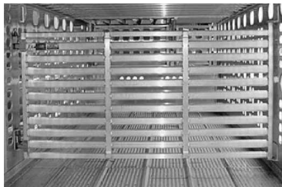
Fig. 10.2 Internal view of livestock trailer showing flooring and metal gate to partition the deck into pens
