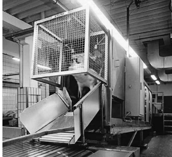
Fig. 10.7 Automatic electrical stunner – Stork MIDAS – shown with pig in stunning box awaiting electrode placement (Source: MPS, Lichtenvoorde, The Netherlands)
