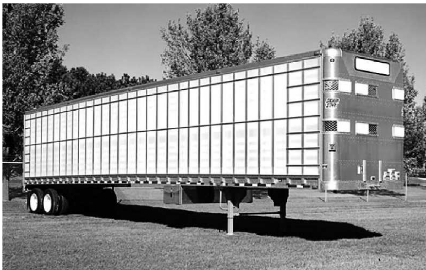
Fig. 10.4 External view of typical North American livestock trailer showing ventilation openings closed off using plastic strips for low temperature travel
