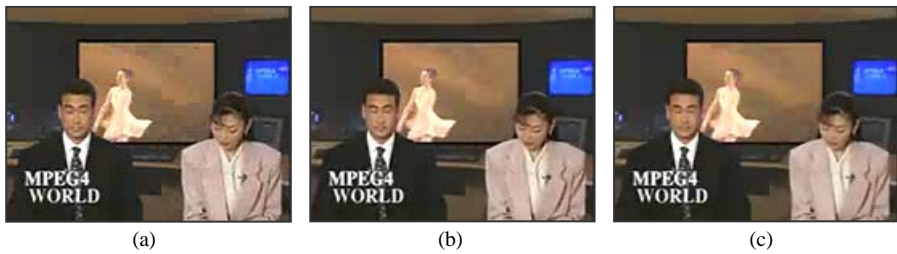
Fig. 2. (a) News 97 th reconstructed frame without loop filter, (b) corresponding reconstructed frame with H.264 loop filter, (c) corresponding reconstructed frame with proposed loop filter
