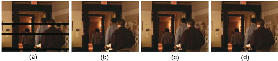
Fig. 6. The reconstructed 144th frame of the P-view S_4 in the “Exit” sequence: (a) error locations - 20.17 dB, (b) SHEC - 26.56 dB, (c) MHEC1 - 28.90 dB, and (d) MHEC2 - 29.37 dB
