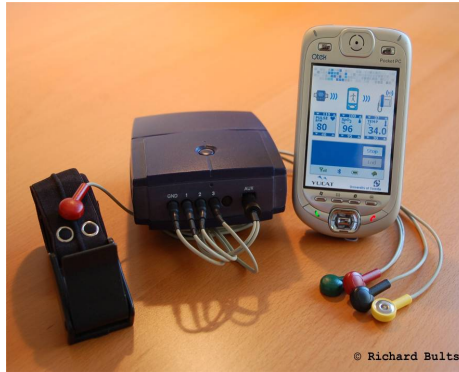
Fig. 2. BAN with electrodes and respiration sensor
