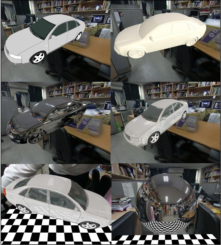
Fig. 6. Rendered images. Colored model (upper-left), diffuse reflection (upper-right), specular reflection (middle-left), combined reflections (middle-right, down).
