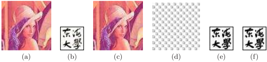
Fig. 3. (a) The original image Lena (b) The watermark (c) The stego-image Lena (PSNR=45.459) (d) The extracted watermark from sub-bands LL and HH (e) The extracted watermark from the sub-band HL (f) The extracted watermark from the sub-band LH
