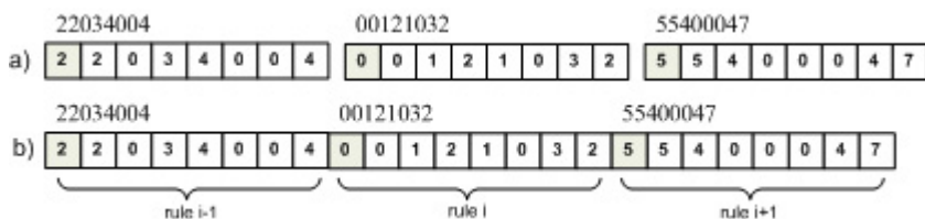
Fig. 5. Coding scheme: a) three rules encoded by natural numbers and b) the fragment of a resulting chromosome
