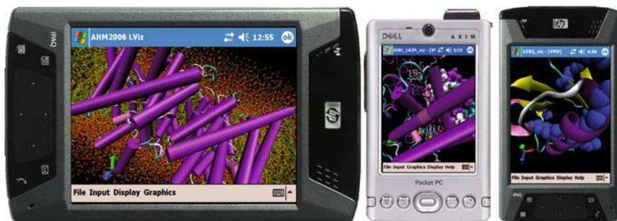
Fig. 6.13 The RealityGrid PDA Client is able to configure itself to provide remote user access and interaction for visualization applications on the grid
