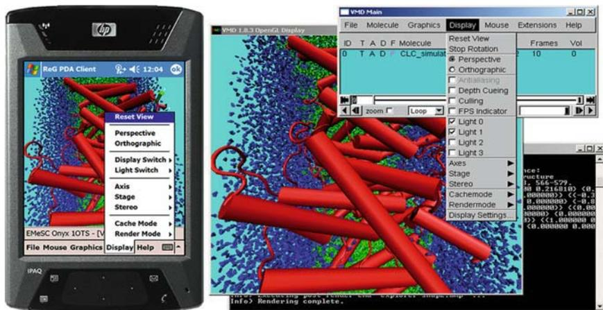
Fig. 6.14 The RealityGrid PDA Client visualization interface has been specifically designed to provide the same user services as the integrated VMD front-end
