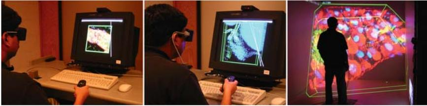
**Fig. 10.10** Experimental setup for the exploring scientific datasets. Scientists examine a range of datasets on a conventional desktop (left), Fishtank (middle), and Cave (right) environment. (Note: different datasets are shown on each display in these images.)
