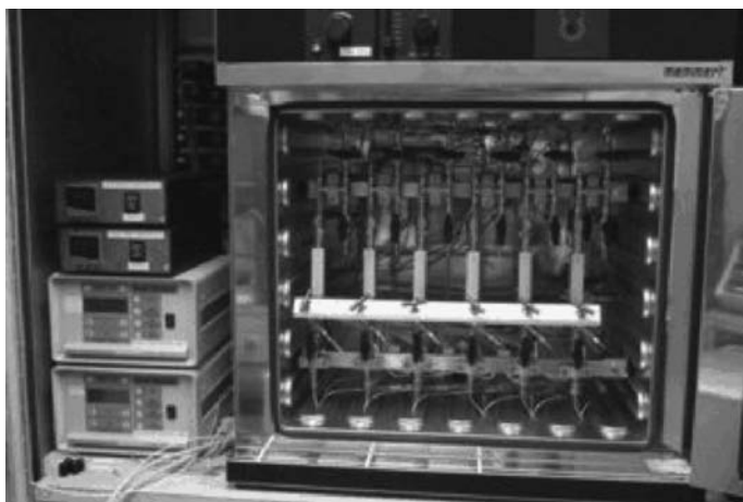
FIGURE A9.5 Fixed beds in laboratory scale, a system of parallel reactors.
