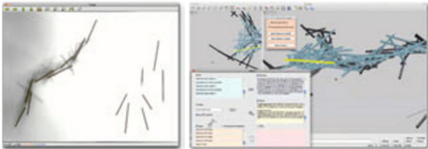
Figure 8 User Interface of the server application and digital model of the stick pile in McNeel Rhinoceros 3D. / Camera tracking: finding the positions of the sticks in the base layer
