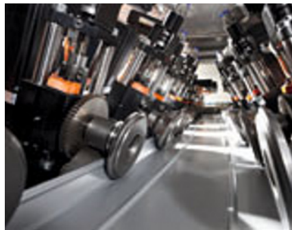
Figure 3 Each MONRO standing seam profile is gradually formed by 24 individually moving stations
