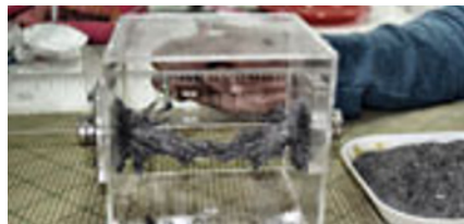
Figure 1 Iron-based material controlled by magnets
