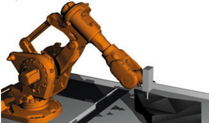
Figure 1 Simulation of robotic fabrication
