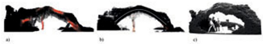
Figure 11 Arch: a) analysis results; b) arch support with parabolic shape; c) resulting structure
