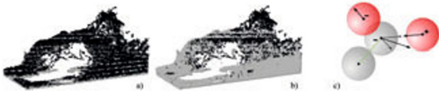
Figure 6 Self-organization method: a) first layers of the structure; b) vanished, omitted particles in the structure; c) magnetic principles in the algorithm
