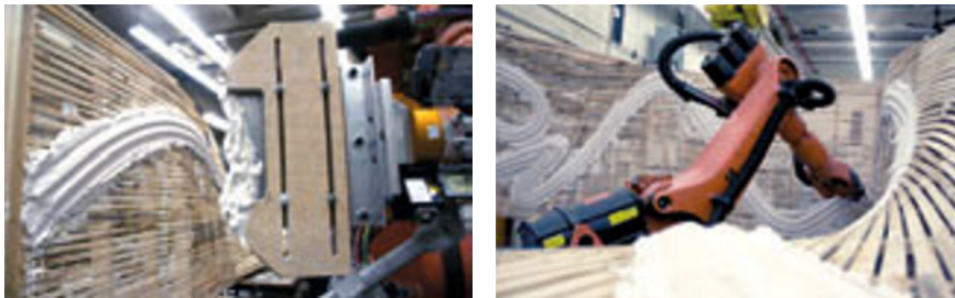
Figure 1 Left: custom robotic profiling tool; right: plaster robotically applied in lab
