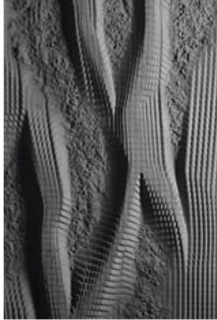
Figure 1 Robotically fabricated concrete element, casted at full scale in concrete (Procedural Landscapes, Gramazio & Kohler, ETH Zurich, 2011, in cooperation with Prof. Girot, ILA, ETH Zurich und Yael Girot, Atelier Girot).
