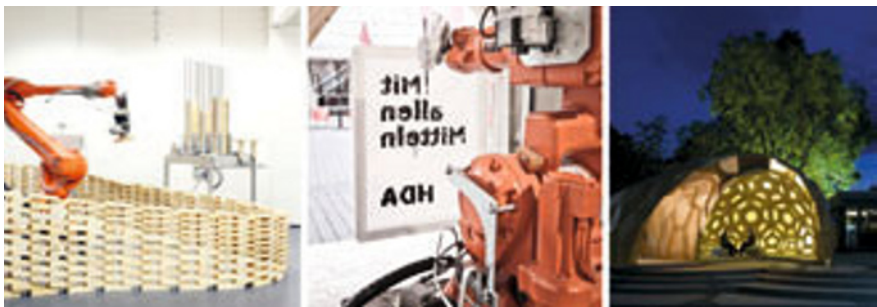
Figure 1 Gramazio/Kohler’s brick-laying robot in action (left); Dank’s Chinese ink painting robot (center); Menges/Knippers’ ICD/ITKE research pavilion 2011 (right)
