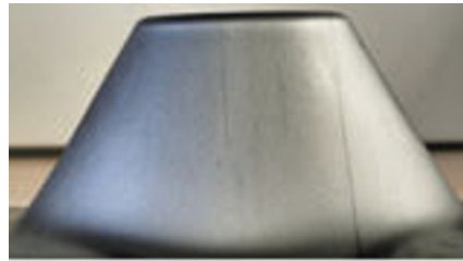
Figure 4 Cone frustum, infeed 1 mm: initial sheet (left), inner surface (middle), outer surface (right)
