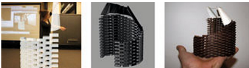
Figure 5 From left: a) simultaneous gestural generation of brick wall and loft surface using hand coordinates; b) geometry exported to Rhino 3d; c) lasercut scale model
