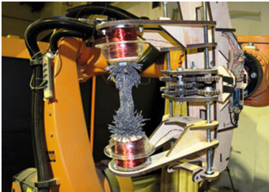
Figure 5 Final end-effector mounted on the industrial robot
