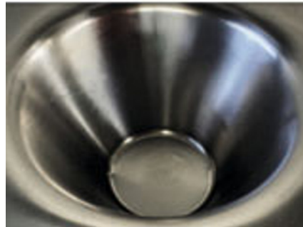
Figure 5 Cone frustum, infeed 0.5 mm, using dummy sheet: produced part (top), formed dummy sheet (bottom)
