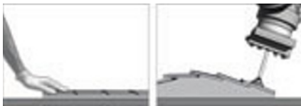
Figure 4 Human versus robotic tiling capability
