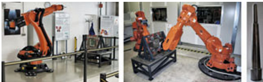
Figure 3 Forming set up used at IRPA: SPIF (left), DPIF-P (center), forming tool (right)
