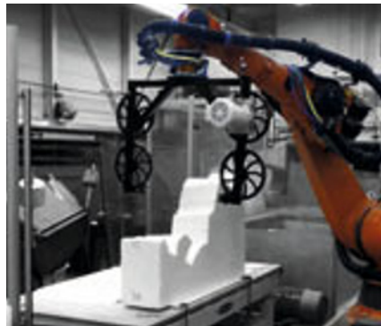
Figure 10 6 axis CNC diamond wire saw (left); Wire sawing end effector developed at the University of Michigan Taubman College (right)
