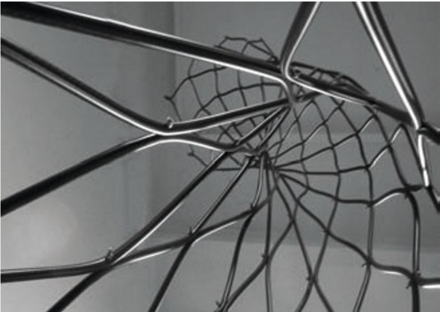
Figure 2 superTEX tower: Vertical shaped net structure made with splineTEX carbon.
