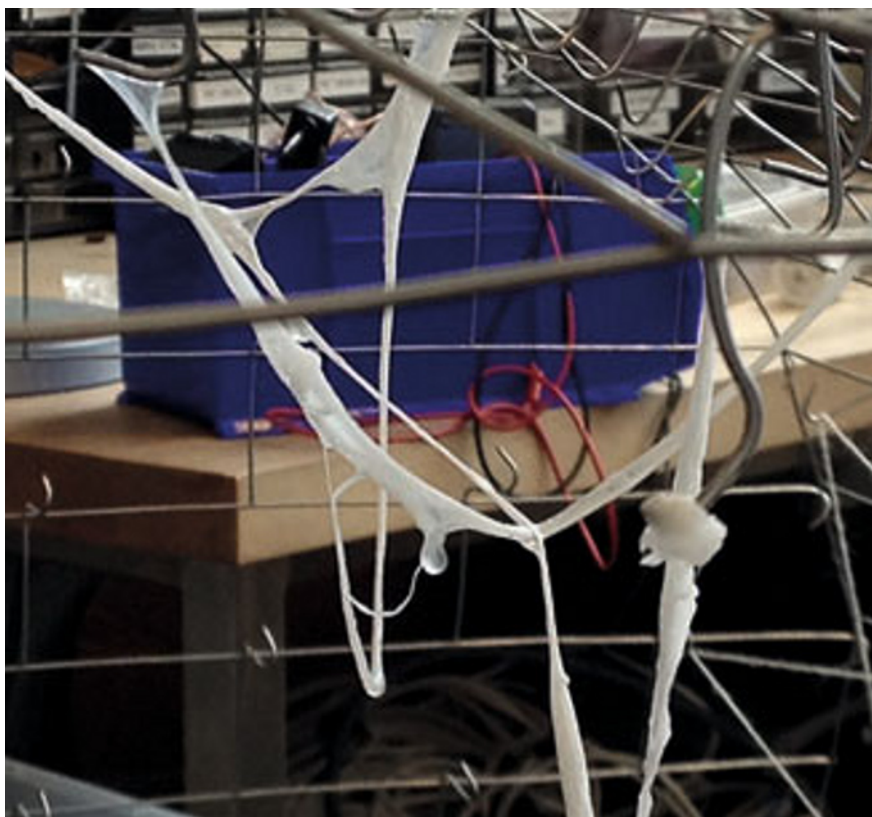
Figure 4 Nylon threads attached to hooks on a steel frame formed by dipping the hooks into a nylon prepolymer solution
