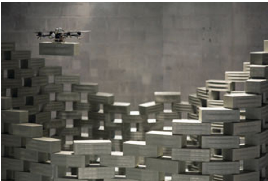
Figure 8 A quadcopter placing a polystyrene module (Flight Assembled Architecture, Gramazio & Kohler and Raffaello D'Andrea in collaboration with ETH Zurich, 2011, image by François Lauginie)
