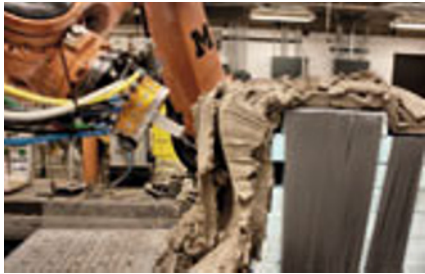
Figure 8 Clay either falls or is forced away on the next cut path
