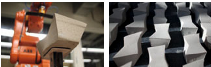
Figure 4 Prototypes produced during flowing matter research using a custom end effector (students: Stefano Andreani, Jose Luis Garcia del Castillo y Lopez, and Aurgho Jyoti)
