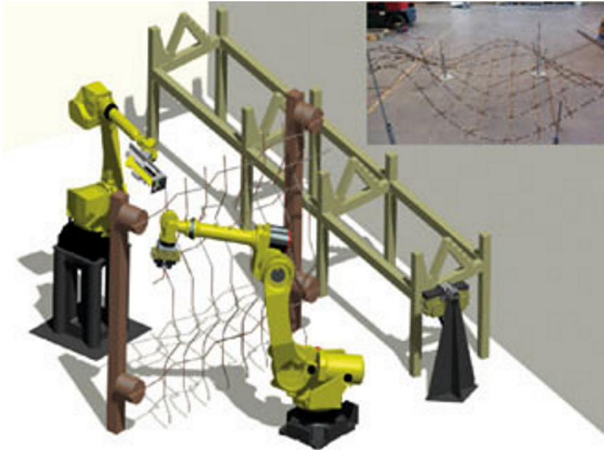
Figure 4 Two robot reinforcement fabrication unit. The robot to the right is #1 and the floor mounted gripper is the bending tool. The robot to the left is #2 and handles the binding of the rebar grid. In the upper right corner a manually produced 3D reinforcement grid is shown.
