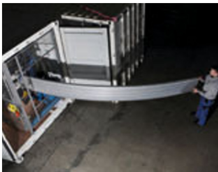
Figure 2 The 3D-bending machine is built into a 20-foot intermodal container
