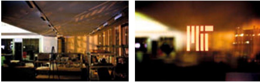
Figure 8 An environment (left) and the resulting inverse light painting from the same scene (right) shows the effects of a large synthetic aperture. Note that occlusions smaller than the synthetic aperture, like the windows on the right of the scene, can be imaged through if the focal plane is tuned past the occlusions.
