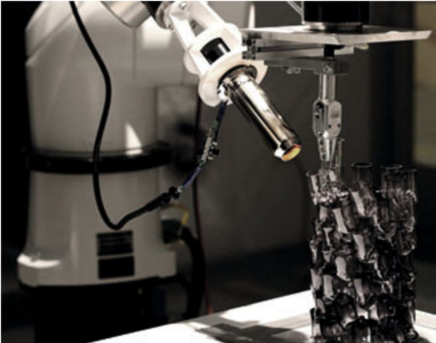
Figure 6 Hot Networks Experiment 1, showing robot collaboration to fuse PETG plastic components using heat and applied pressure
