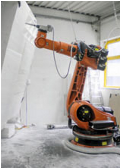
Figure 2 Robot milling foam mold
