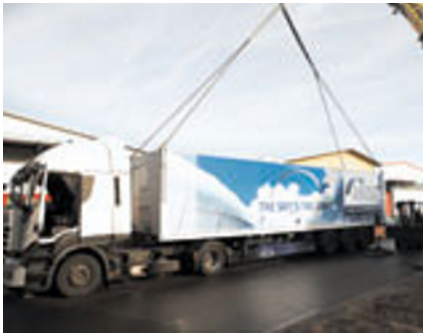
Figure 1 A customized 40-foot intermodal container enables deployment of the 3D-roll forming machine
