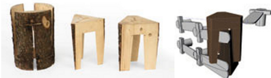
Figure 7 The log after machining: waste, first stool, second stool, toolpath-planing 2 of 14 cuts
