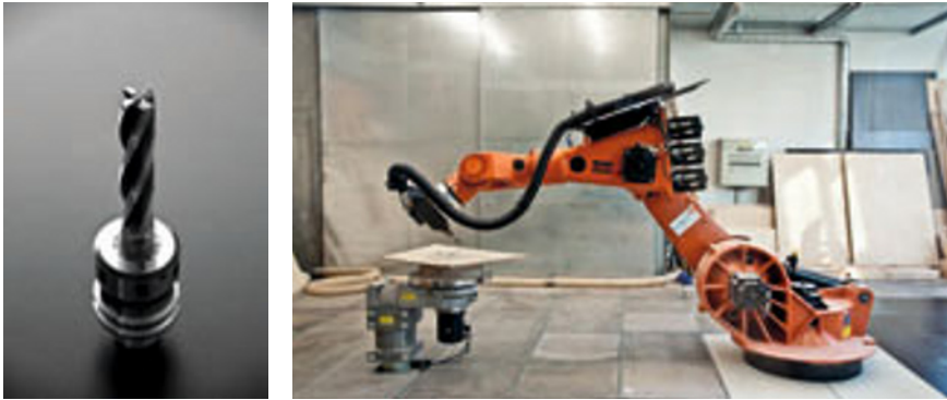
Figure 4 Customized milling cutter for shaft and end milling utilized in the developed robotic fabrication process (left); machine setup: 6-axis robot connected with a separate turntable as an external axis (right)
