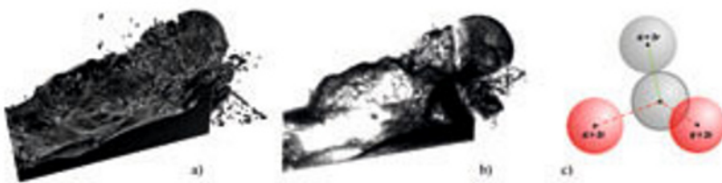
Figure 2 Fluid simulation: a) surface area based on mesh geometry; b) volume of the wave, represented by particles; c) particle position dilemma
