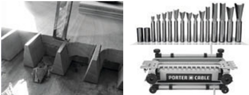
Figure 2 Manual fabrication of dovetail joints (Baumgartner, left); Tools for machine-based fabrication of different finger joints restricted to a 90° connection (Super Carbide Tools and Porter Cable, right)
