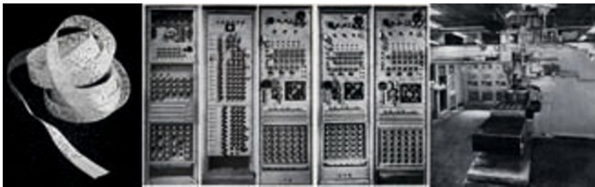
Figure 1 Pre-punched program tape, control panels and general view of the MIT's Cincinnati Hydrotel 3-axis milling machine, early working prototype of NC (Numerical Control) technology (Pease, 1952)
