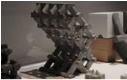
Figure 4 Structural UHPC mesh sample from EZCT's u-Cube construction system
