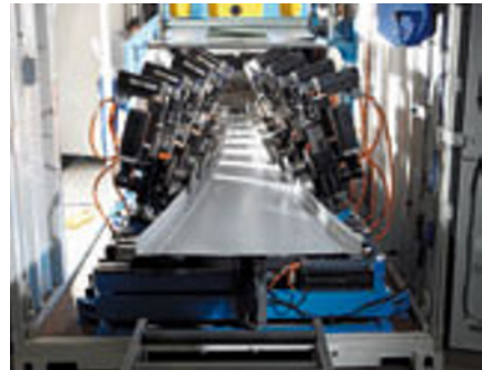
Figure 1 A customized 40-foot intermodal container enables deployment of the 3D-roll forming machine
