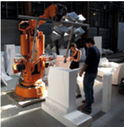
Figure 3 Production of the RDM Vault at Hyperbody’s robotics workshop in Rotterdam
