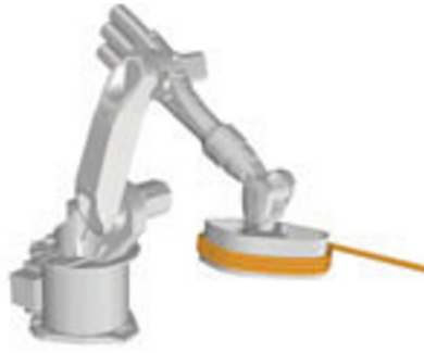
Figure 4 Robotic winding process fully simulated in a CAD environment
