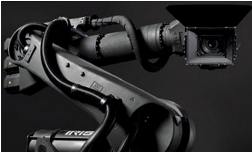
Figure 1 Bot&Dolly's IRIS Motion Control System
