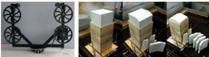
Figure 3 Left: custom robotic wire saw; right: successive cuts from plaster block
