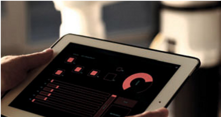
Figure 5 Custom ipad interface for charla designed in Touch OSC that allows the user to configure and control the robotic network from one device. The interface also has a feedback component, which allows the user to visualize each robot’s status in their program in real-time.
