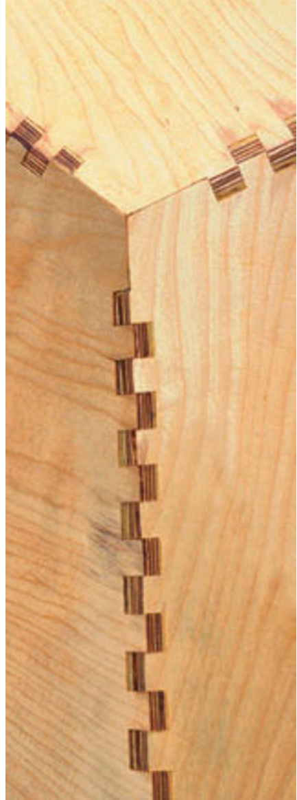
Figure 4a The robotic fabrication of finger joints allows the connection of plywood plates at variable angles without the need for any additional mechanical elements.
