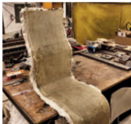
Figure 10 Minimal fiberglass wasted near edge
