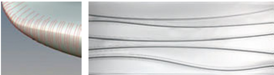
Figure 4 Principle Curvature Lines indicate directions for families of geodesics that form the centerlines and/or the edges of strips which represent almost straight developable surfaces with low torsion (left). Sample surface displaying metal standing seam panels with independently curved edges (right).
