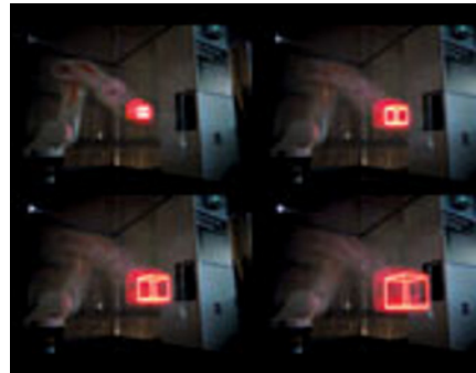
Figure 5 A series of 3D light structures are fabricated and captured as long-exposure photographs, as frames of an animation sequence of a growing cube.
