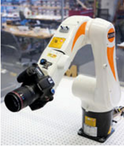
Figure 6 The setup used for inverse light painting has a robotically controlled camera and a fixed environmental light source.
