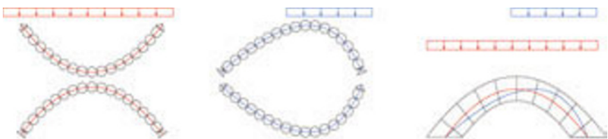
Figure 5 Functional curve: uniformly distributed load (left); nonuniformly distributed load (middle); inside an arch (right)
