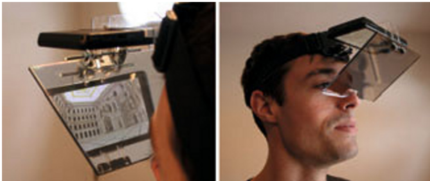
Figure 2 Smartphone based augmented reality headset; Equirectangular image credit: Ilja van de Pavert
