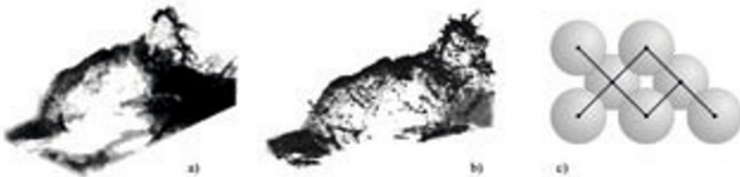
Figure 10 Analytical model: a) result of "virus" algorithm; b) top nodes with applied snow load; c) spheres transformed into beam finite elements
