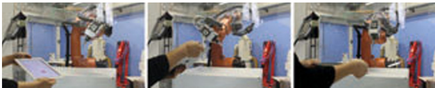
Figure 4 Communication between an iPad and the KUKA robot via the server-application: simultaneous movement of the end effector of the robot to the orientation of the iPad
