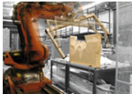
Figure 6 Slab cutting EPS
