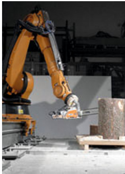
Figure 1 Robotic log-cutting using a chainsaw, programmed in Rhino2krl
