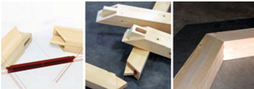
Figure 6 Comparison of digital parametric model (left); milled joint parts (center); assembled joint (right).
