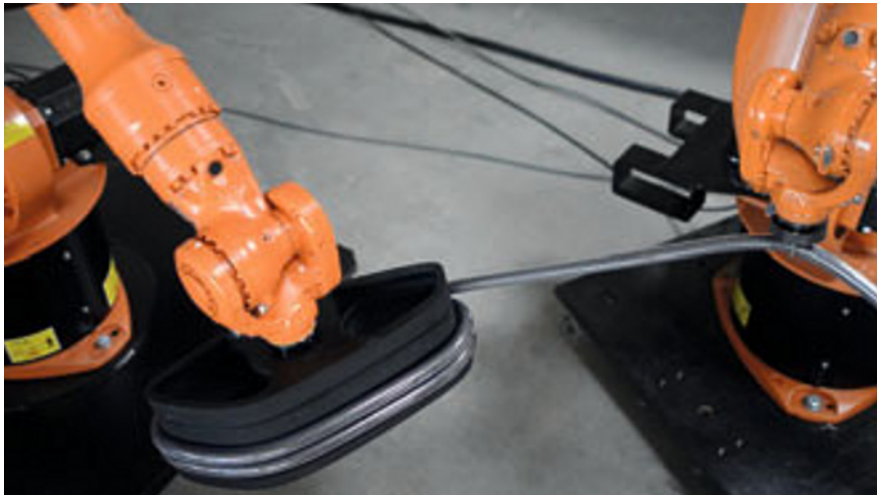
Figure 5 KUKA robots forming a 1:5 scale chassis part, parametrically programmed in KUKA|prc
