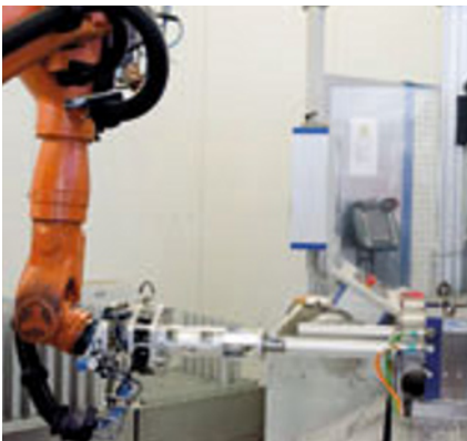
Figure 1 Robot inserting tube into CNC machine
