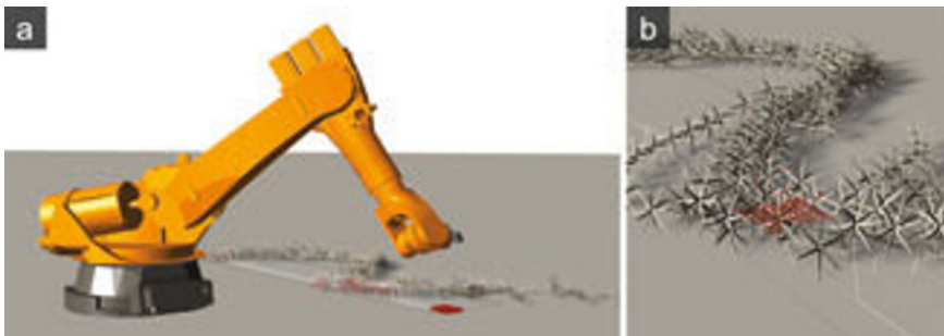
Figure 4 Simulation of the tool-path using the online motion-planning strategy established. As a basis of this simulation a rigid-body dynamics generated model of the designed granulates is being used: a) real-time simulation of the robotic kinematics, b) detail of the robotic motion paths.
