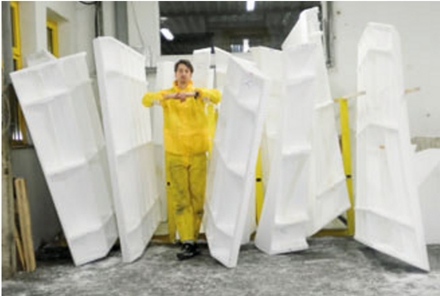
Figure 3 Foam molds, ready for aluminium casting
