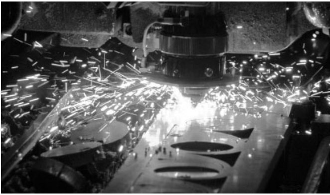
Milgo's laser-cutter, one of the several digital-fabrication devices used for different Milgo experiments.
