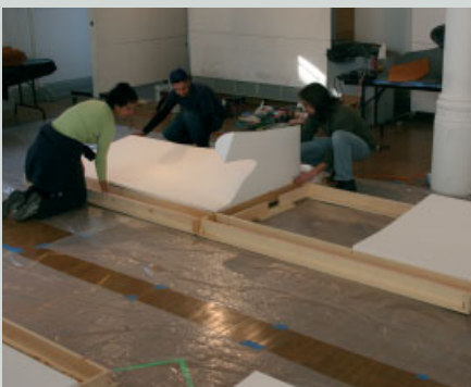
Chandelier fabrication process using epoxy resin, carbon-fibre and Nomex drapes over a CNC foam-cut mandrel.
