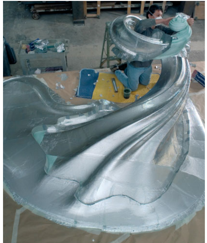
View of single Helioscope under construction. The fabricator applies metal foil as a seal to the foam surface in anticipation of a 15-piece urethane mould. The final cast of the helical tail will produce a super-lightweight fibreglass shell.
