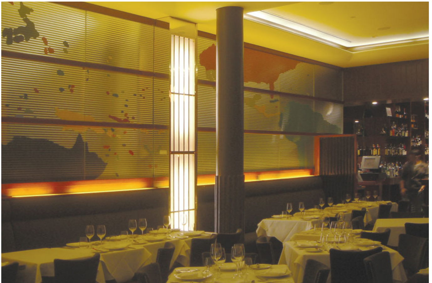
David Higginbotham's glowing mural on the south wall depicts a map of the world to reinforce the international theme. The various countries are painted in greens, reds, ochres and dark blues etched in paint on the back of a mirror and then covered with clear corrugated glass. Glowing pilasters between each section supplement light from recessed coves and ceiling fixtures.
