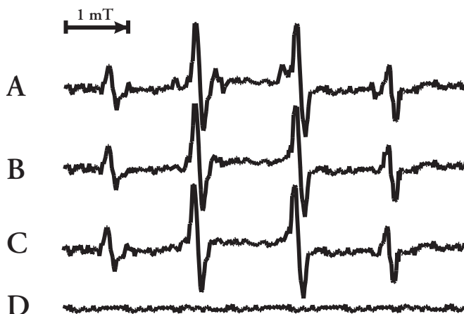
FIGURE 11.11 ESR spectra of the DMPO/OH adduct formed by trapping of HO • radicals from respiring mitochondria; no addition (A), + SOD (B), + catalase (C), myxothiazol (D). Mitochondria were uncoupled by freezing and subsequent thawing. Mitochondrial protein (1.5 mg) was suspended in 300 \mu l reaction medium [0.15 M KCl – 0.5 mM KH 2 PO 4 -buffer (pH 7.4)] in the presence of 6 mM succinate, 1 \mu g antimycin A and 0.3 M DMPO.
