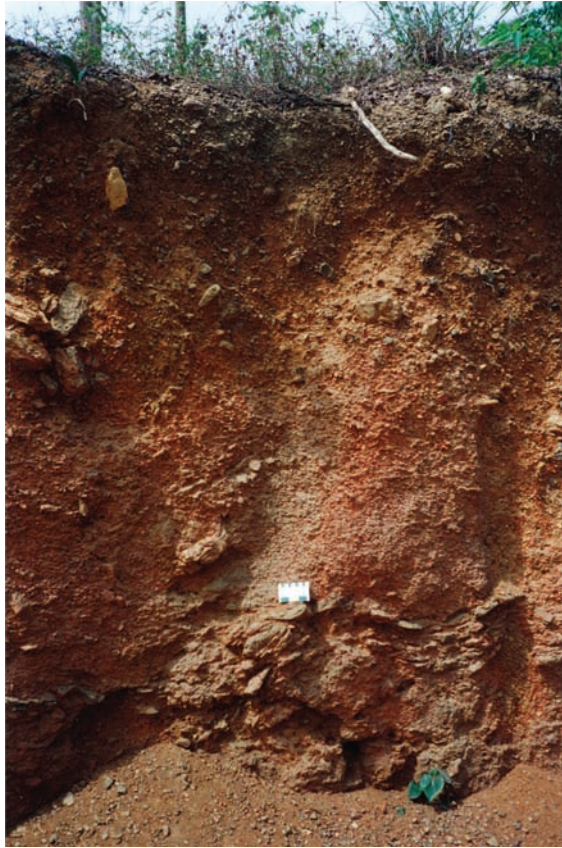
C.7 Lateritic gravel formed in a profile of residual weathered shale.
