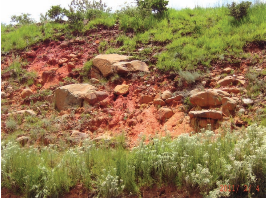
C.3 Residual profile of a diabase dyke.
