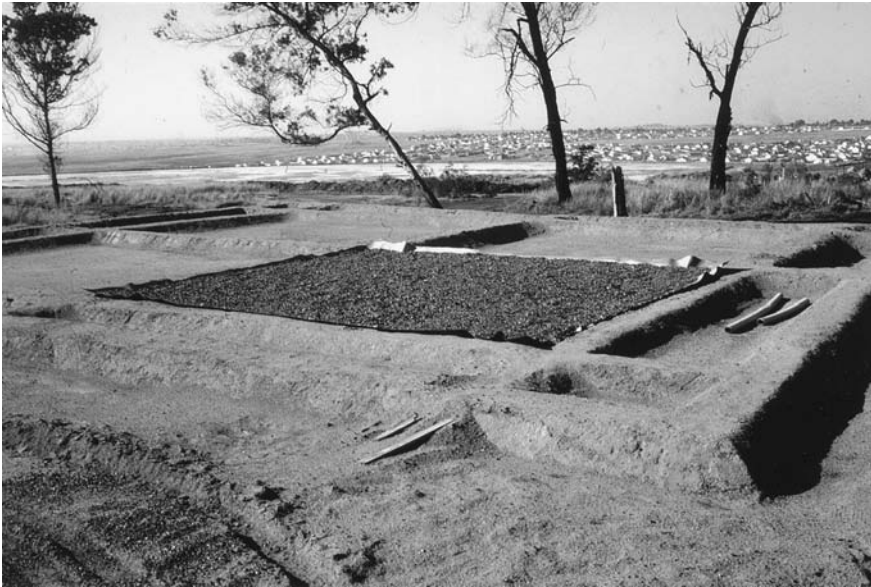
Plate 5.1 Set of four moated seepage test ponds with lined pond (for assessing evaporation) closest to camera.
