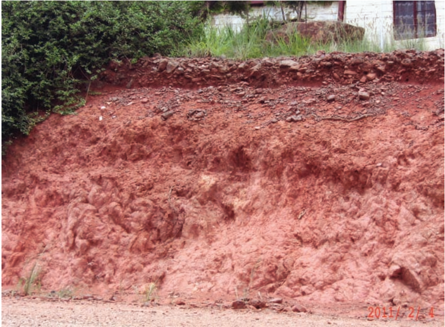
C.11 Relatively shallow weathering of a mudstone profile.
