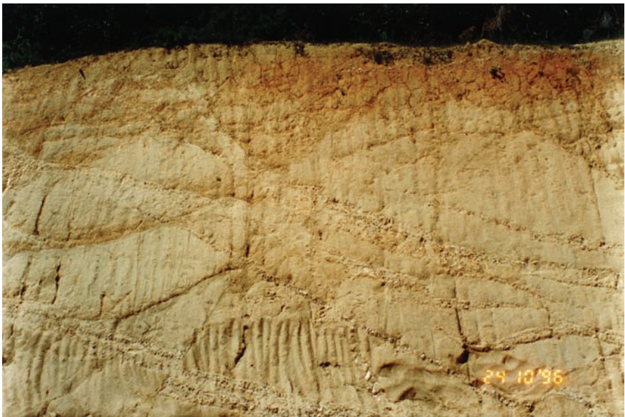
C.6 Profile of residual volcanic ash showing saprolitic features.
