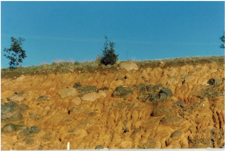
C.4 Residual weathered andesite lava flow containing quartzite floaters.
