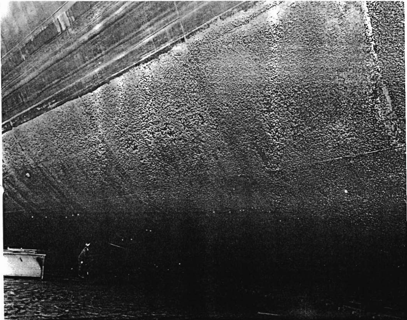
Fig. 2 Underwater hull showing heavy fouling
