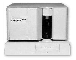
Fig. 18.8 The Luminex 100<sup>TM</sup> system (Copyright (2000) of the Luminex Corporation TX, USA; all rights reserved); the unit below the cytometer is for the storage and automatic loading of 96-well plates. (Reprinted with permission of the copyright holder, the Luminex Corporation.)
