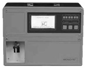
Fig. 18.4 The Microcyte portable cytometer. The cytometer, which weighs just 12 kg and measures 330 mm  $\times$  430 mm  $\times$  160 mm, can be powered by rechargeable batteries or an external 12 V d.c. source. (Reprinted with permission of the copyright holder, Optoflow AS.)
