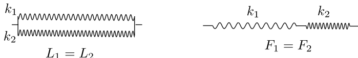
Figure 32. What is the effective Hooke's constant for springs in series and in parallel?
