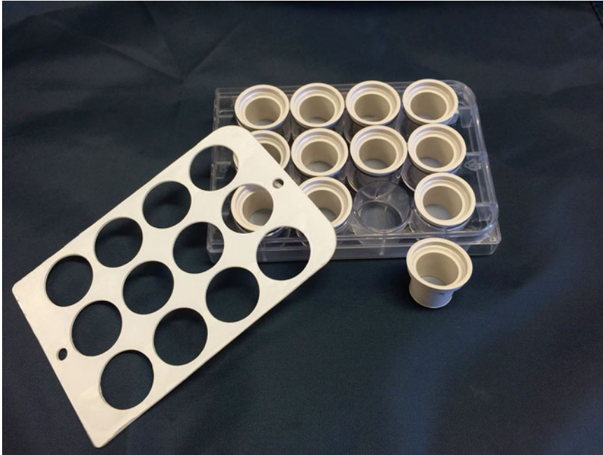
Fig. 1 Net wells used to incubate samples
