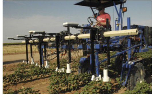
Fig. 30.8 High clearance tractor with sets of sensors that allow simultaneous measurement of canopy height, temperature, and spectral reflectance of cotton crop (Source: White et al. 2012)
