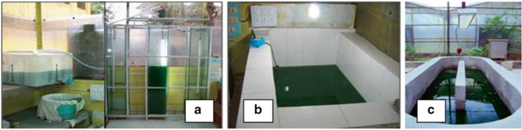
Fig. 2.8 Algal cultivation in (a) photobioreactor, (b) open tank, and (c) open raceway pond
